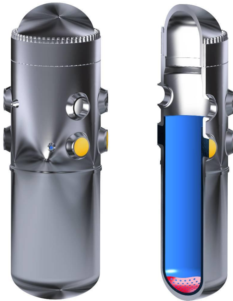
Fig. 2: WWER-1000 CFD model
