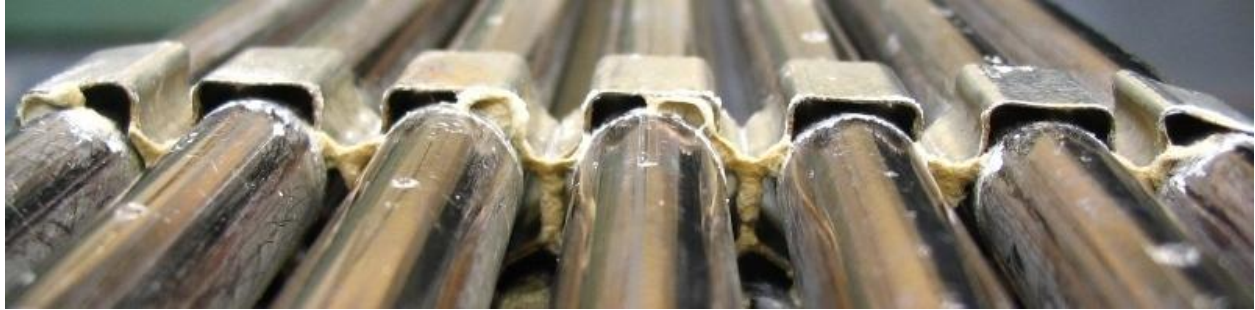
Figure 4 Mineral wool fibers attached at the spacer grid of the VVER-440 FA model in the experiment carried out with a full-scale sump strainer model.
