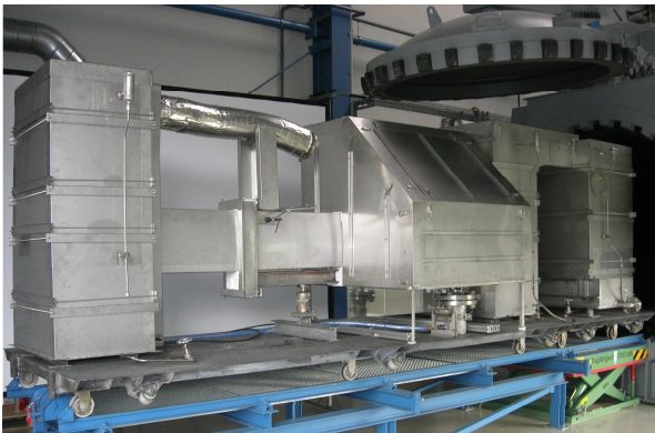
Fig. 2: TOPFLOW Hot leg model in front of the pressure chamber
