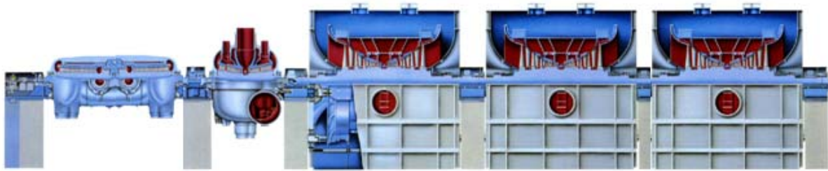
Fig. 2: Turbine design concept with double flow HP, IP and 3 LP turbines [11]
