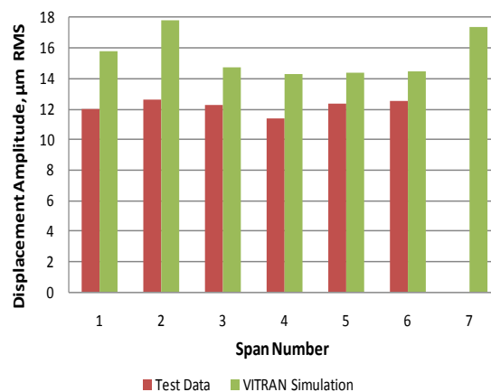
Figure 14: Fuel rod displacement vibration amplitude: Test data vs. CFD/VITRAN simulation
