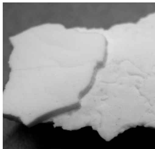
Figure 4 crust with easily separated layer at the wall in L5L test test
