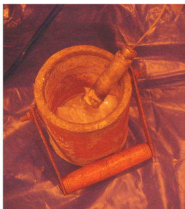
Figure 5 Lifted Al-can with some white materials sticking to its bottom.
