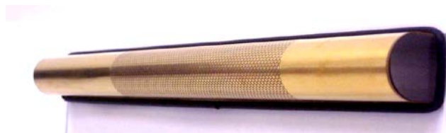
Figure 17 Bended film sensor on top of a semi-cylindrical fuel rod model
