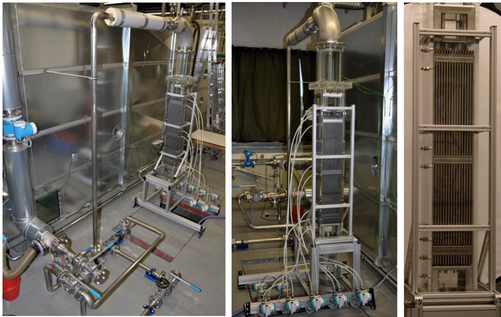
Figure 4: FA-dummy test-section with head loss-instrumentation.
