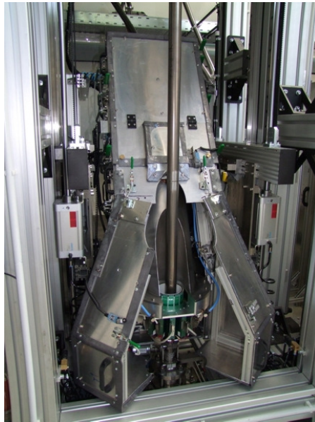
Figure 6: left side: scheme of the titanium test section with tomography scanner and gas injection; middle: scanner in elevator system; right side: multi-hole gas injection device
