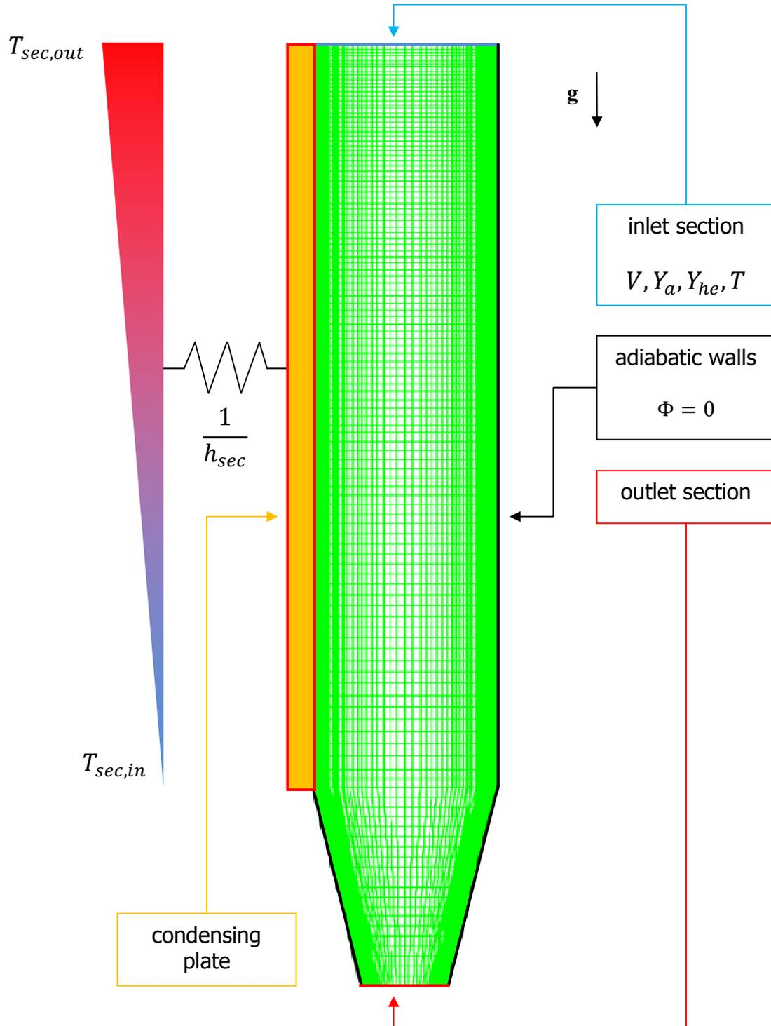
Figure 9 Computational discretization and boundary conditions
