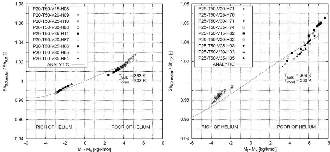
**Figure 7 Ratio of the Sherwood numbers calculated according to Bird et al. [32] and Lienhard [30] models.**
