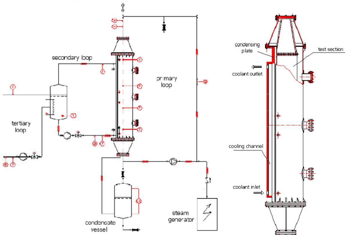
Figure 1 Layout (left) and test section (right) of the CONAN facility.
