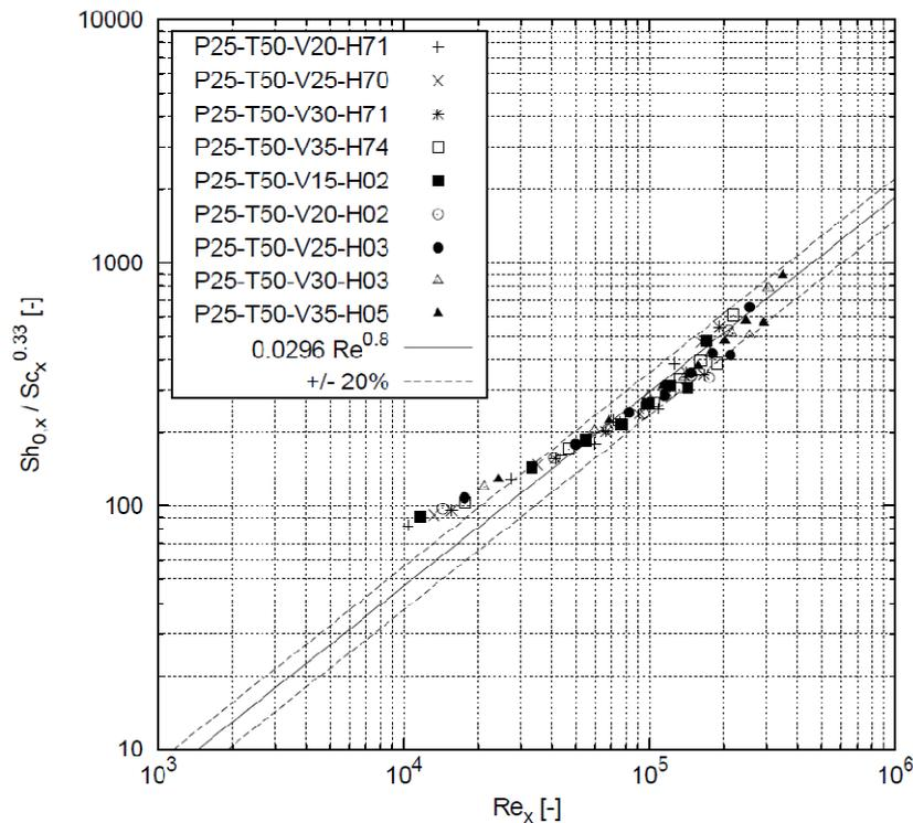
**Figure 4 Experimental Sherwood number in forced convection tests at 25 kW**
