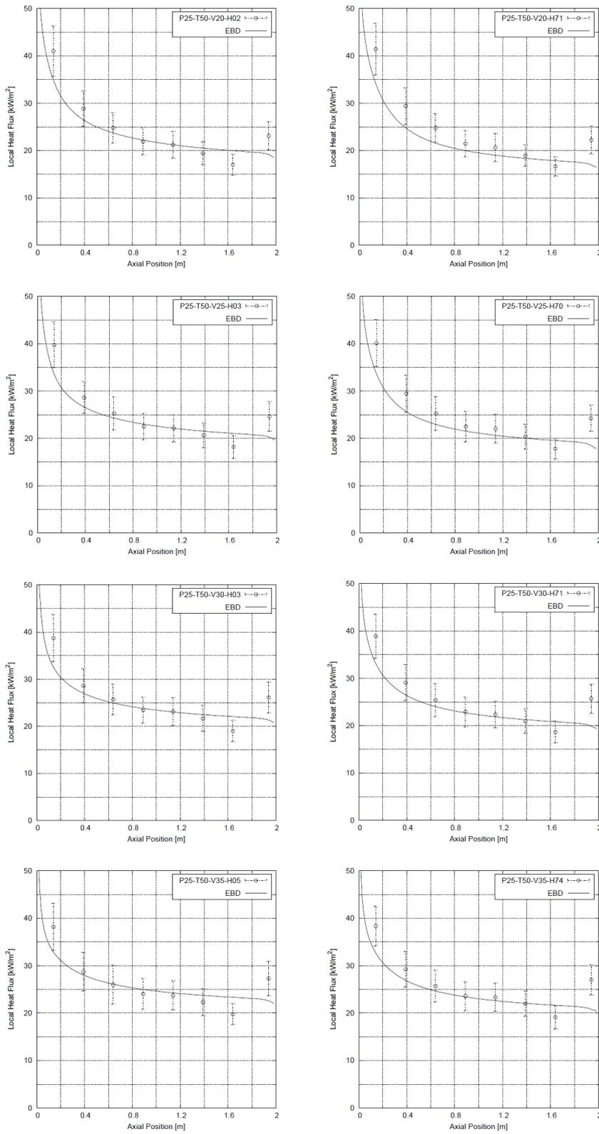
Figure 12 Comparison between calculated and experimental heat fluxes in tests at 25 kW.
