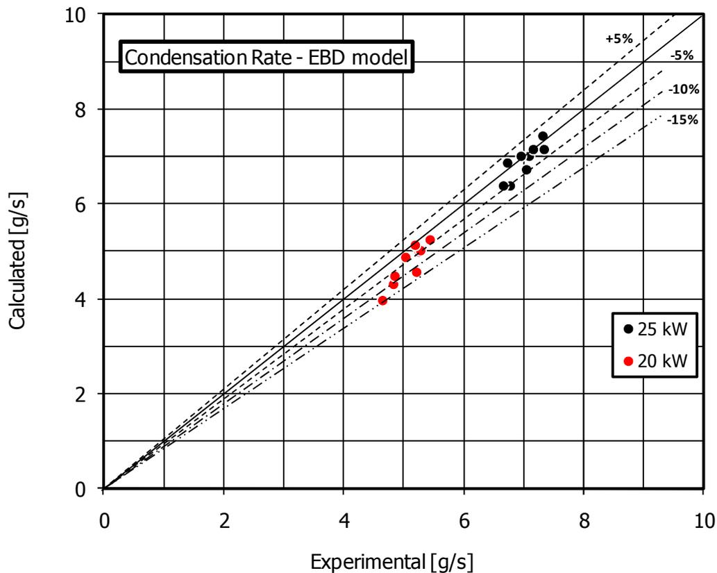
**Figure 10 Comparison between calculated and experimental condensation rates.**
