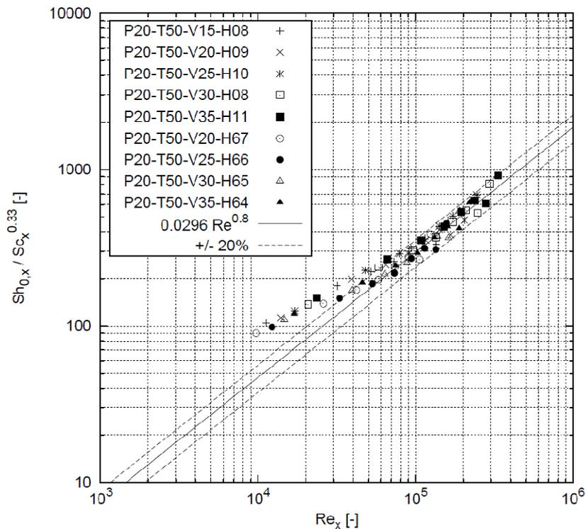
Figure 3 Experimental Sherwood number in forced convection tests at 20 kW
