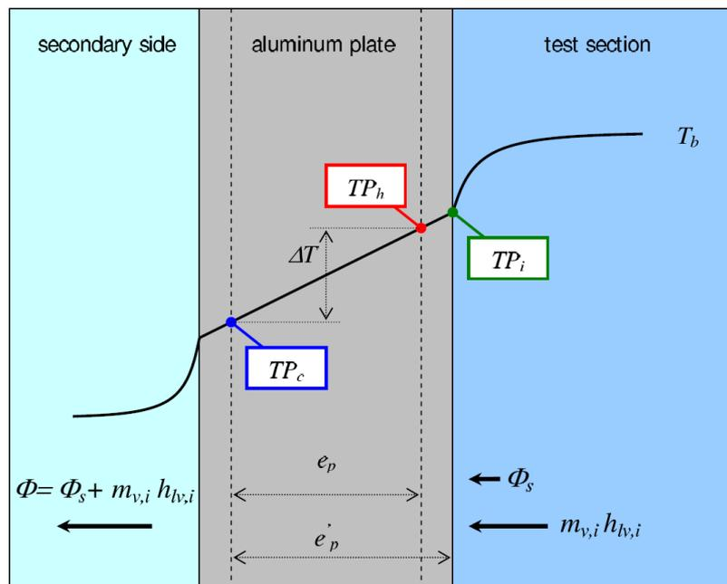
**Figure 2 Sketch of temperature profile within the condensing plate**
