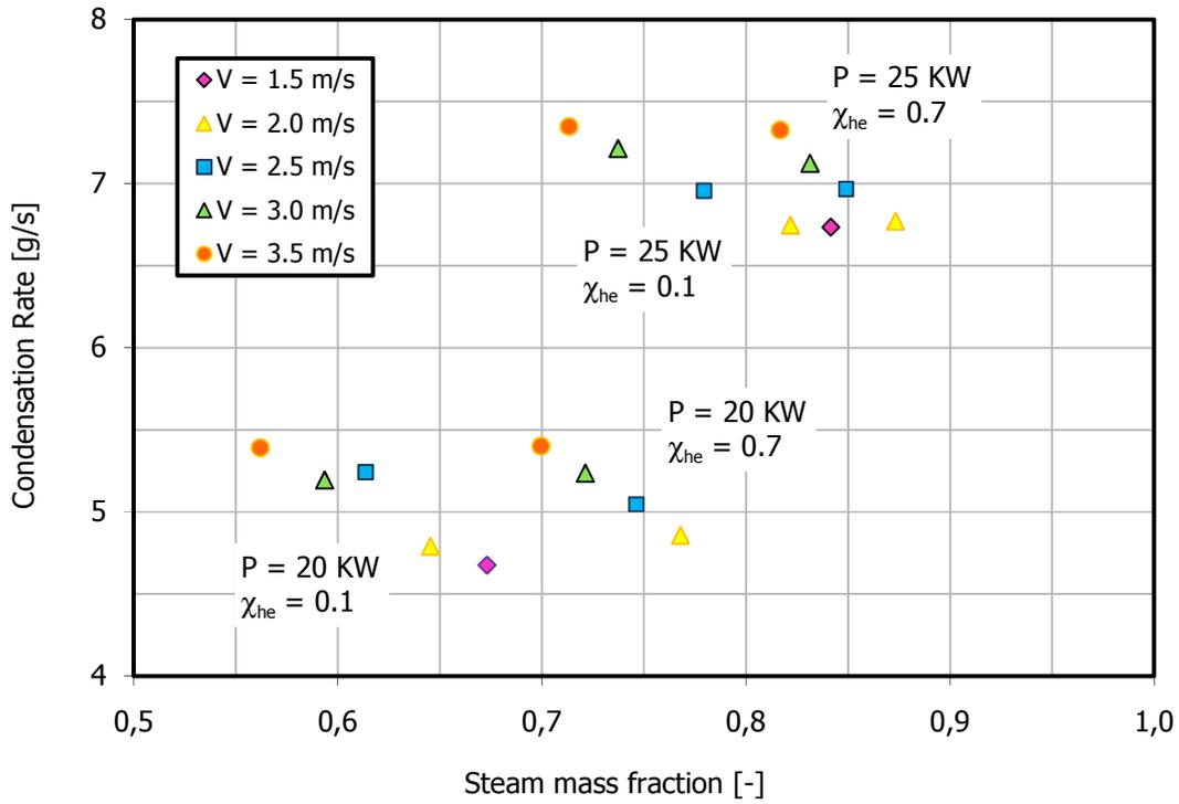
Figure 5 Overall condensation rates vs. steam mass fractions
