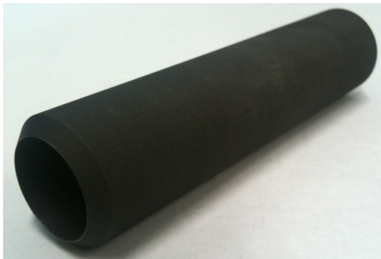
Figure 12: Image of the final heater element shape, composed of Tokai A348 Isostatic Graphite.
