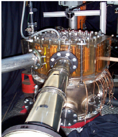
Figure 2 Banquise experiment (1/5 th scale of a PWR 4 loops)
