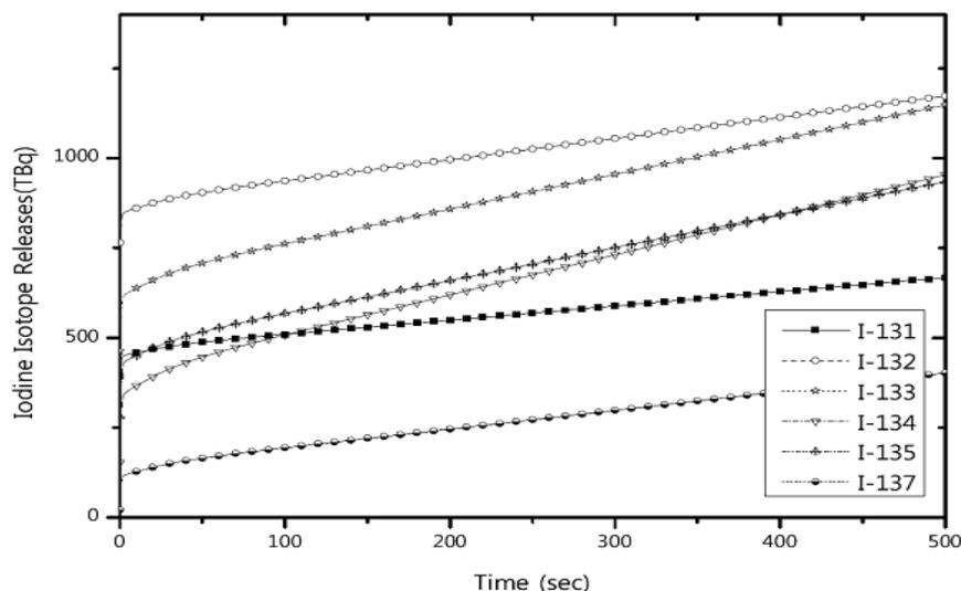
Figure 3 Iodine transient releases following end fitting failure (prompt release + transient release from grain boundary and in-grain inventories)
