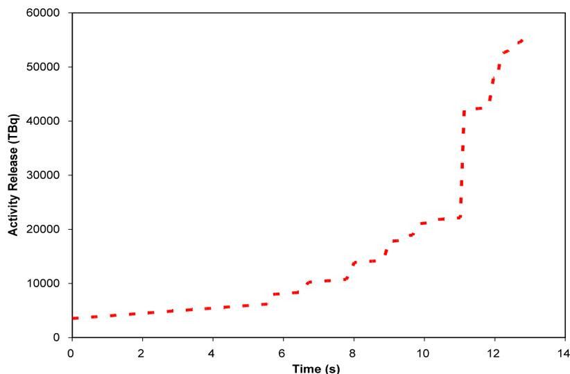
Figure 2 Transient releases for Iodine, Krypton and Xenon following feeder stagnation break
