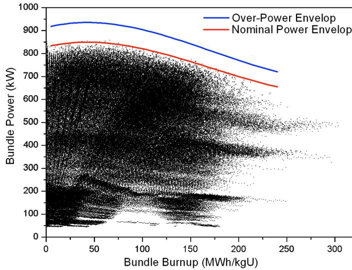
Figure 2 Nominal and overpower envelopes for refurbished Wolsong-1 NPP
