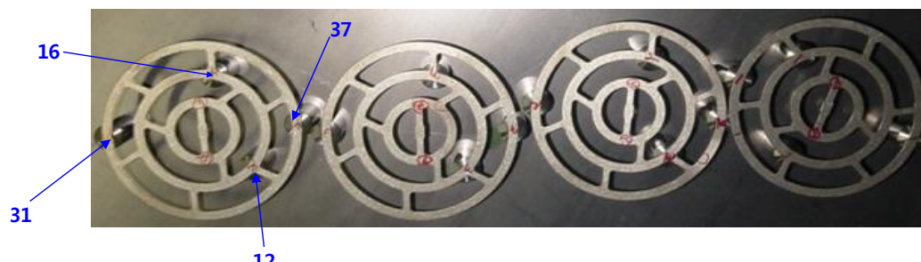
Figure 10 Photograph of the weld specimens for PM torque test.
