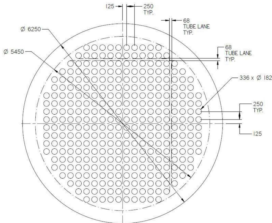
**Figure 5 Cross-Section Layout of Fuel Channels in the Canadian SCWR Core.**
