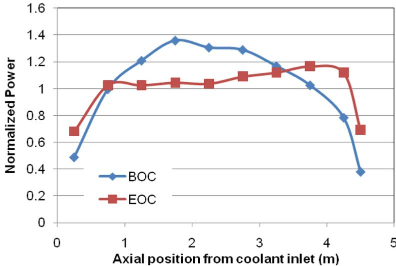
Figure 8 Axial power profile of maximum power channel.
