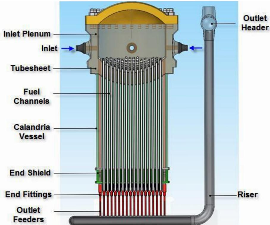
Figure 4 Cross Sectional View of the Pre-Conceptual Canadian SCWR Design.
