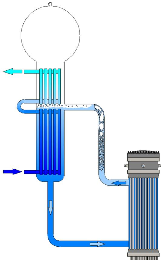
**Figure 10 Schematic Diagram of the Passive Moderator Cooling System.**
