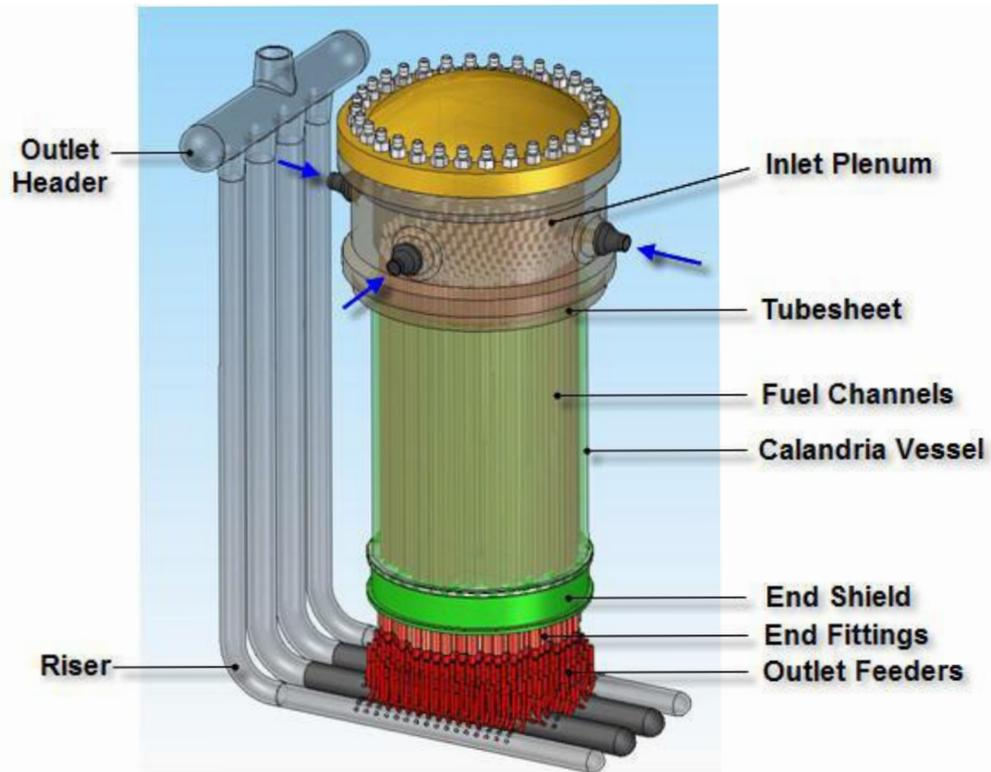
Figure 3 Schematic Diagram of the Pre-Conceptual Canadian SCWR Core Design.
