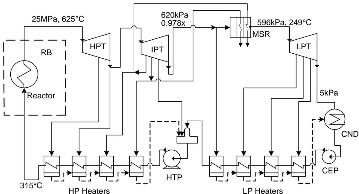
**Figure 1 Schematic of Direct Cycle with an MSR in an SCWR Plant.**
