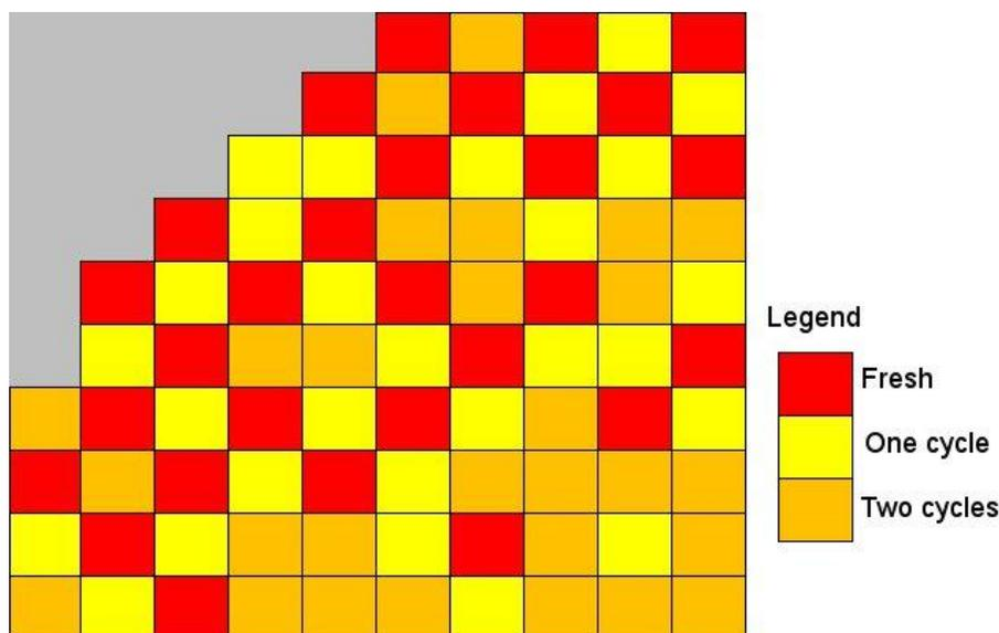
**Figure 7 Quarter core fuel loading pattern.**
