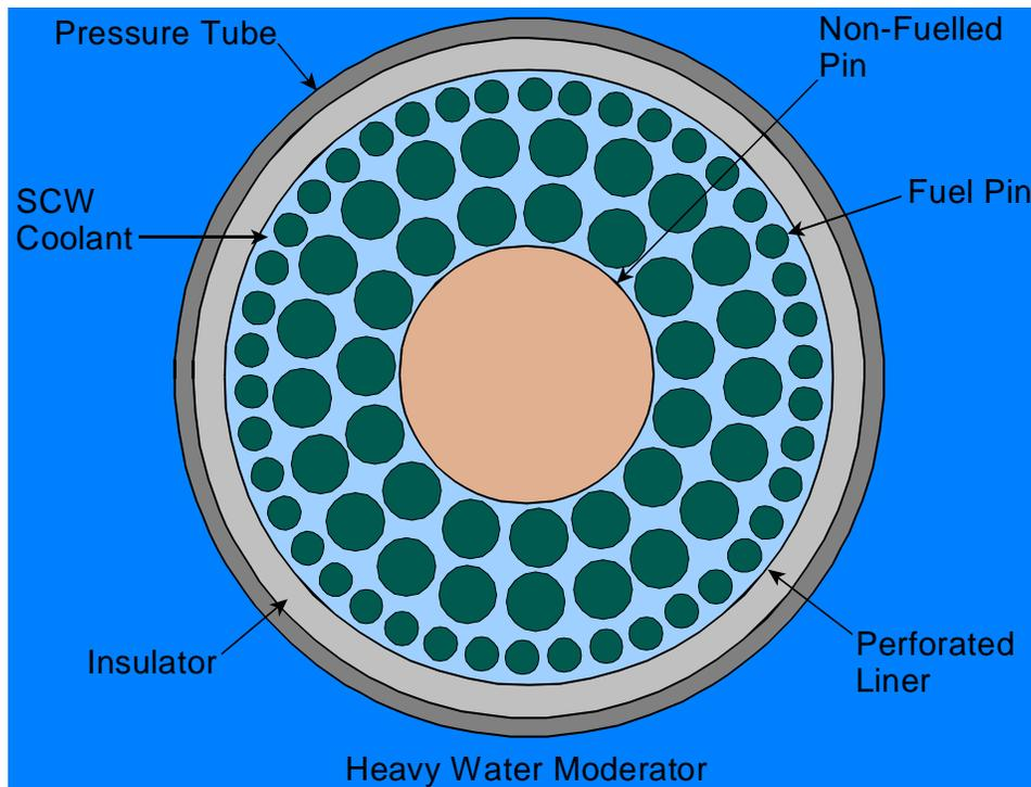
**Figure 6 Schematic Diagram of the High Efficiency Channel.**
