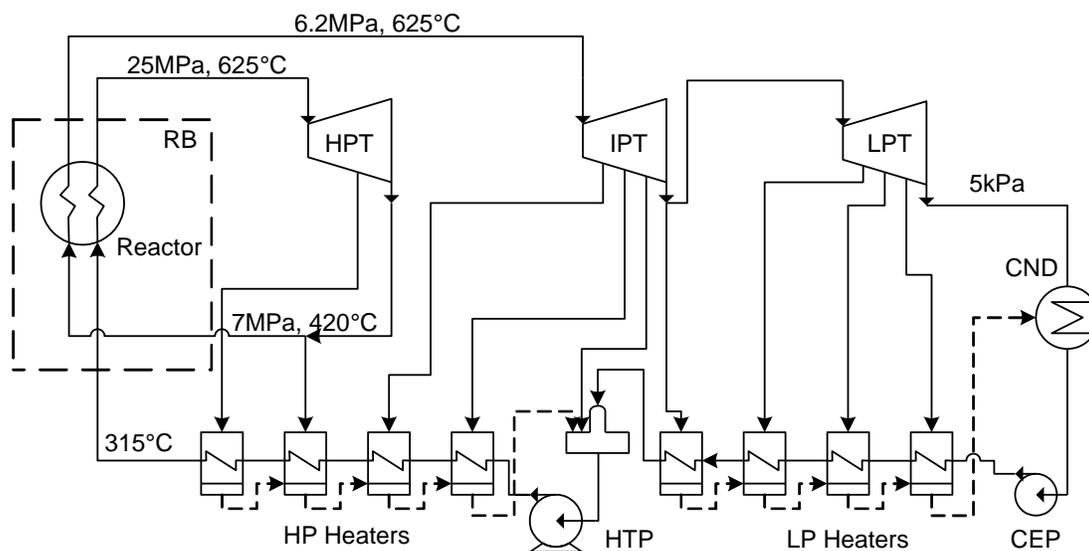
**Figure 2 Schematic of Direct Cycle with Reheat in an SCWR Plant.**
