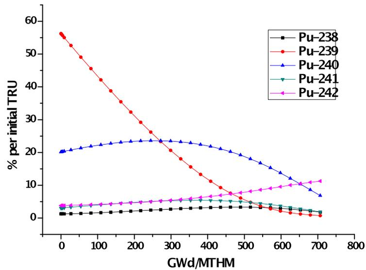
Figure 4. Plutonium composition vs. burnup for regular kernel size with PF=40%.
