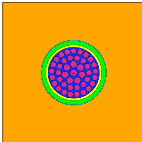
Figure 1. Schematic configuration of the CANFLEX fuel bundle.
