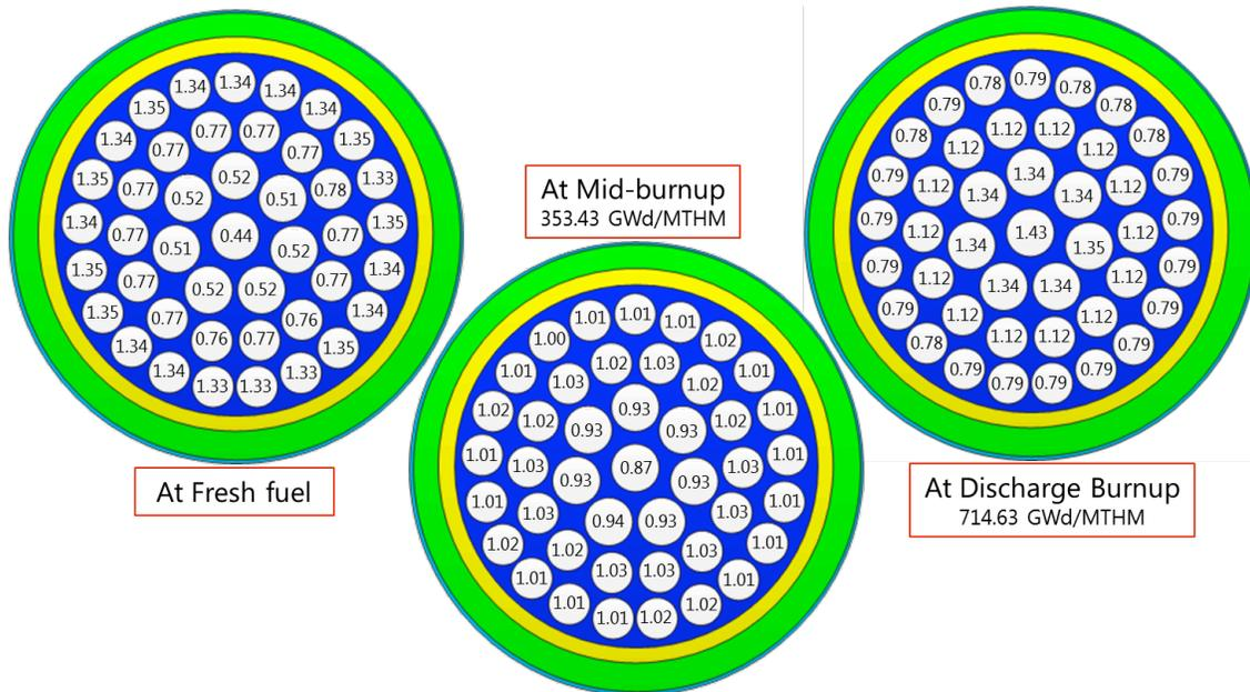
Figure 6. Normalized fission power distribution for regular kernel size PF=40%.
