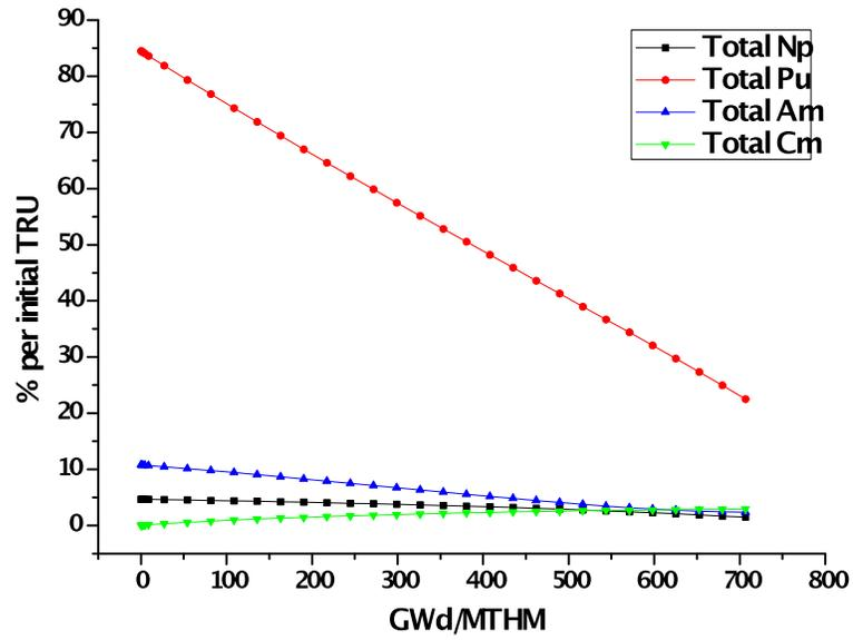
Figure 3. Transuranic composition vs. burnup for regular kernel size with PF=40%.
