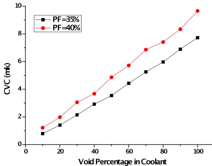
Figure 8. The coolant void reactivity for regular kernel size.
