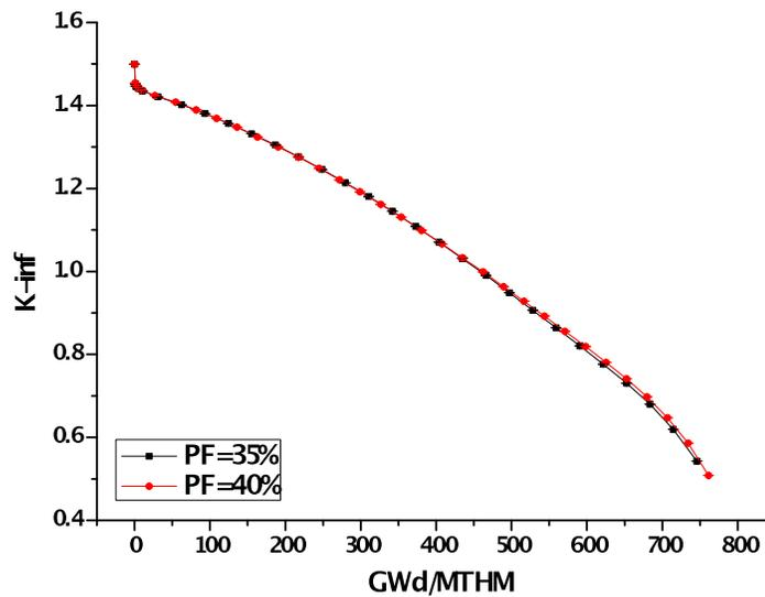
Figure 2. Infinite multiplication factor for regular kernel size.
