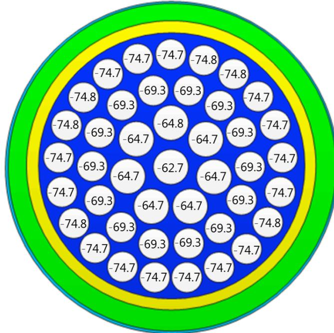
Figure 5. TRU discharge burnup distribution for regular kernel size with PF=40%.
