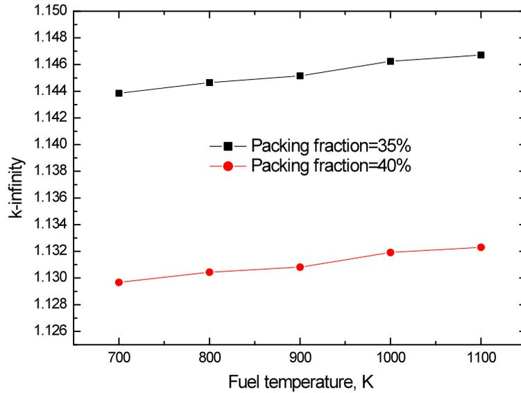
Figure 7. Impact of the SiC matrix temperature on the reactivity.
