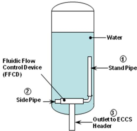
Fig. 5a: Accumulator tank with Fluidic Flow Control Device (FFCD)
