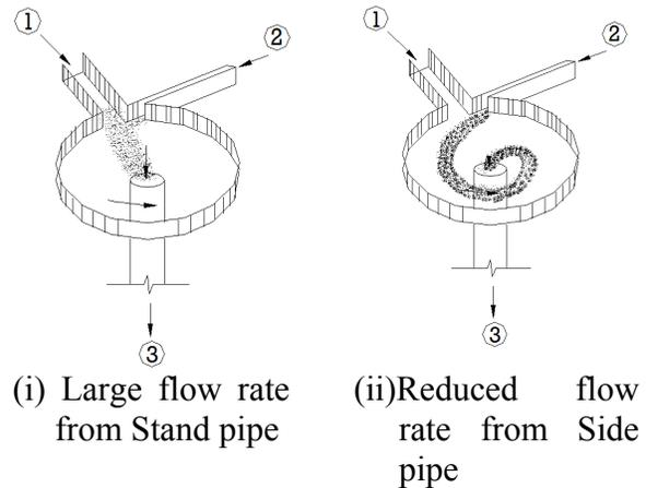
Fig. 5b: Details of FFCD
