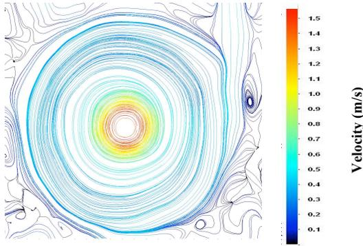
Fig. 5e: Velocity stream line and contour using PIV system
