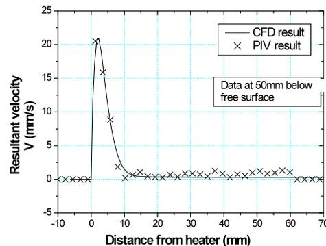
Fig. 4g: Comparison of PIV and CFD results at 50 mm below free surface of water
