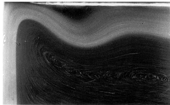
Fig. 4e: Flow visualization with aluminium particles
