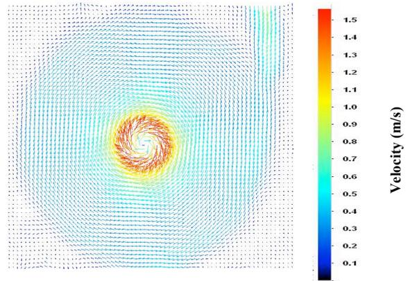
Fig. 5d: Velocity vector pattern using PIV system
