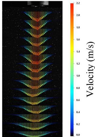
Fig. 3b: Velocity profile at different axial distances of submerged water jet by PIV system
