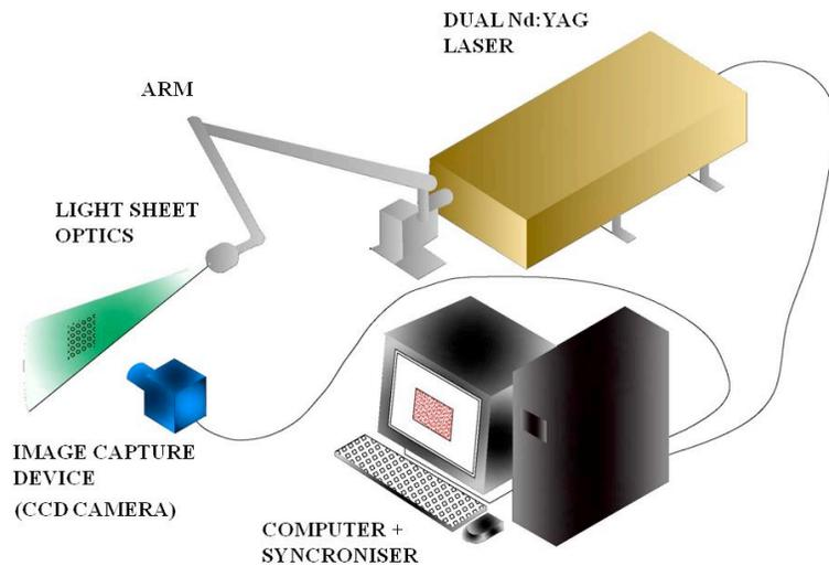
Fig. 1: Typical 2D PIV Setup
