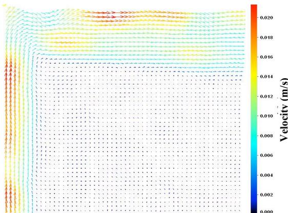
Fig. 4b: Velocity vector by PIV system
