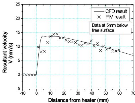
Fig. 4f: Comparison of PIV and CFD results at 5 mm below free surface of water
