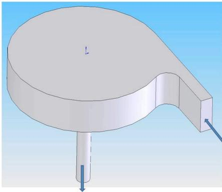
Fig. 5c: Schematic of Glass Fluidic flow device used in PIV experiment
