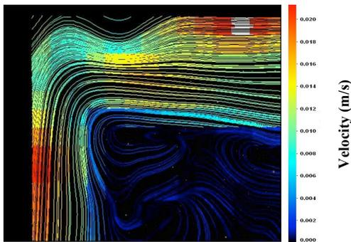
Fig. 4d: Velocity stream lines and contours by PIV
