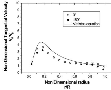
Fig. 5f: Tangential velocity distribution using PIV system
