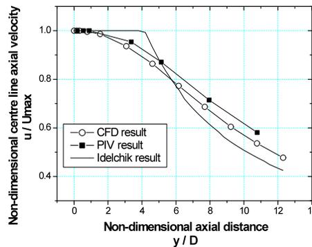
Fig. 3d: Comparison of PIV results, CFD results and Idelchik results for jet axial velocity
