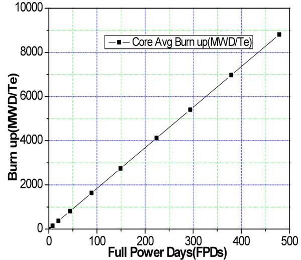
*Fig. 4(b) Core Avg. Burnup Vs FPD*
