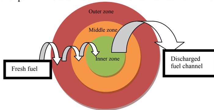
*Fig 7 Refueling with double reshuffling*
