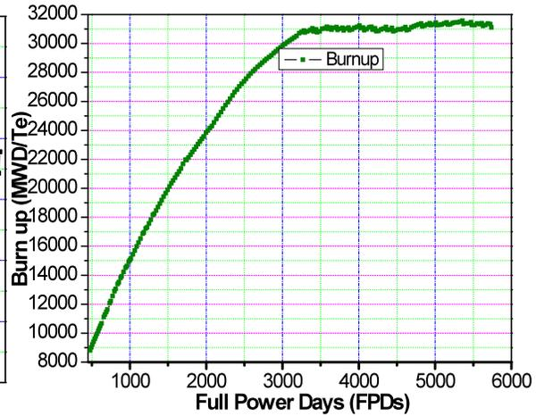
Fig. 8(b) Core avg burnup Vs FPDs
