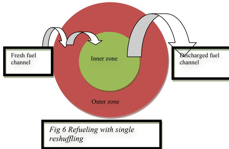
to replace the partially burnt fuel cluster and the partially burnt cluster from outer zone are moved to the inner zone to replace the highly burnt fuel cluster which is due for discharge to spent fuel bay. Hence, one refuelling operation requires one reshuffling operation as shown in fig 6.
