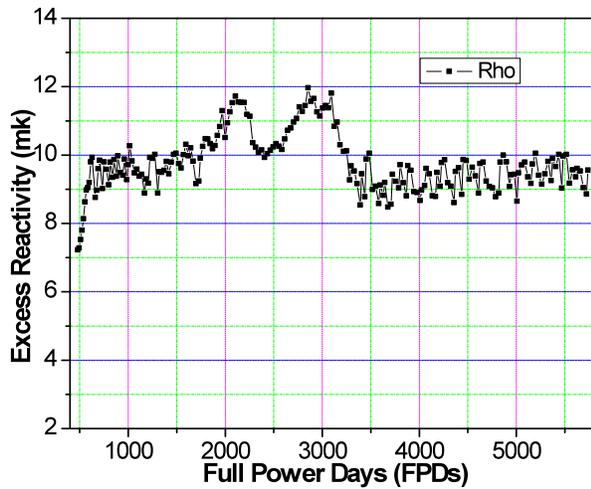
Fig. 8(a) Core excess reactivity Vs FPDs
