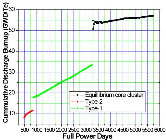
Fig. 10a Cumulative discharge burnup Vs FPD
