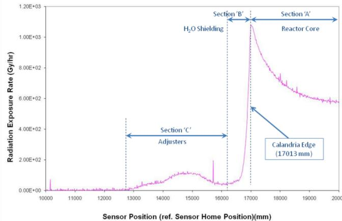
Figure 4 A plot of the  $\gamma$ -ray dose rate profile measured within the SUI tube.
