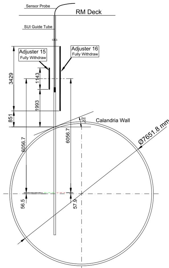
Figure 3 A diagram of the outer calandria wall, SUI guide tube and Adjuster Rods 15 and 16.
