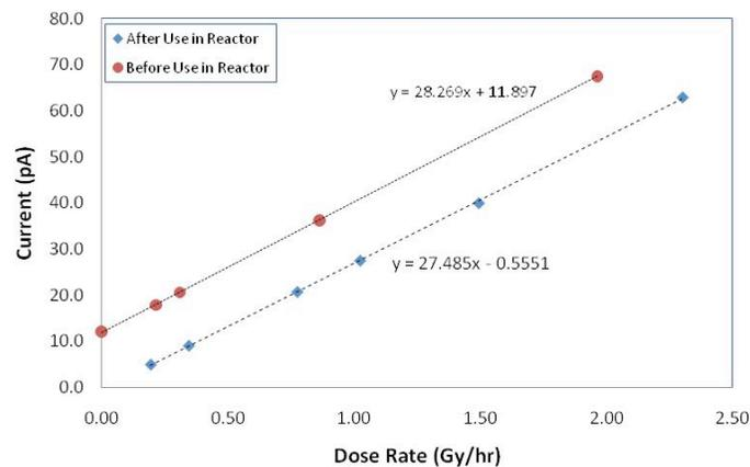
Figure 2 Plots of the diode current versus dose rate for the silicon diode sensor.
