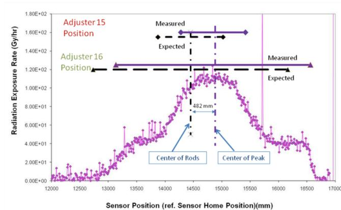
Figure 5 A plot of the measured  $\gamma$ -ray dose rate with the calandria's contribution removed.
