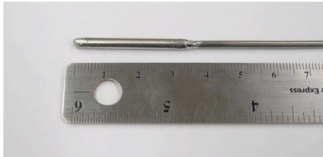
Figure 1 The silicon p-n junction diode sensor attached to a 30-m-long MI cable.
