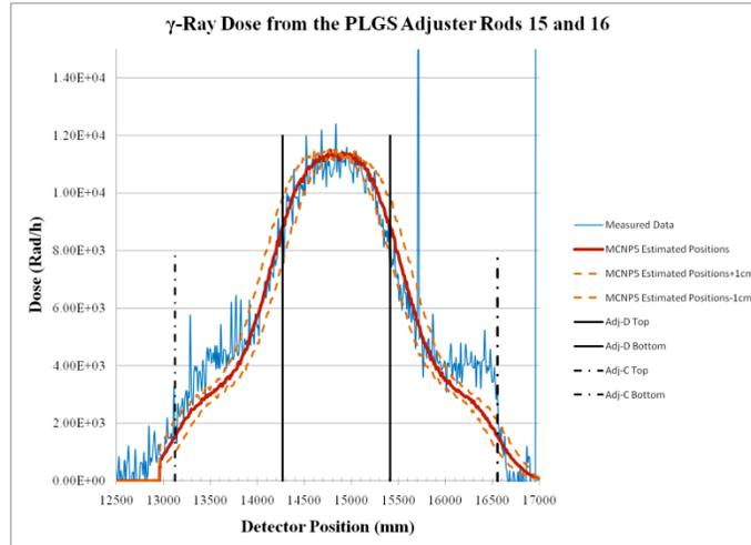
Figure 9 Overlaid plots of the measured and simulated dose rates due to Adjuster Rods 15 and 16. The adjuster rods were at their estimated locations, 10 cm above them and 10 cm below them.
