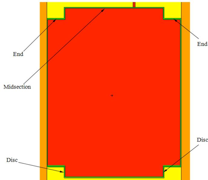
Figure 7 An MCNP5 visualization of the calandria midsection, ends and discs.
