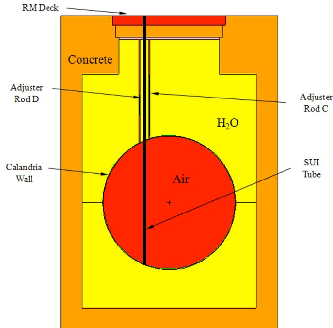
Figure 6 A visualization of the MCNP5 geometry used for the PLGS  $\gamma$ -ray profile simulations.
