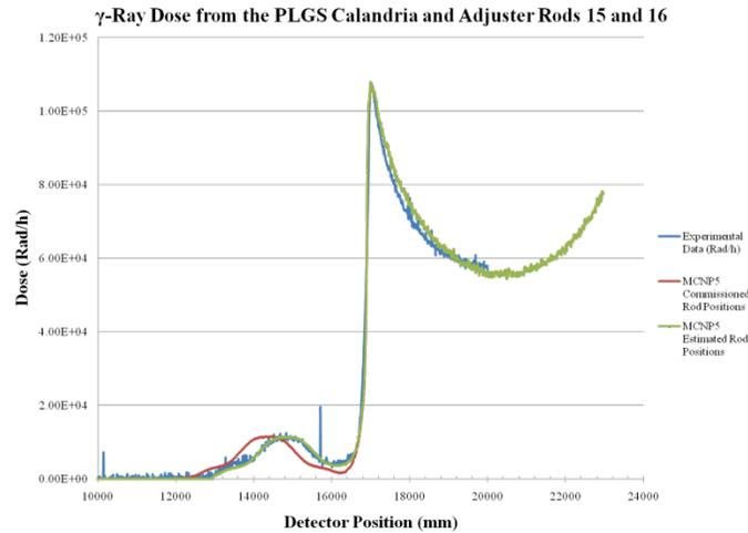
Figure 8 Overlaid plots of the measured dose rate and the simulated dose rates for the adjuster rods at their estimated positions and their expected positions during refurbishment.
