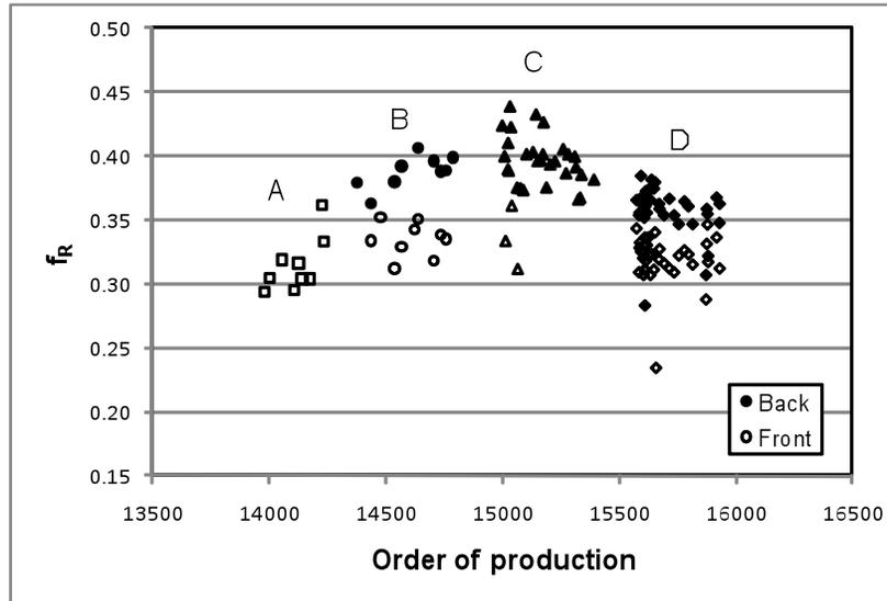
Figure 7. Radial texture parameters for the back-ends and front-ends of recent production tubes. The labels indicate different manufacturing routes.
