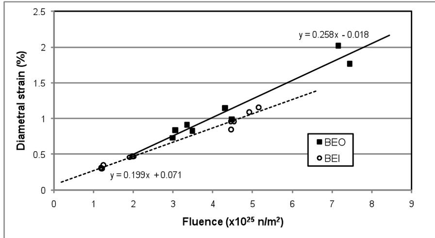
Figure 3. Diametral strain near outlet for pressure tubes in two CANDU reactors (same tubes as Figure 1 and 2); one unit installed with tube back-end at outlet (BEO) and one unit installed with tube front-end at outlet (BEI).
