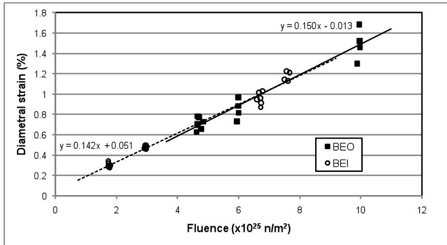
Figure 1. Diametral strain at axial midline of tube for pressure tubes in two reactors; one unit installed with tube back-end at outlet (BEO) and one unit installed with tube back-end at inlet (BEI).
