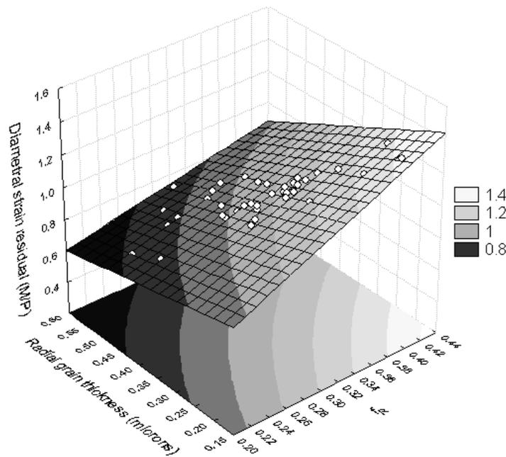
Figure 5. Diametral residuals (measured/predicted) fitted surface as a function of Kern's radial texture parameter and the mean radial grain thickness. White dots locate the predicted value of the diametral residuals for the observed texture and grain thickness (from Figure 4). Fitted model provided in Table 1.
