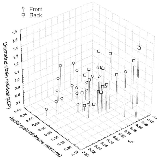
Figure 4. Diametral residuals as a function of the Kern's radial texture parameter and the mean radial grain thickness from historical CANDU pressure tubes. Drop lines end at the texture/grain thickness plane as a visual aid to help see the 3D perspective.
