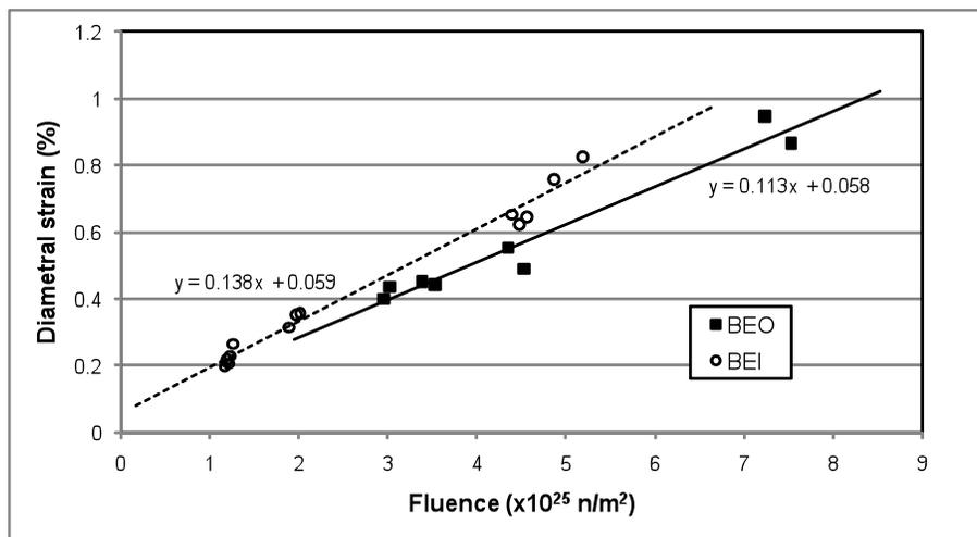
Figure 2. Diametral strain near inlet for pressure tubes in two CANDU reactors (same tubes as Figure 1); one unit installed with tube front-end at inlet (BEO) and one unit installed with tube back-end at inlet (BEI).
