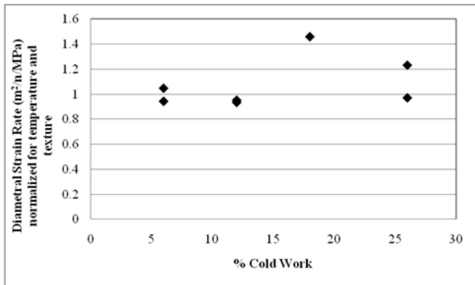
Figure 9. Trillium 5 normalized diametral strain rates showing no significant dependence on cold work.
