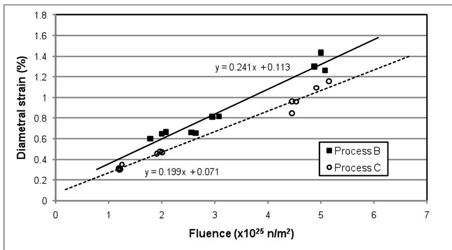
Figure 8. Diametral strain near the outlet for pressure tubes in two CANDU reactors (both installed as BEI). This figure compares diametral strain of tubes made following Process B and Process C under near identical operating conditions.
