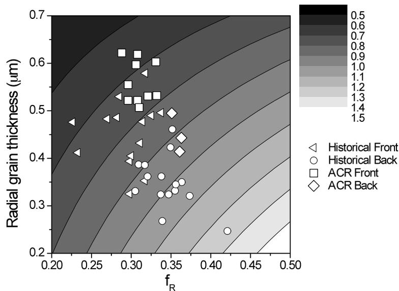
Figure 6. Contour plot of the response surface. The contour lines and gray scale indicate the diametral strain residual (M/P). Data points overlaid on the contour plot are the coordinates of the microstructure attributes for various pressure tubes. The historical data is the same as the fitted data from Figures 4 and 5.
