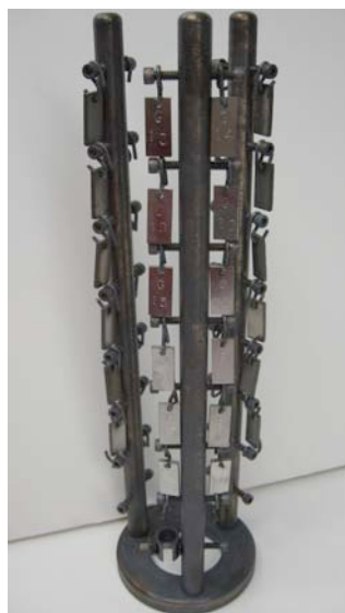
Figure 2. Picture of coupon tree loaded with samples of the two steels.
