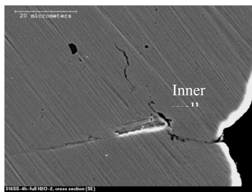
Figure 6 The cross section of the 316 SS tube that did not rupture after testing at 500°C for 4 h. The tube was fully filled with water before exposure.
