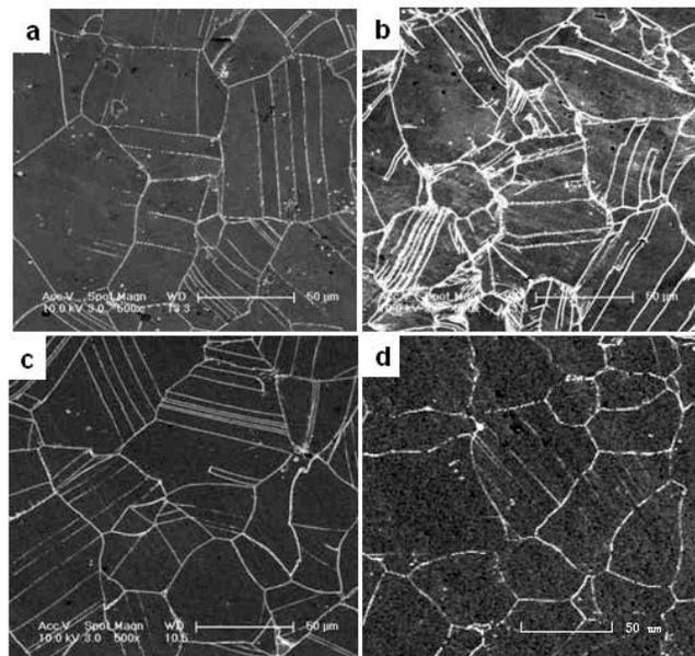
**Fig.4 SEM cross-section investigations of specimens ruptured at 650°C under (a) 430 MPa ( $t_r=76$  h); (b) 400 MPa ( $t_r=143$  h); (c) 300 MPa ( $t_r=400$  h); and (d) 260 MPa ( $t_r=650$  h).**
