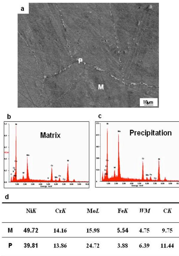
**Fig.5 C-276 ruptured at 650 °C under 430 MPa ( $t_r=76$  h) ( a ) Back scattering image; (b) EDS of the matrix; (c) EDS of the precipitates; (d) Comparison of the composition between the matrix and the precipitates.**
