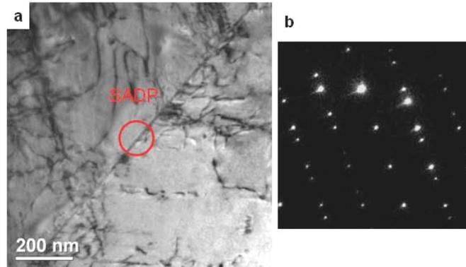
**Fig.3 (a) Bright-field TEM image of as-received C-276 alloy; (b) Selected area diffraction pattern (SADP) taken from the grain boundary spot indicated in (a).**
