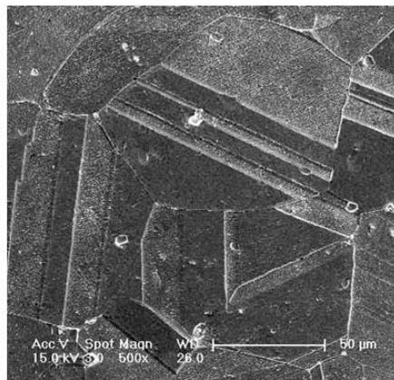
**Fig.2 SEM image of as-received C-276 alloy.**
