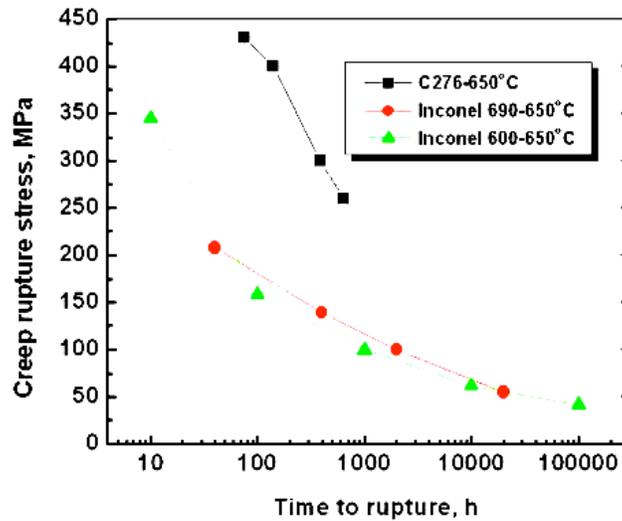
**Fig.1 Rupture stress vs. time of C-276 alloy tested at 650°C under various stresses, compared with Inconel-690 and Inconel-600 alloys.**
