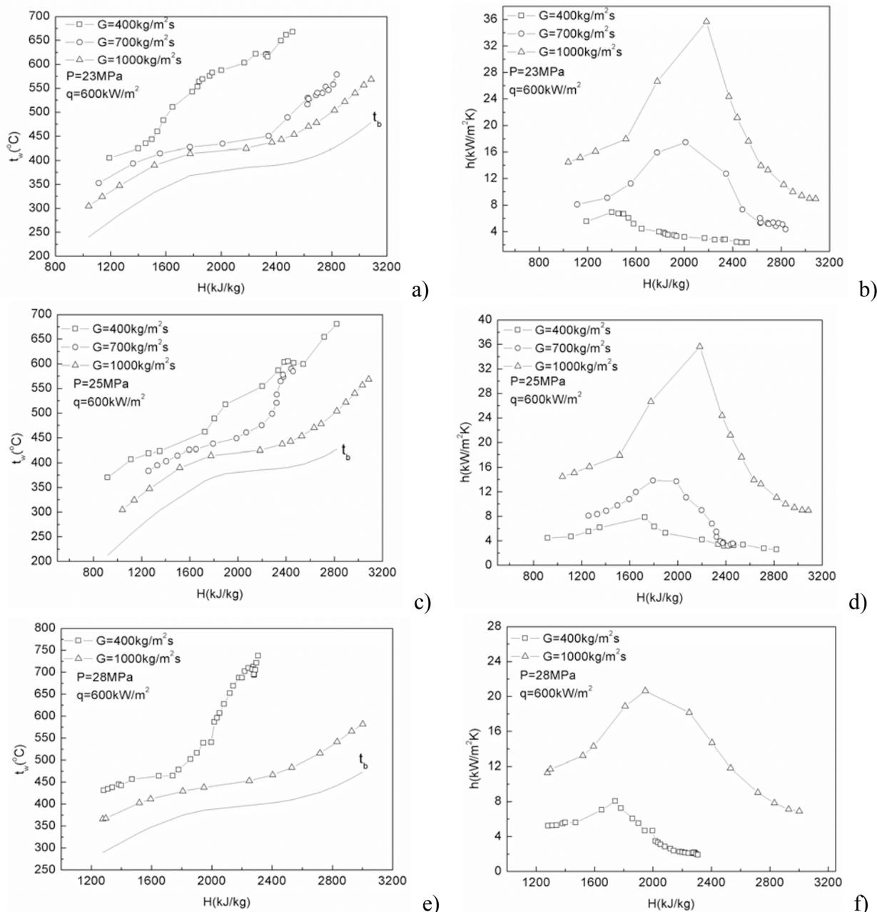
Fig.4 Comparison of the wall temperatures and HTC at different mass fluxes
