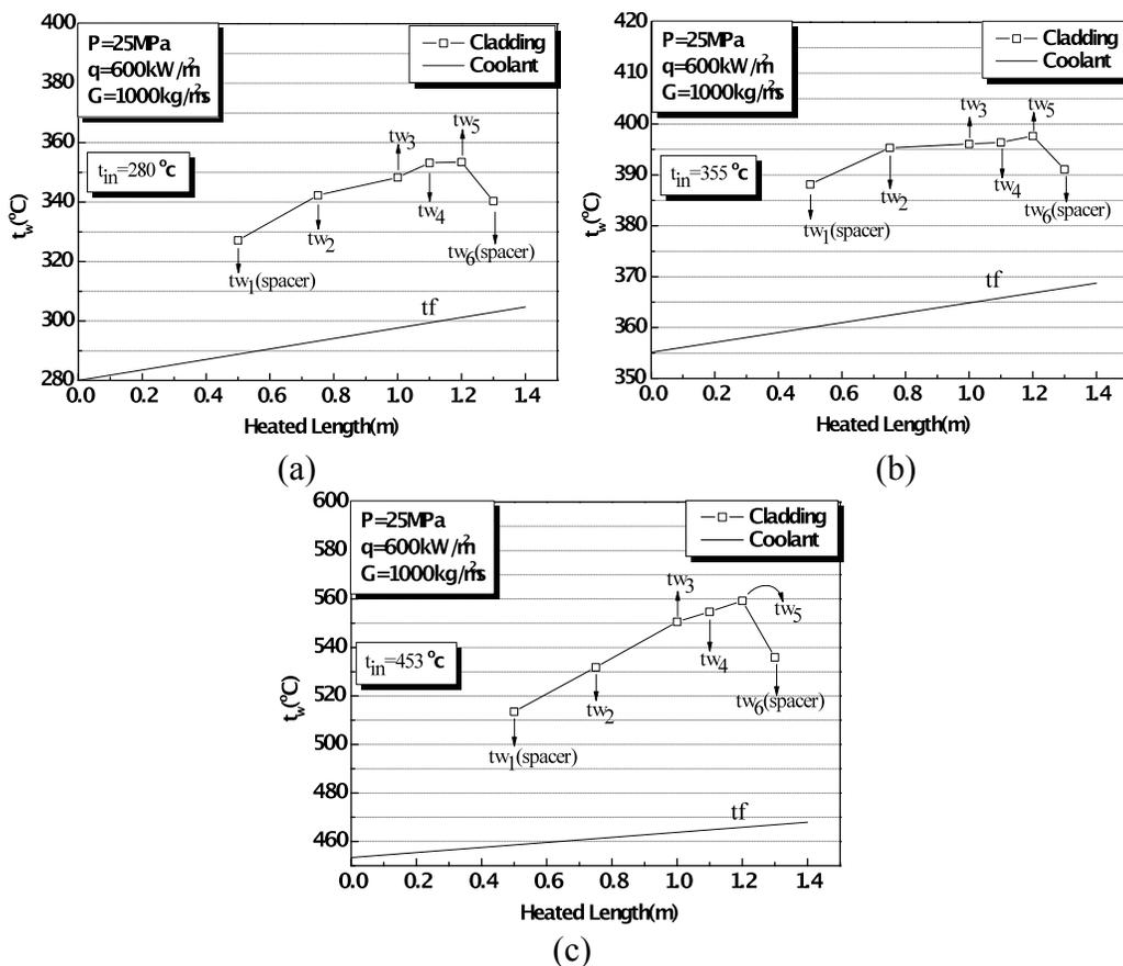
Fig.7 Wall temperature distribute along the heater length
