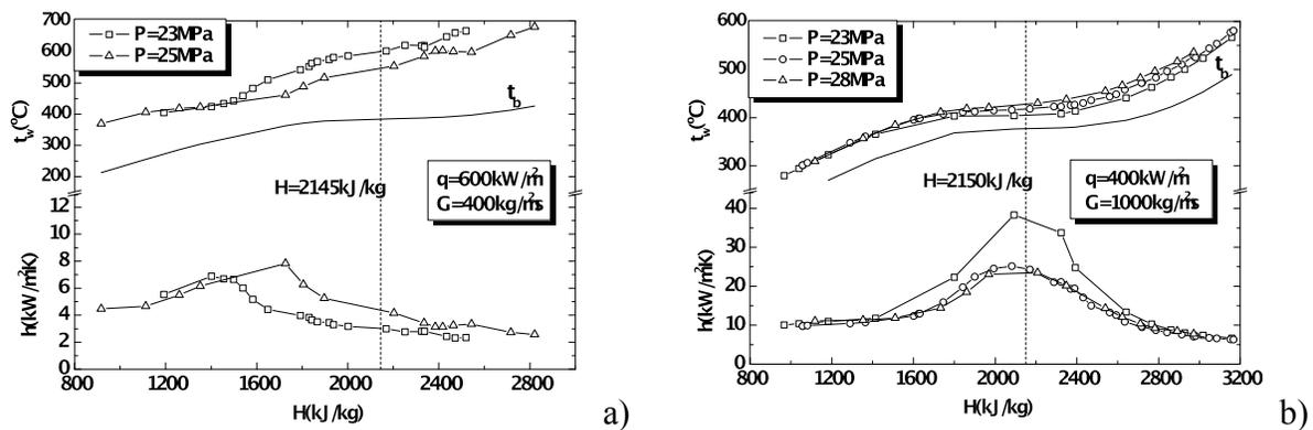
Fig.6 Comparison of the wall temperatures and HTC at different pressure
