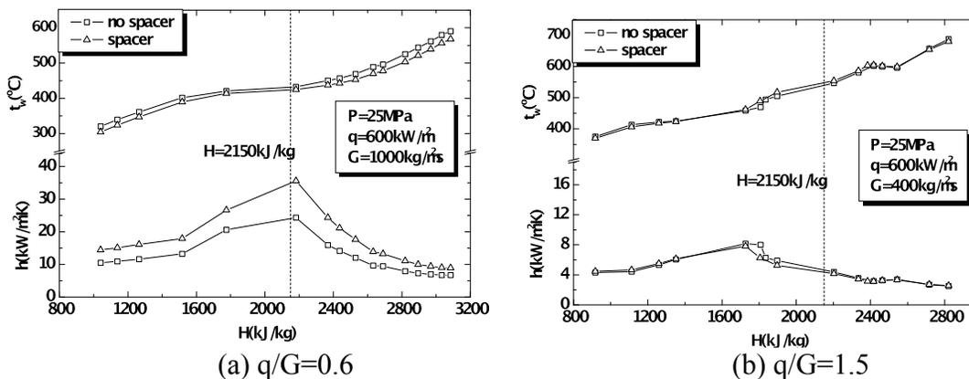
Fig.8 Comparison of the wall temperatures and HTC with and without spacer
