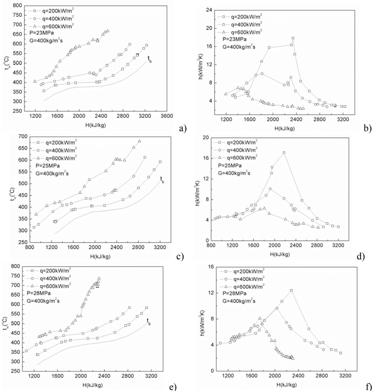
Fig.5 Comparison of the wall temperatures and HTC at different heat fluxes
