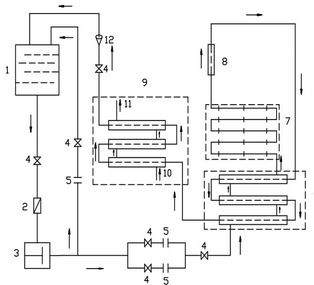
1: Water tank; 2: Filter; 3: Water pump; 4: Valve; 5: Orifice;
