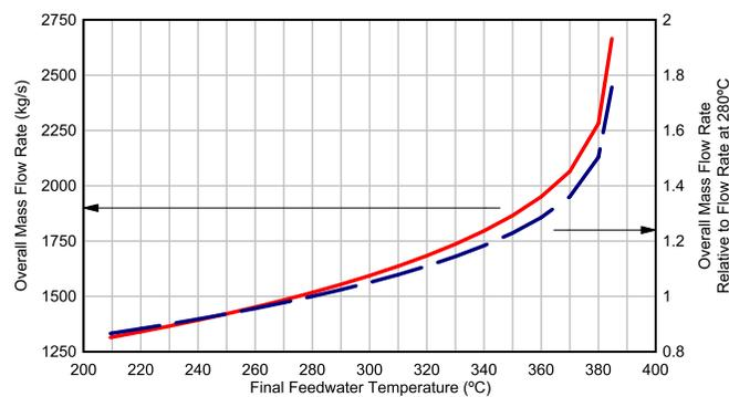
Figure 4 Effect of final feedwater temperature on overall cycle mass flow rate.
