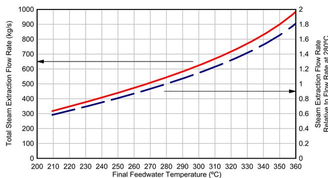
Figure 5 Effect of final feedwater temperature on the steam extraction flow rate (solid line). The effect of final feedwater temperature on steam extraction flow rate relative to that at 280°C (dashed line).
