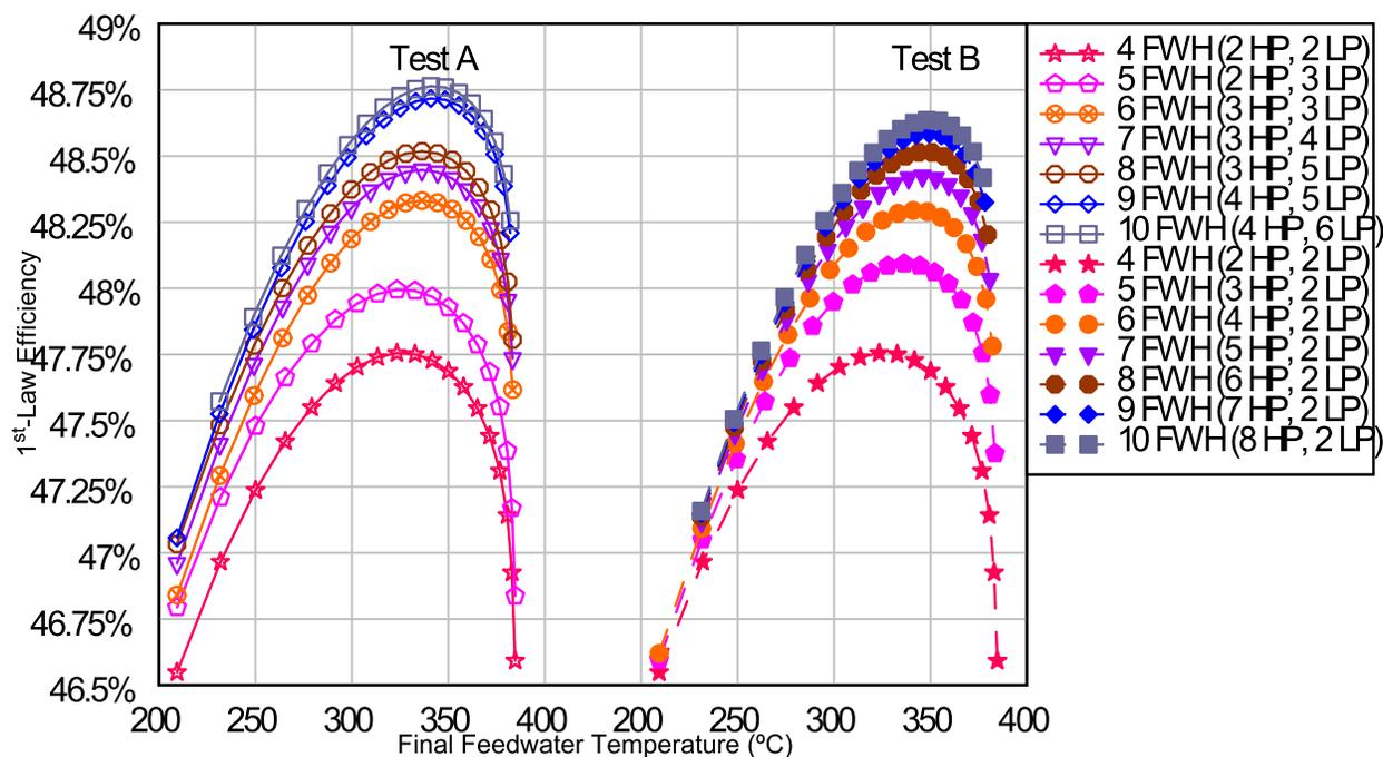
Figure 3 The effect of adding feedwater heaters to a basic 4-feedwater heater model on cycle efficiency. The origin of the extraction line (in parentheses in the legend) is seen to have an effect.
