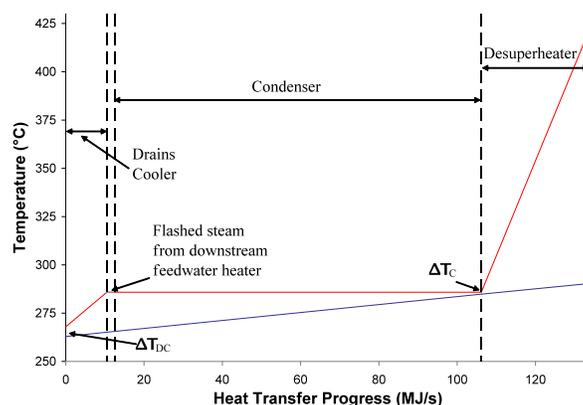
Figure 1 T-Q diagram of a typical heat exchanger with desuperheating, condensing and drains cooling sections.
