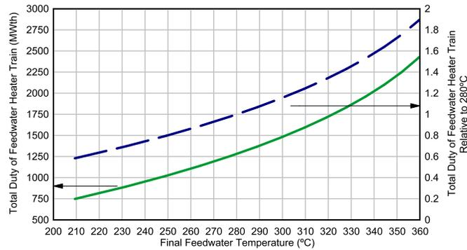
Figure 6 Effect of final feedwater temperature on the sum of the heat transfer within the feedwater heater train (solid line). The effect of final feedwater temperature on the sum of the heat transfer within the feedwater heater train relative to that at 280°C (dashed line).
