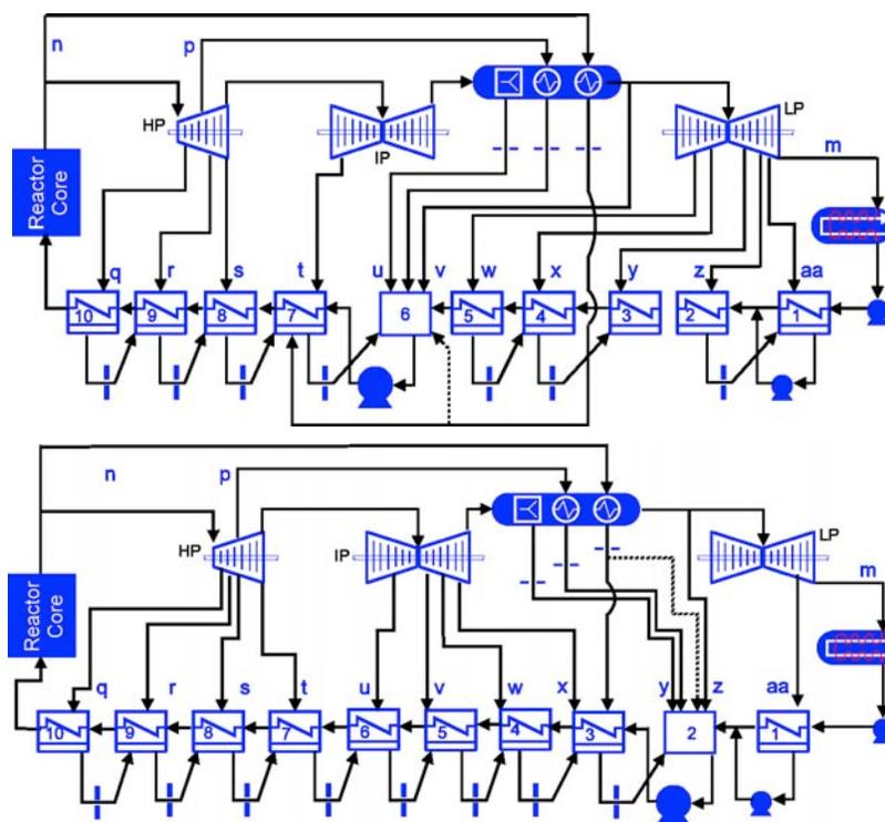
Figure 2 Plant models for Test A (top) and Test B (bottom) with 10 feedwater heaters.
