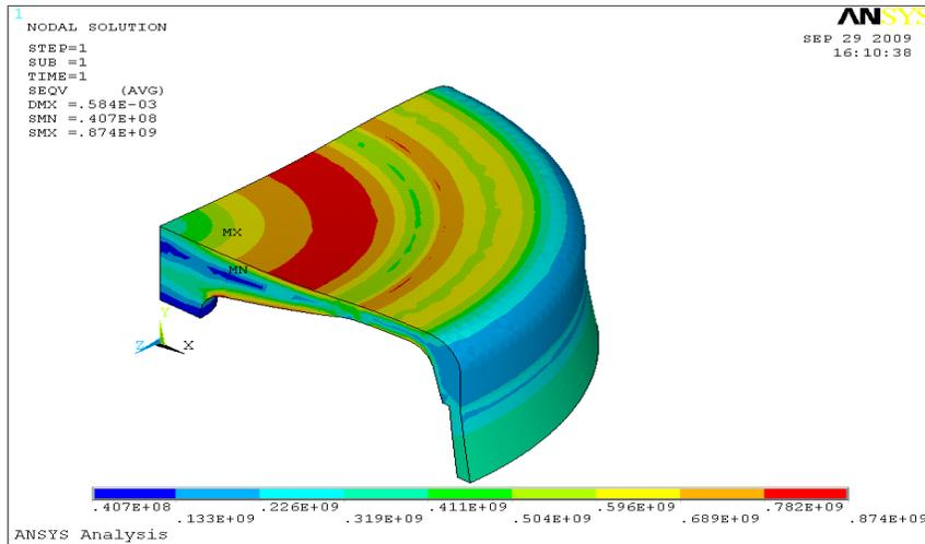
Figure 9 ANSYS calculation of the stress on the seal element and seal disk shown in Figure 8.
