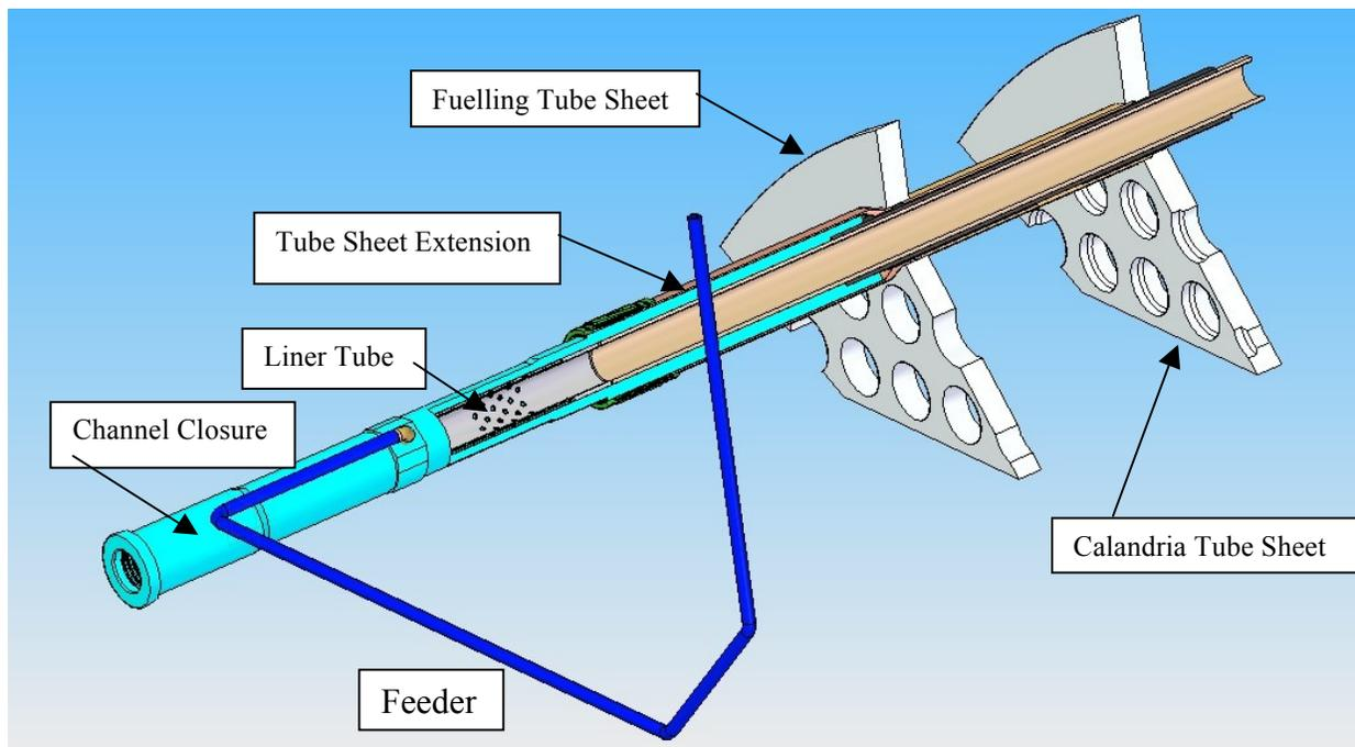
Figure 4 Solid model of one concept of the input end of a SCWR fuel channel.
