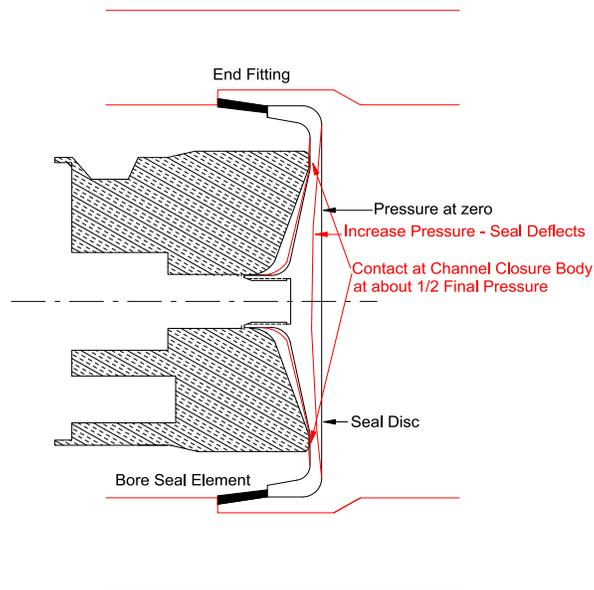
Figure 8 Application of the bore seal.
