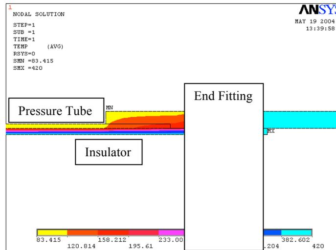
Figure 5 Temperature distribution at the rolled joint region for the insulated pressure tube to end fitting transition.
