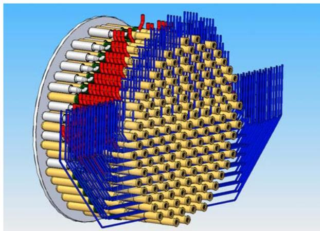
Figure 13 Solid 3-D model of the face of a SCW reactor built in a horizontal orientation.
