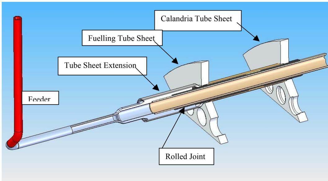
Figure 10 Solid model of one concept of the input end of a SCWR fuel channel.
