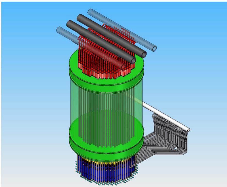
Figure 14 SCW Reactor Concept – Vertical Orientation
