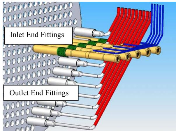
Figure 12 The assembly of inlet and outlet end fittings and feeders.
