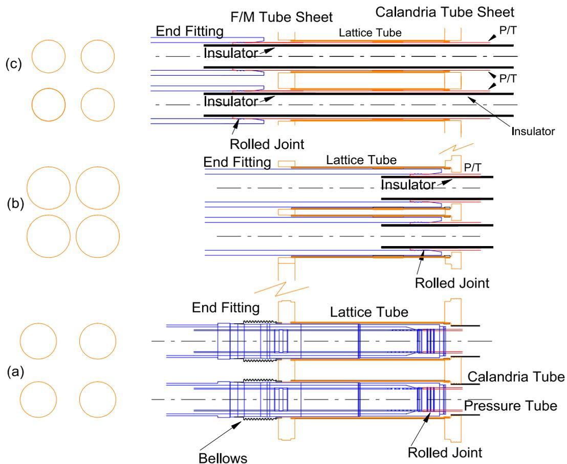
Figure 3 Key out-of-core components of CANDU reactors.
