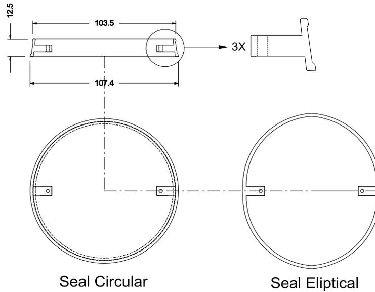
Figure 7 Principle of bore seal element.
