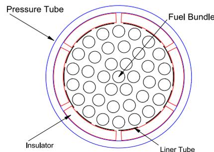
Figure 1 Illustration of High-Efficiency Fuel Channel.
