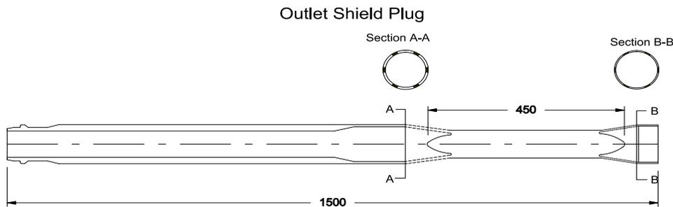
Figure 11 Outlet Shield Plug. The design is meant to provide substantial line-of-sight shielding with high-density stainless steel with minimal flow resistance to the outlet coolant.
