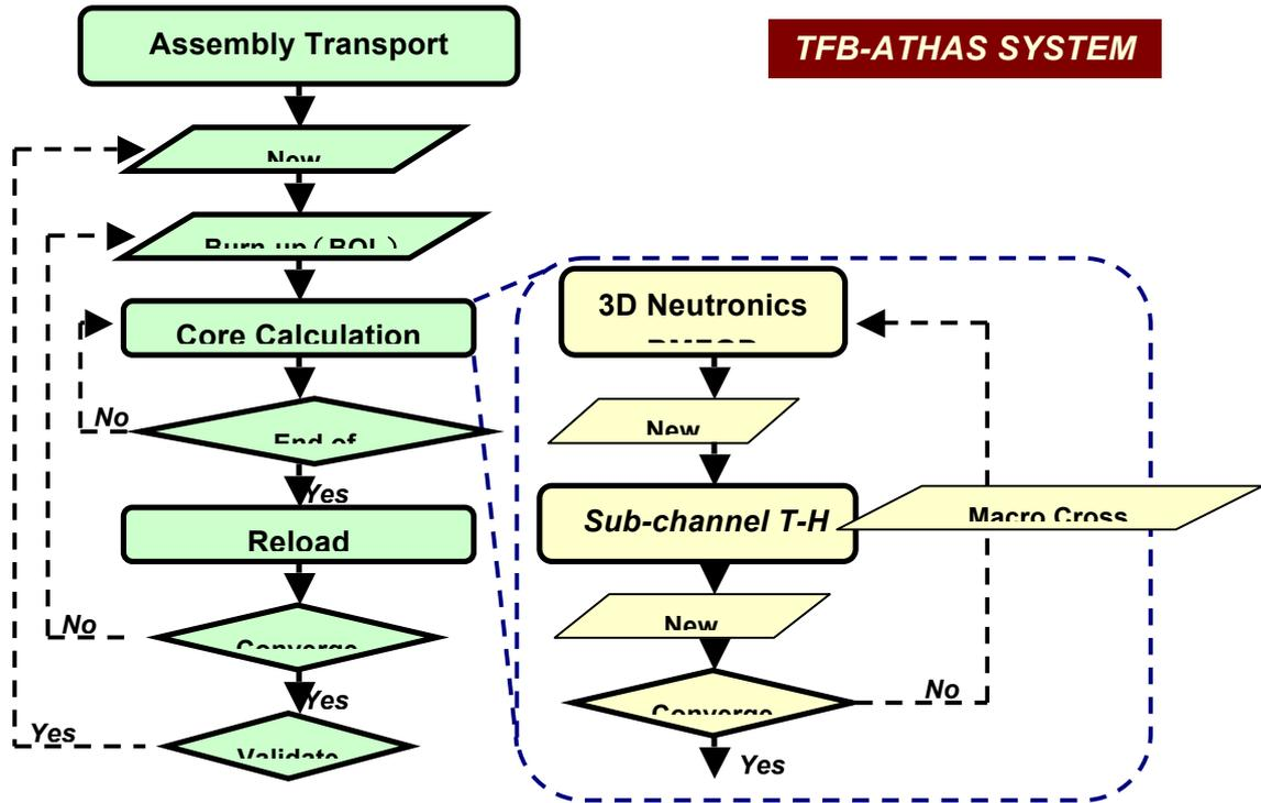
TFB-ATHAS SYSTEM is builed by 3 codes, which are TPFAP-E ( Assembly neutron transport), BMFGD ( 3D diffusion finite difference), and ATHAS ( Sub-channel thermal-hydraulic).
