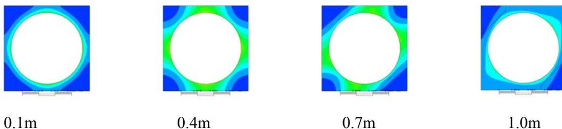
Figure 12 Temperature contour along channel with equal distance
