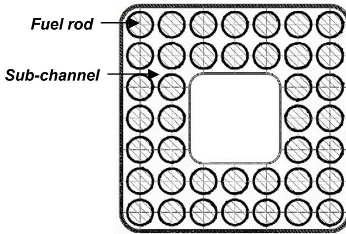
Figure 16 Assembly of SCWR
