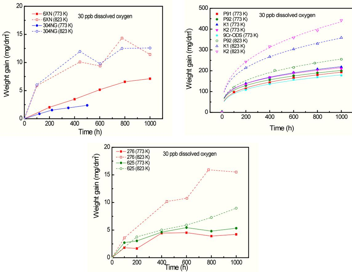
Figure 10 Results of the corrosion experiments
