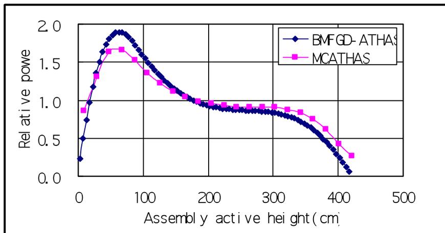
Figure 18 Axial relative power distribution of assembly
