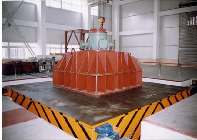
Figure 6 6m×6m Seismic Rig
