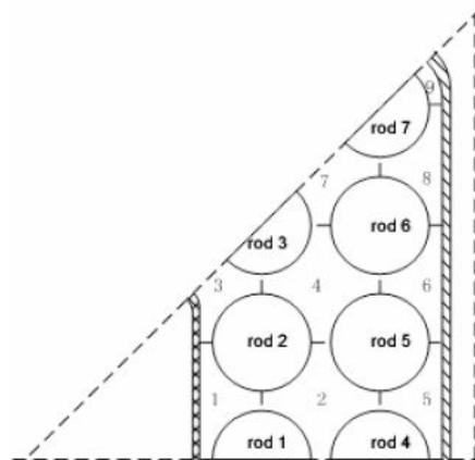
Figure 17 1/8 Assembly of SCWR
