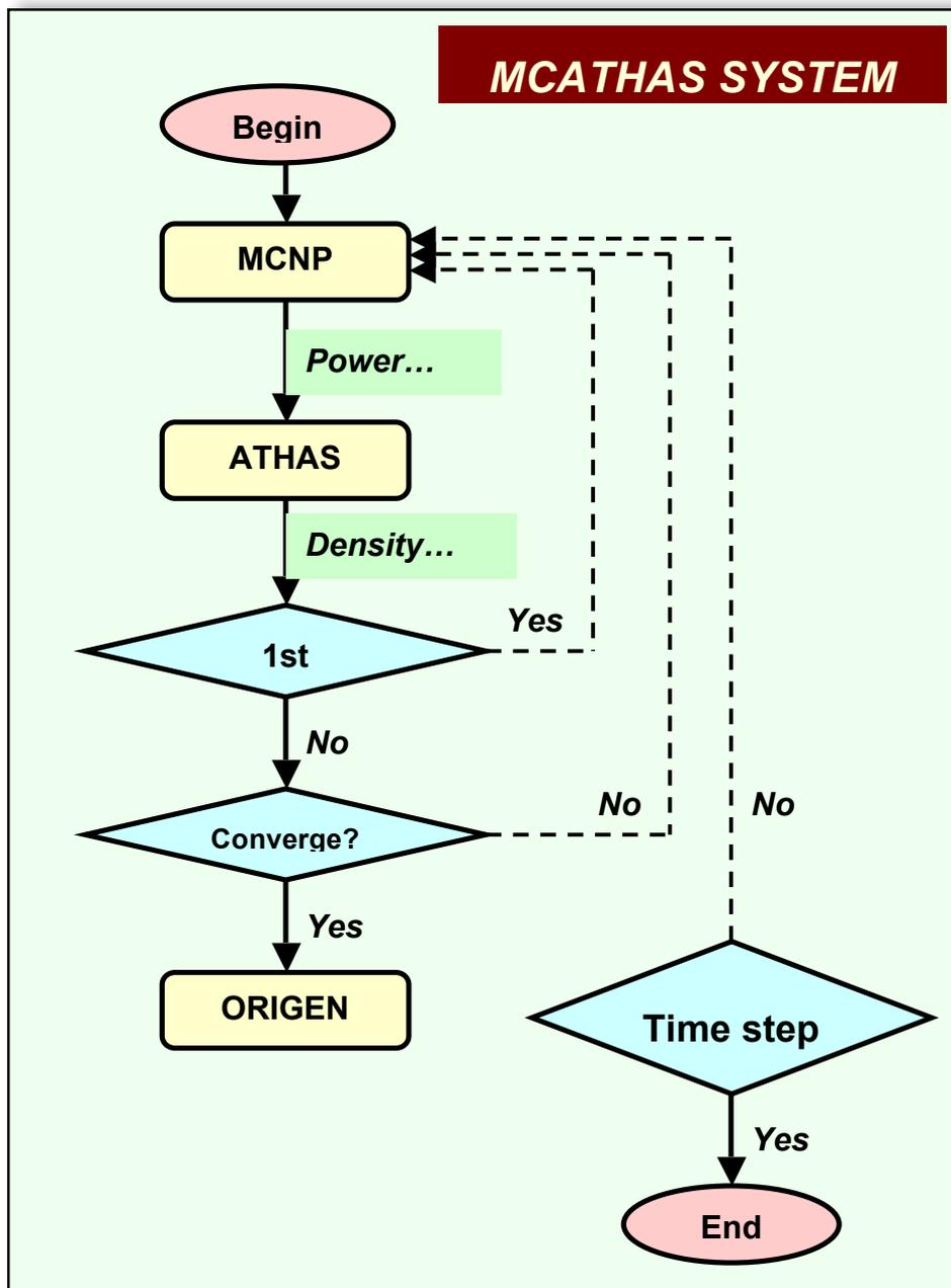
Figure 14 the structure of the codes
