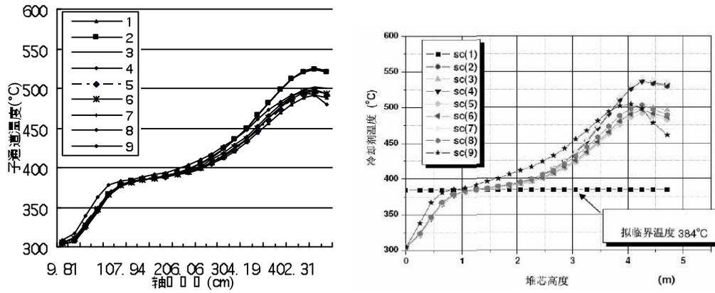
Figure 15 Axial coolant temperature distribution of sub-channel
