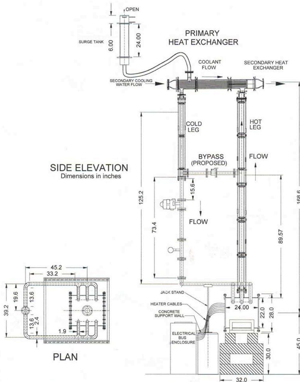
Figure1 PT-SCWR Moderator Cooling Test Loop
