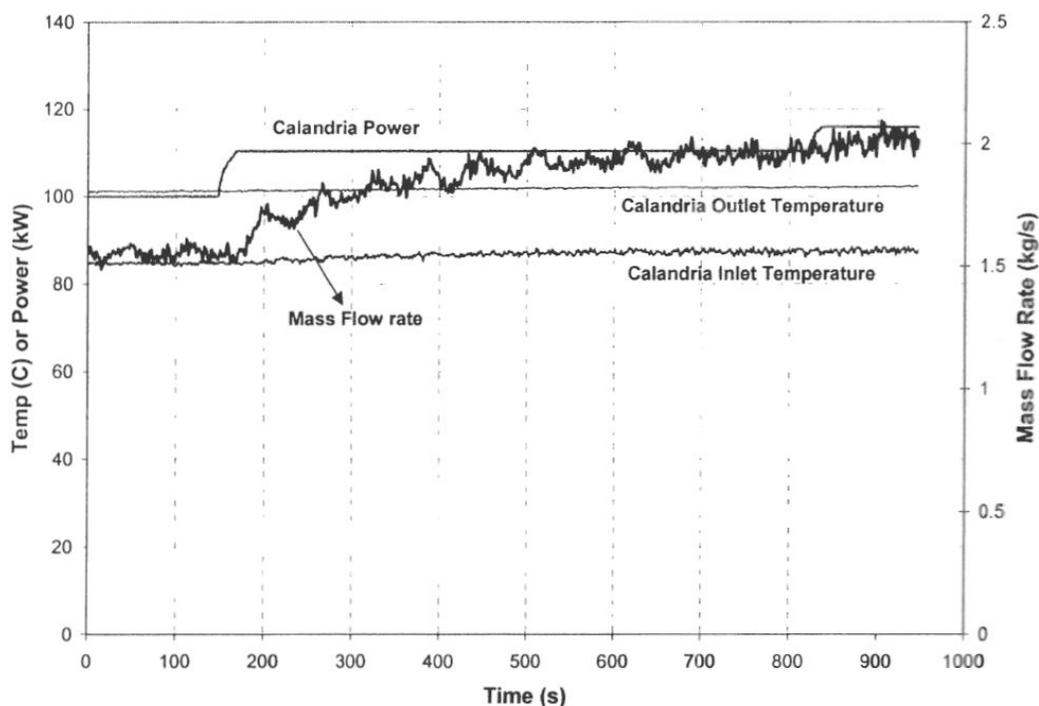
Figure 5 The experiment data of the test loop
