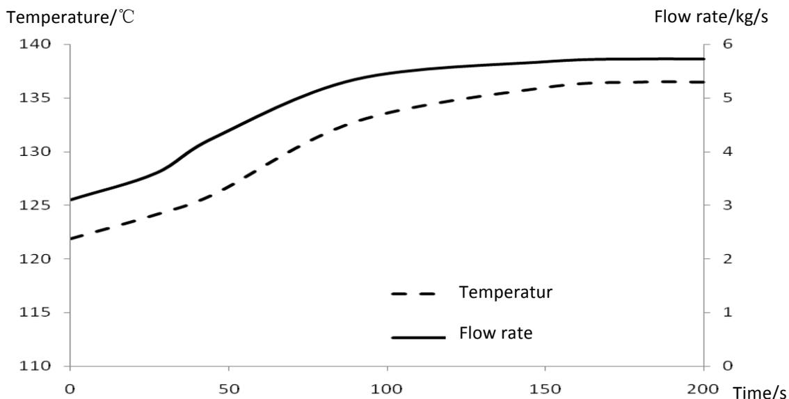
Figure 9 The flow rate and temperature of loop variation by time
