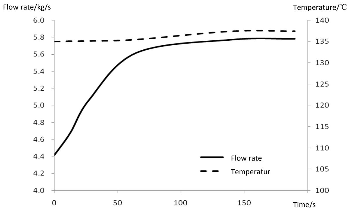
Figure 6 The flow rate and temperature of loop
