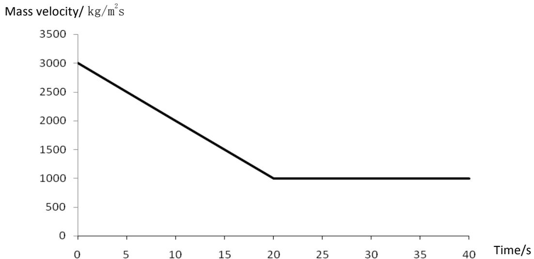
Figure 8 The change condition of cooling water mass velocity
