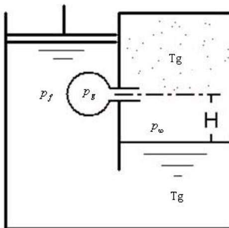
Fig 2 The schema of bubble growing
