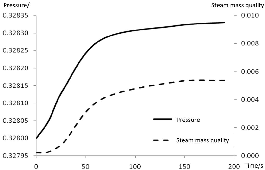
Figure 7 The pressure and steam mass quality
