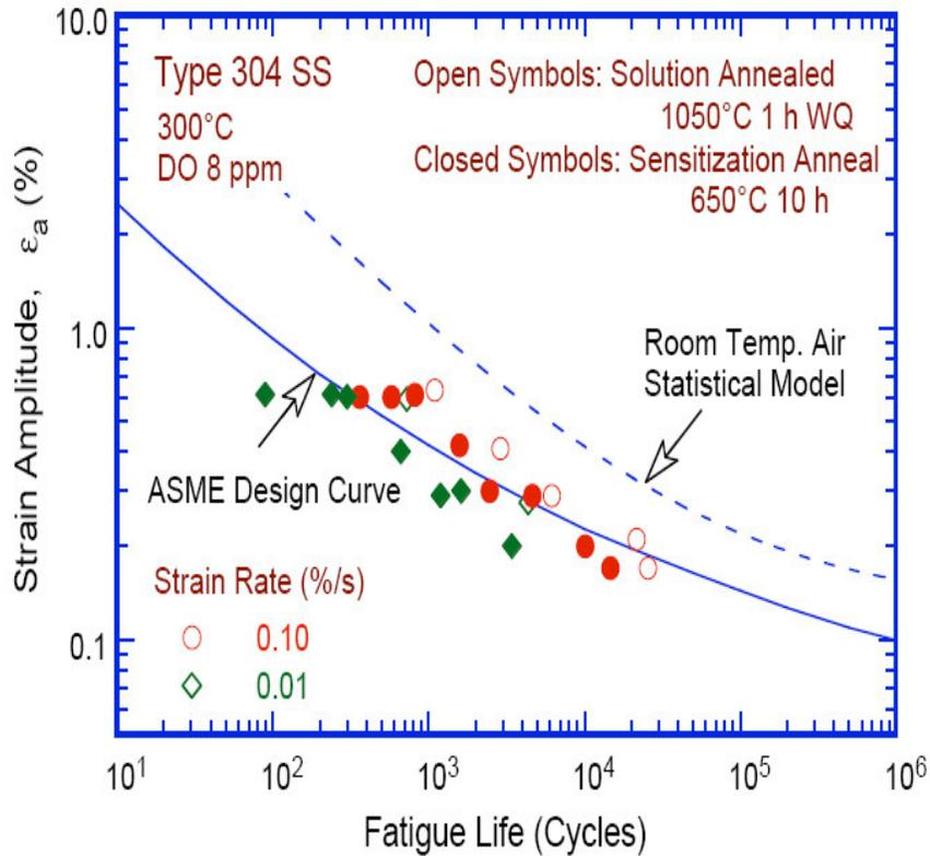
Figure 4. ASME design curve for 304 ss used in subcritical water (Courtesy of ANL)
