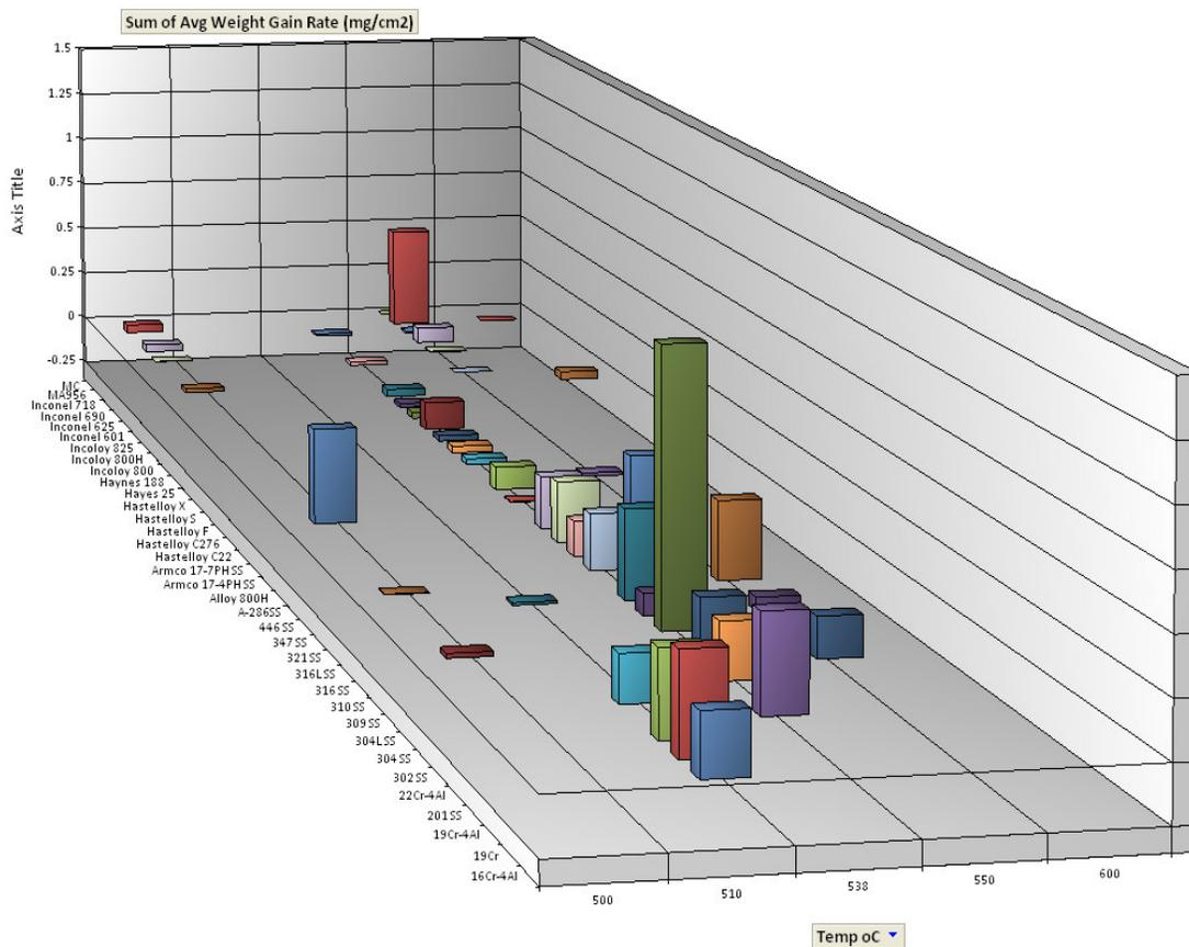
Figure 2. Variation of corrosion rate as a function of temperature using the data collected in the MTL-AECL Corrosion database [6, 9] (only alloys with Cr content greater than 16% are plotted)
