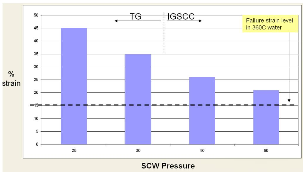
Figure 3. Variation in SCC susceptibility and change in failure mode as a function of water pressure for 316 tested at 400 °C and a strain rate= $2.78 \times 10^{-6}$  s<sup>-1</sup> (Graph generated using data in [15])
