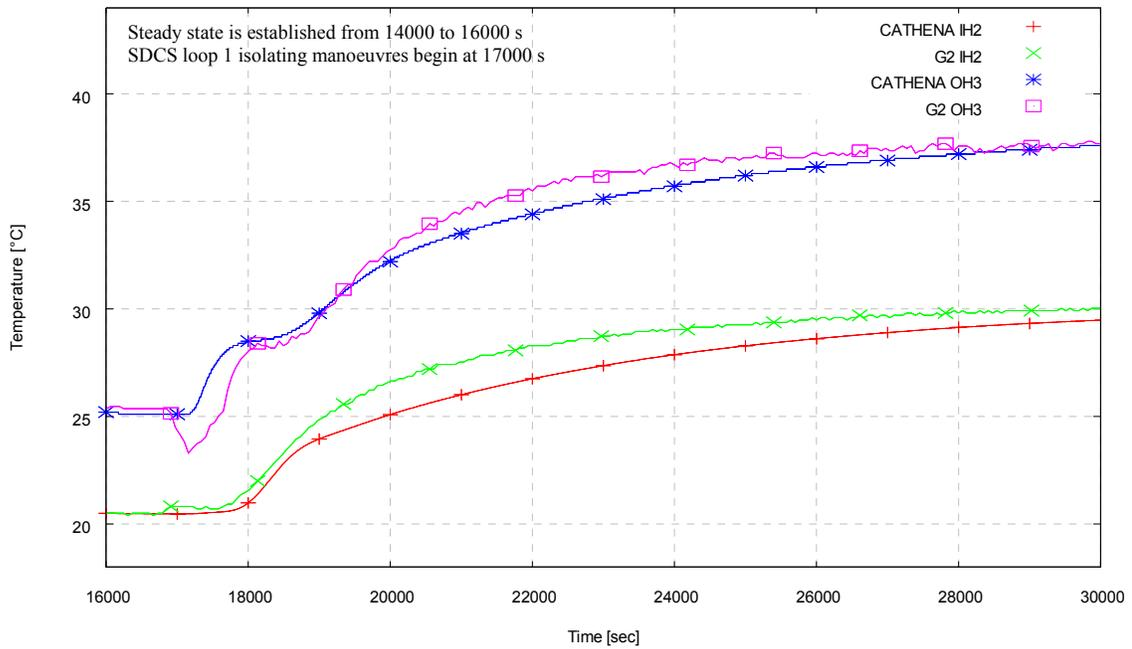
**Figure 18 : Transient Temperature at Inlet Header 2 (IH2) and Outlet Header 3 (OH3)
