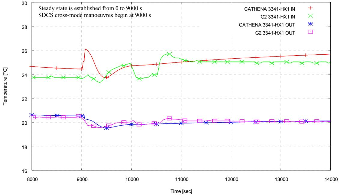
**Figure 14 : Transient Temperature at SDCS Heat Exchanger 3341-HX1 (case #2 : 0.22%PP)**
