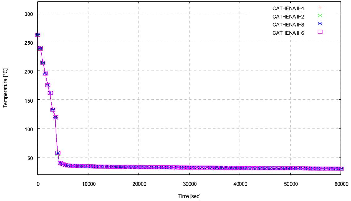
**Figure 6 : Inlet Headers (IH) Temperature (case #1)**
