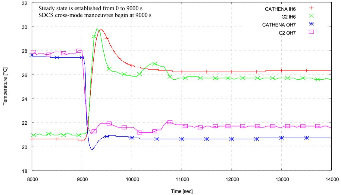
**Figure 12 : Transient Temperature at Inlet Header 6 (IH6) and Outlet Header 7 (OH7)
