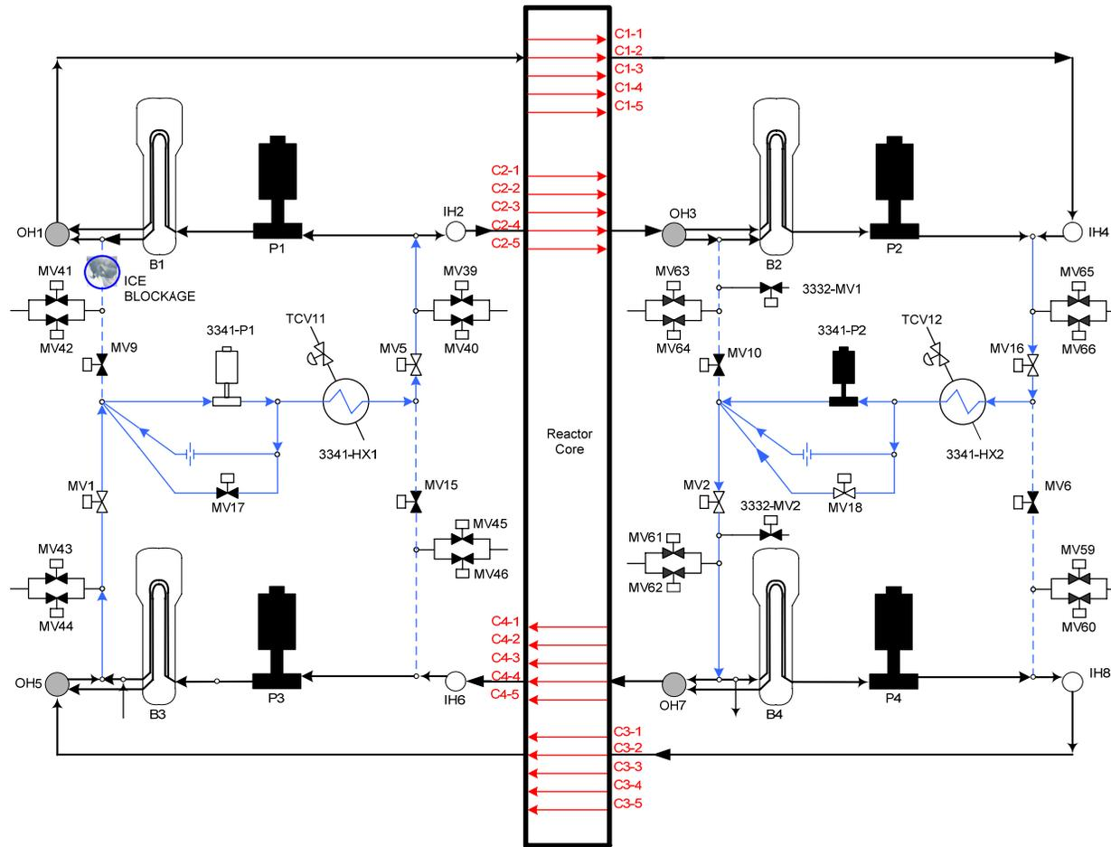
Figure 4: Flow Path of the PHTS and SDCS in Cross-mode with 3341-P2 Stopped (case #2)
