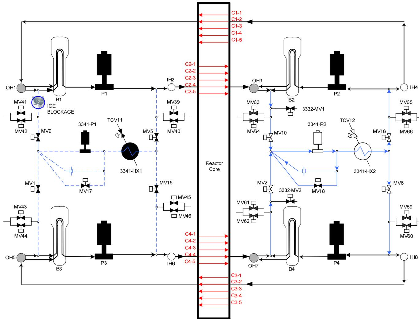
**Figure 5 : Flow Path of the PHTS and SDCS in Cross-mode with SDCS Loop 1 Isolated (case #3)**
