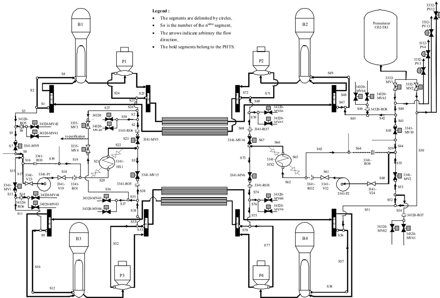
Figure 1 : PHTS and SDCS Circuits Segmentation
