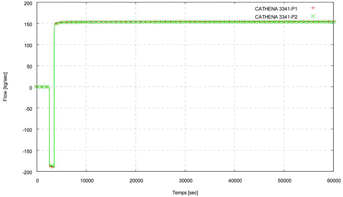
**Figure 8 : Flow through SDCS Pumps (case #1)**
