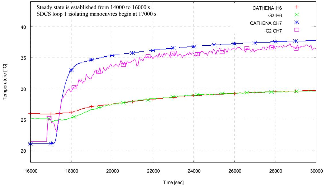
**Figure 19 : Transient Temperature at Inlet Header 6 (IH6) and Outlet Header 7 (OH7)
