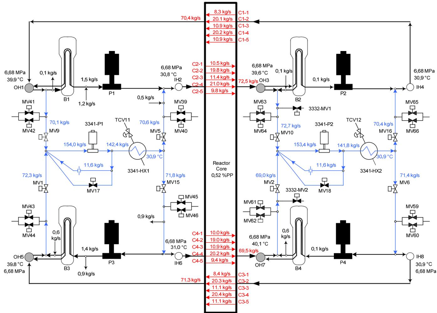
Figure 9: Plant Conditions after 50000 sec (case #1)
