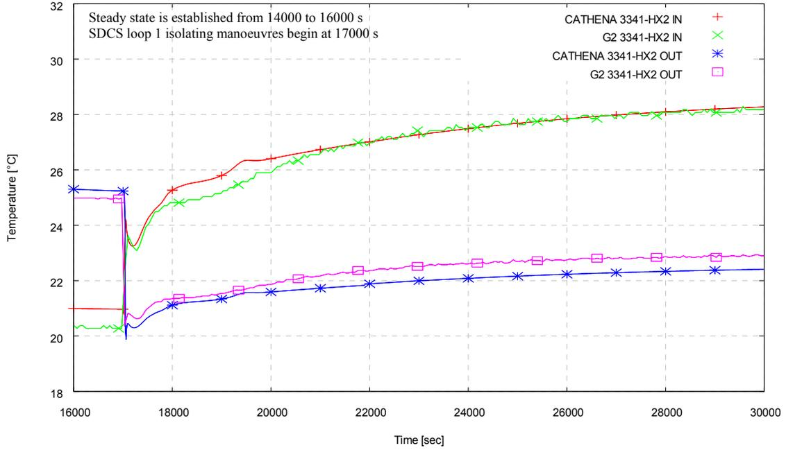
**Figure 21: Transient Temperature at SDCS Heat Exchanger 3341-HX2 (case #3 : 0.18%PP)**
