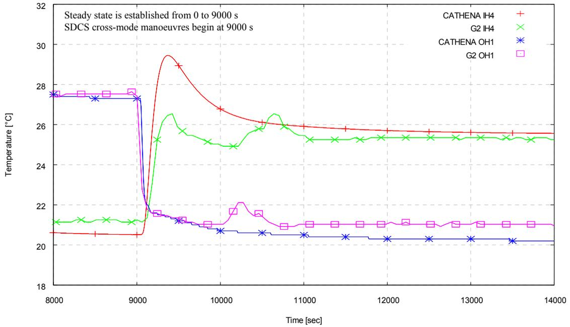
**Figure 10 : Transient Temperature at Inlet Header 4 (IH4) and Outlet Header 1 (OH1)
