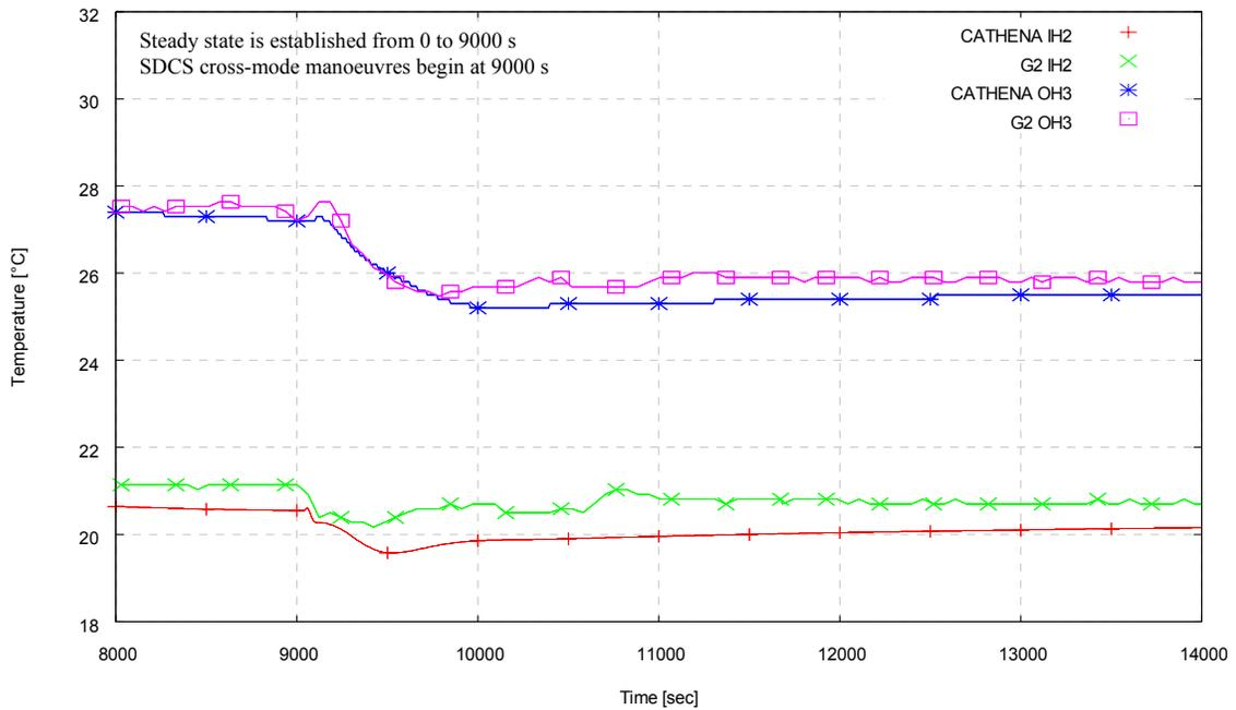
**Figure 11 : Transient Temperature at Inlet Header 2 (IH2) and Outlet Header 3 (OH3)
