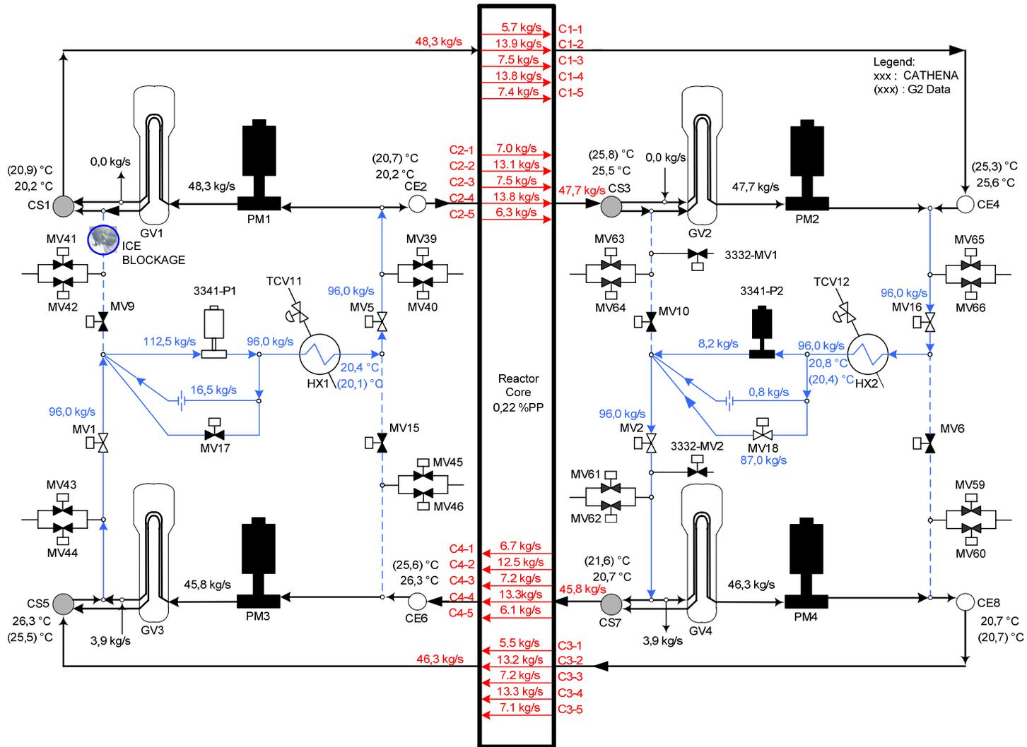
Figure 16 : Steady Plant Conditions after 14000 sec (case #2)
