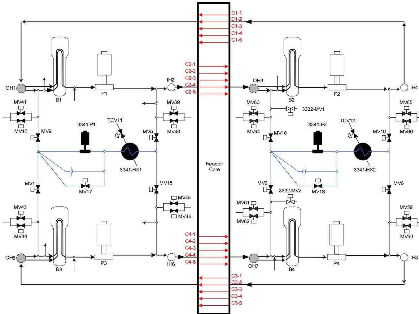
Figure 2: Representation of the PHTS and SDCS Circuits (case #1)
