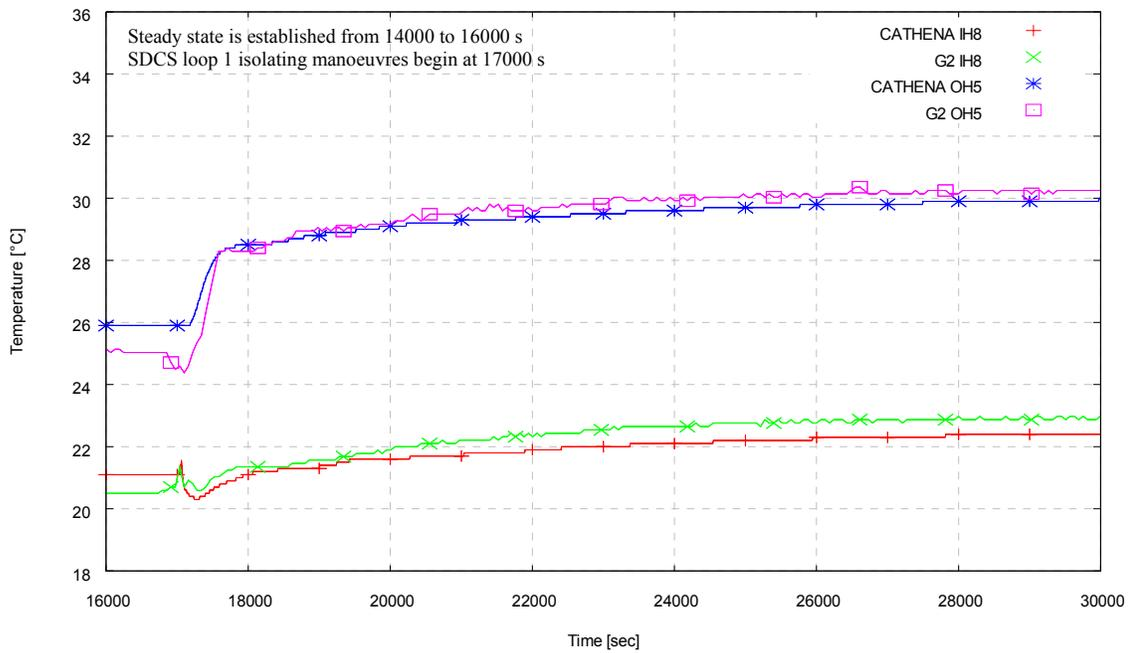
**Figure 20 : Transient Temperature at Inlet Header 8 (IH8) and Outlet Header 5 (OH5)
