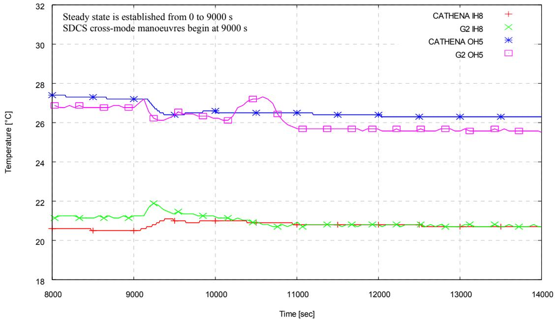
**Figure 13 : Transient Temperature at Inlet Header 8 (IH8) and Outlet Header 5 (OH5)
