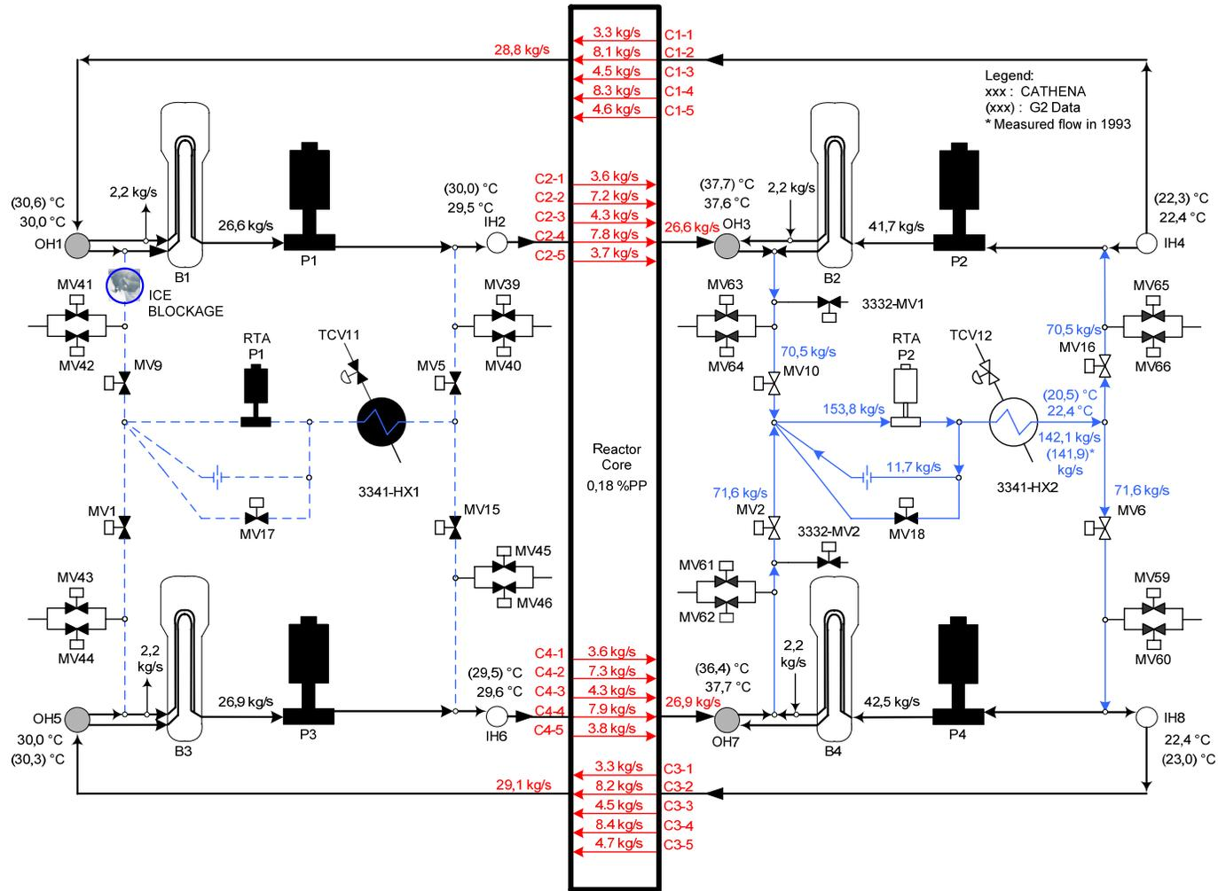
Figure 22: Steady Plant Conditions after 30000 sec (case #3)
