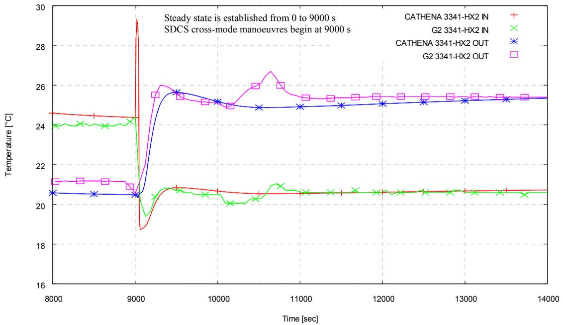
**Figure 15 : Transient Temperature at SDCS Heat Exchanger 3341-HX2 (case #2 : 0.22%PP)**
