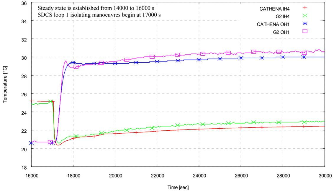
**Figure 17 : Transient Temperature at Inlet Header 4 (IH4) and Outlet Header 1 (OH1)
