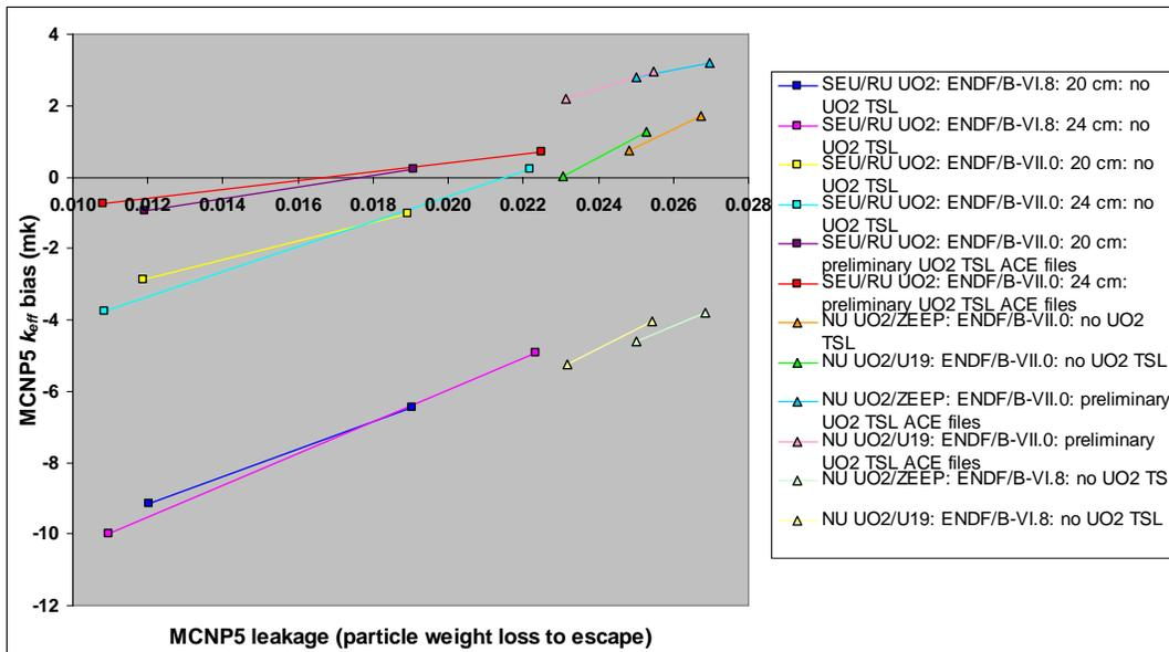
Figure 2: MCNP5  $k_{eff}$  simulation bias for ZED-2 critical experiments.
