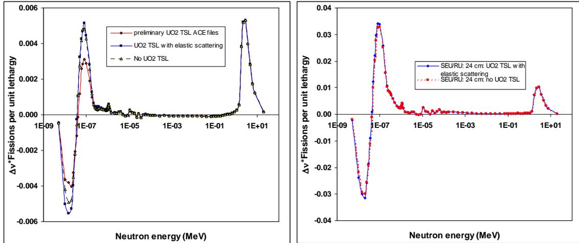
Figure 4: Energy dependence of MCNP CVR simulation bias based on differences in fission-yield tallies for air/D<sub>2</sub>O-cooled NU UO<sub>2</sub>/ZEEP and air/H<sub>2</sub>O-cooled SEU/RU 24-cm-pitch simulations.
