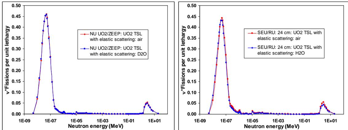
Figure 3: Energy dependence of MCNP track-length  $k_{eff}$  based on fission-yield tallies for air/D<sub>2</sub>O-cooled NU UO<sub>2</sub>/ZEEP and air/H<sub>2</sub>O-cooled SEU/RU 24-cm-pitch simulations.
