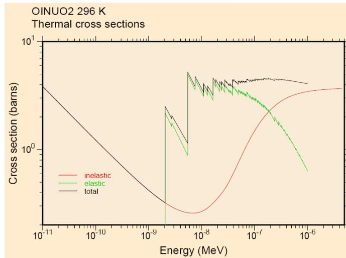
Figure 1: O-in-UO<sub>2</sub> TSL cross-section data components.
