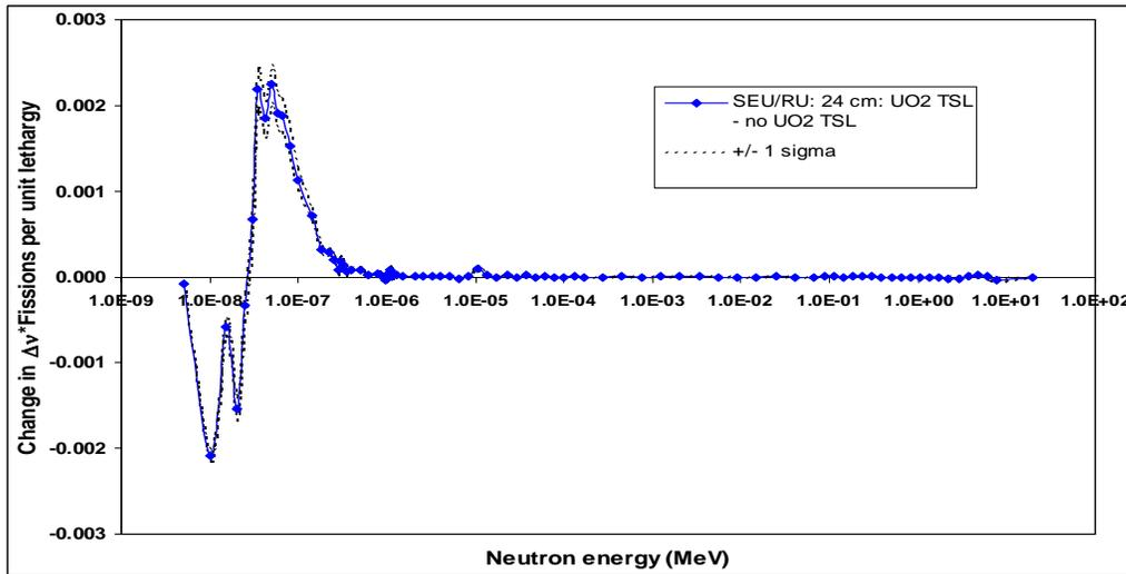
Figure 5: Energy dependence of the difference between MCNPX CVR biases for 24-cm-pitch SEU/RU simulations with and without UO<sub>2</sub> TSL data.
