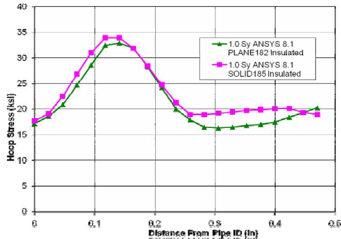
**Figure 9: Hoop Residual Stress Comparison for 2D And 3D models**
