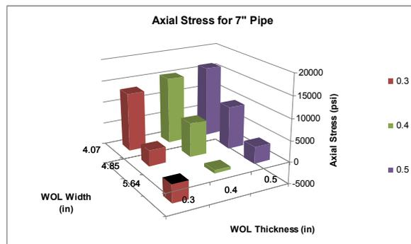
Figure 13: Axial Stress Distribution for the 7" Pipe
