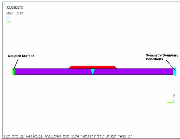
**Figure 4: Applied Boundary Conditions**
