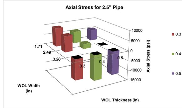
Figure 10: Axial Stress Distribution for the 2.5" Pipe
