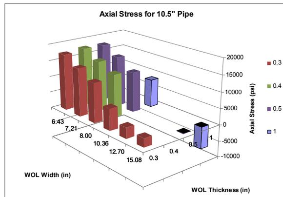
**Figure 15: Axial Stress Distribution for the 10.5" Pipe**
