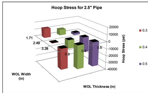
Figure 11: Hoop Stress Distribution for the 2.5" Pipe
