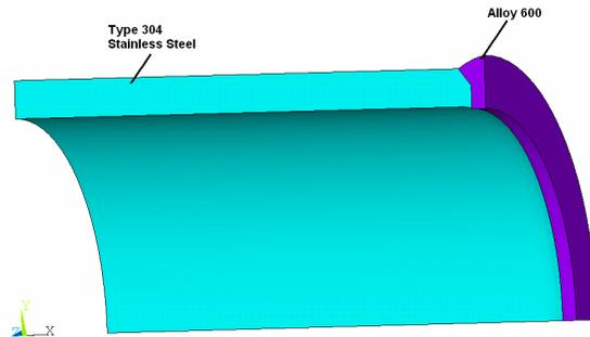
**Figure 2: Material Designation for the 3D Model
