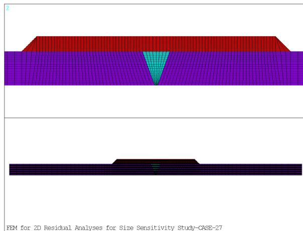
**Figure 6: Mesh Pattern of the Axisymmetric Model**
