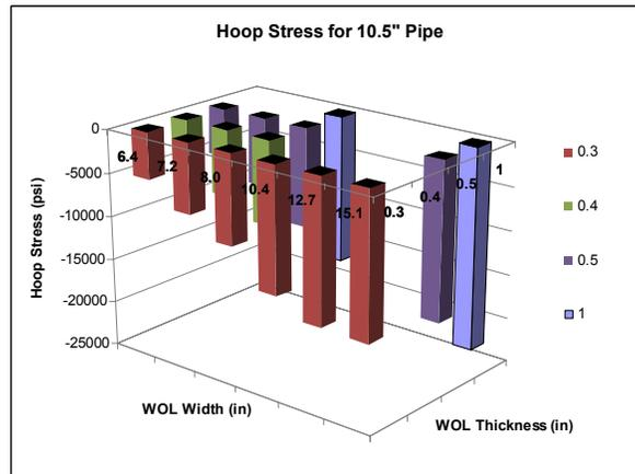
**Figure 16: Hoop Stress Distribution for the 10.5" Pipe**
