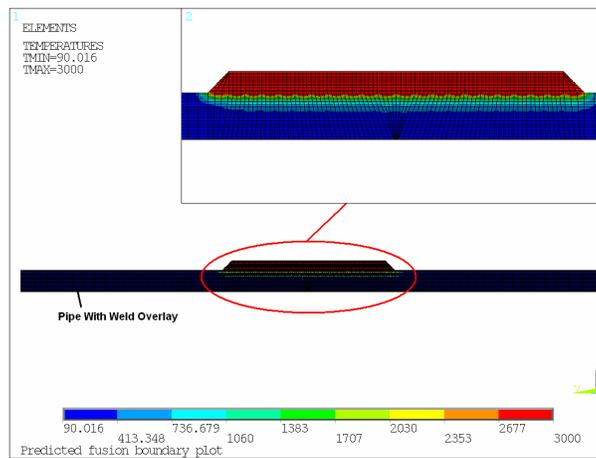
**Figure 7: Fusion Boundary Plot for the Weld Overlay**
