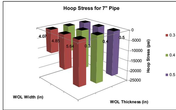
**Figure 14: Hoop Stress Distribution for the 7" Pipe**
