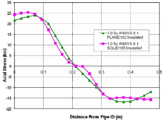
**Figure 8: Axial Residual Stress Comparison for 2D And 3D models**
