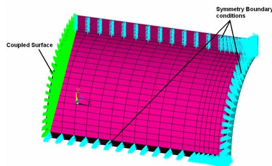
**Figure 1: Boundary Conditions for 3D Model**
