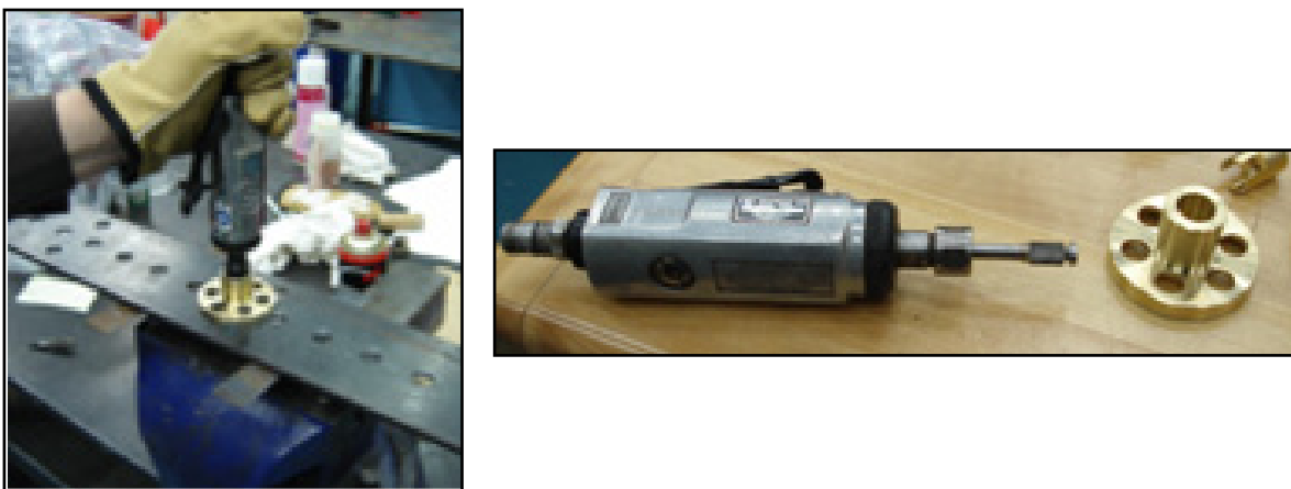
Figure 10 : Boring tool with the deburring plate
