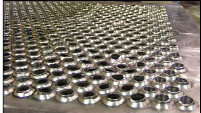
Figure 6 : Mock-up to test machining
