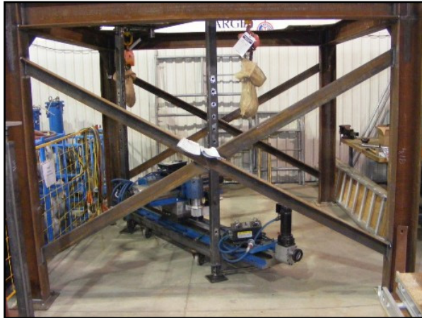
Figure 6 : Mock-up to test machining
