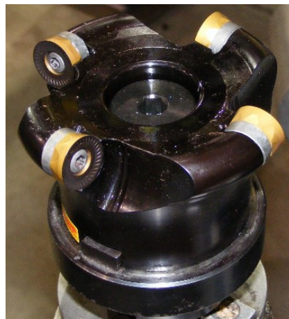
Figure 7 : Cutters used on the portable milling machine
