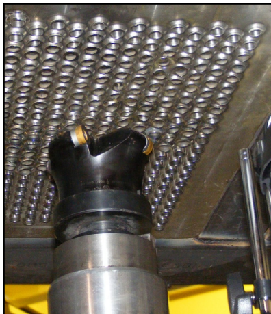
Figure 7 : Cutters used on the portable milling machine
