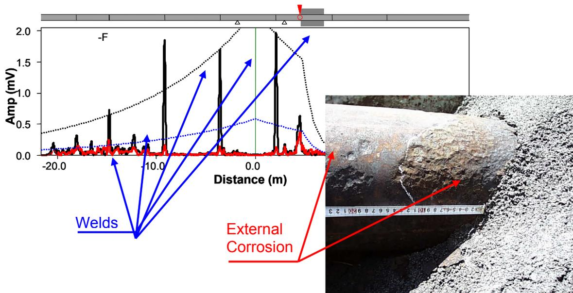
Figure 7: Typical G-Scan™ Data and Corresponding Pipe Features
