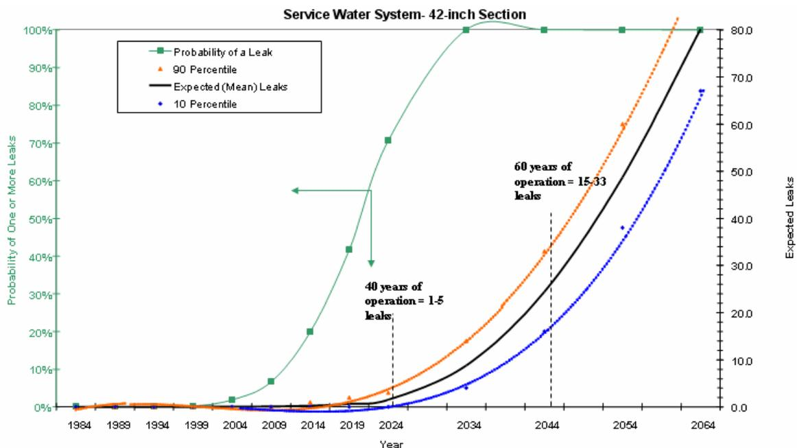
Figure 2. Predicted Leak Evolution. Example
