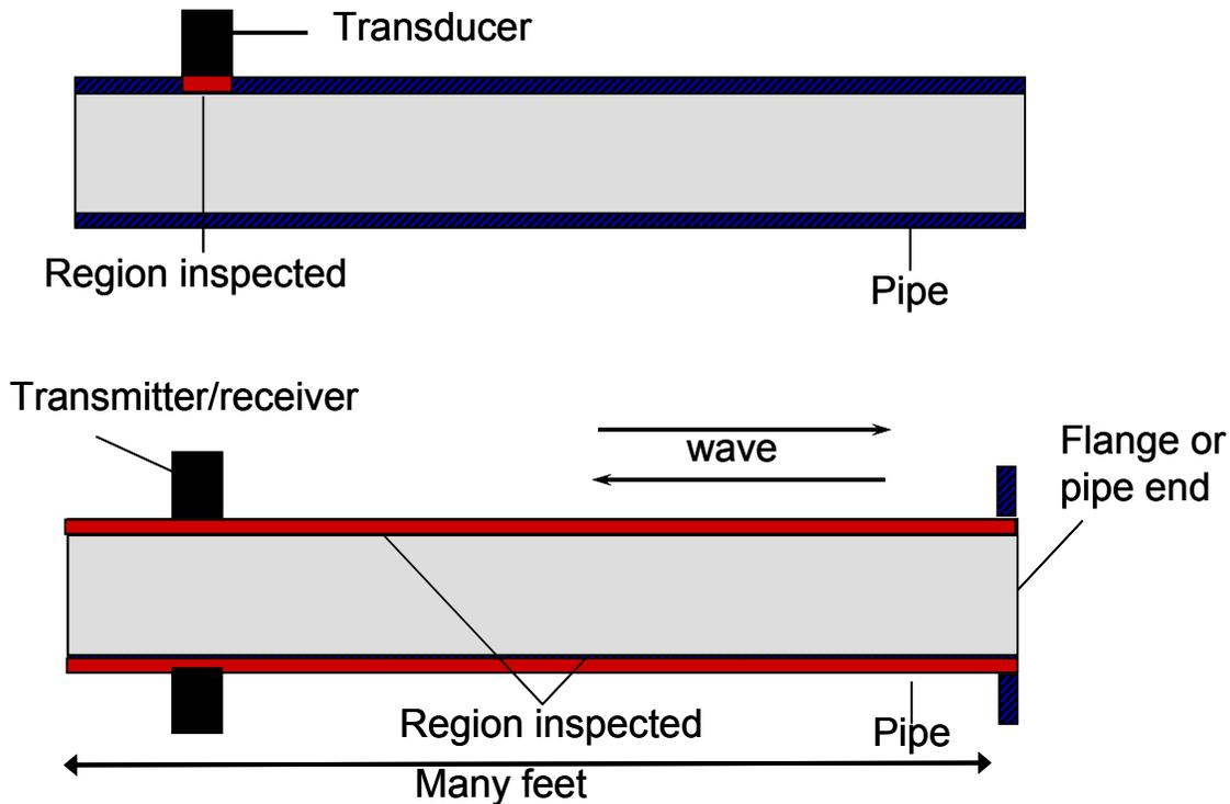
Figure 5. Typical UT (upper) vs. Long Range Guided Wave UT
