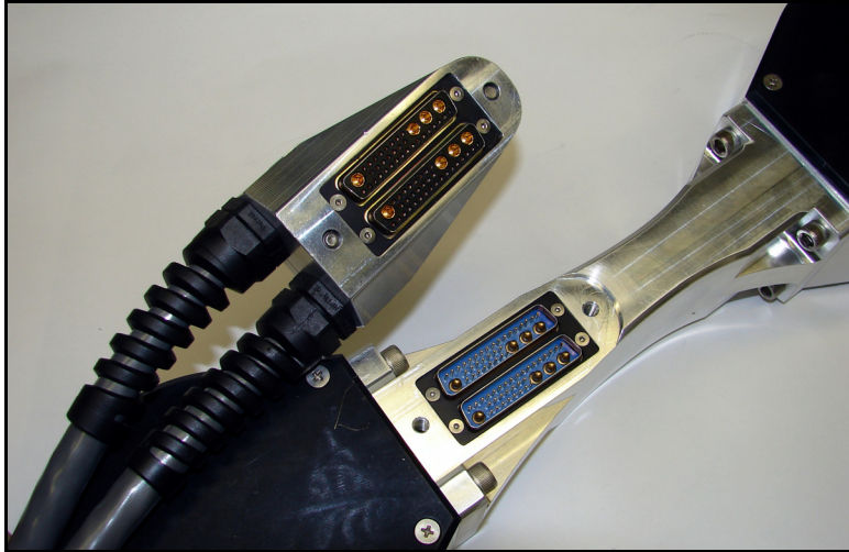
Figure 6: A prototype of the control cable interface.
