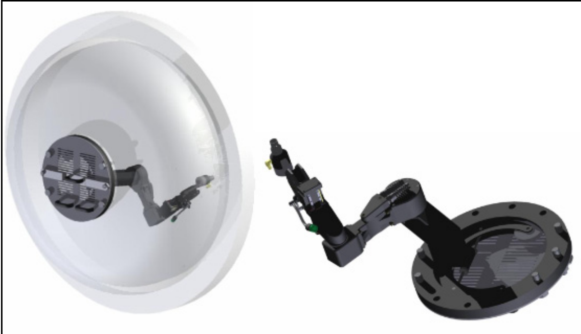
Figure 11: A Manway mounted Spyder Manipulator with manual third axis
