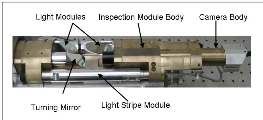
**Figure 4 Assembled inspection module.**
