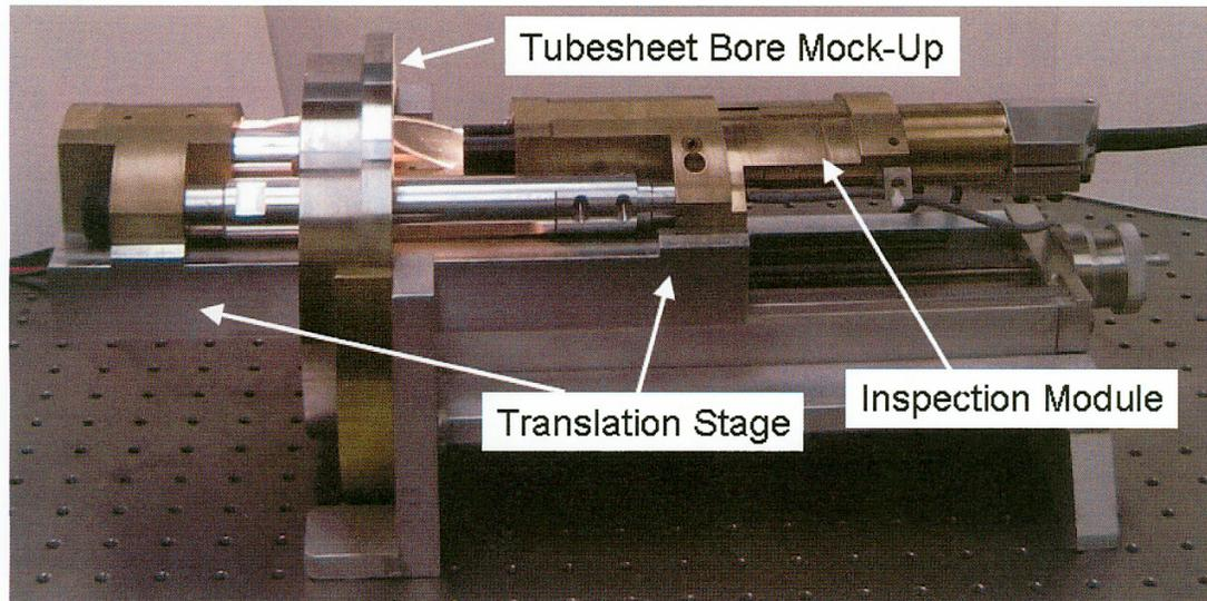
**Figure 5 Inspection module in alignment jig set up under the tubesheet bore mock-up.**
