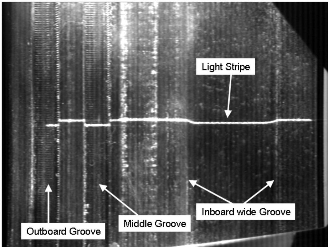
**Figure 6 Captured image of lattice rolled joint area with inspection module.**
