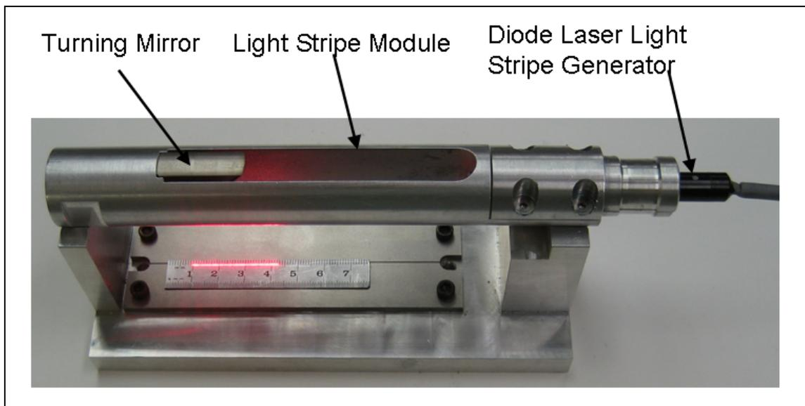
**Figure 3 Light stripe module mounted on its alignment jig.**
