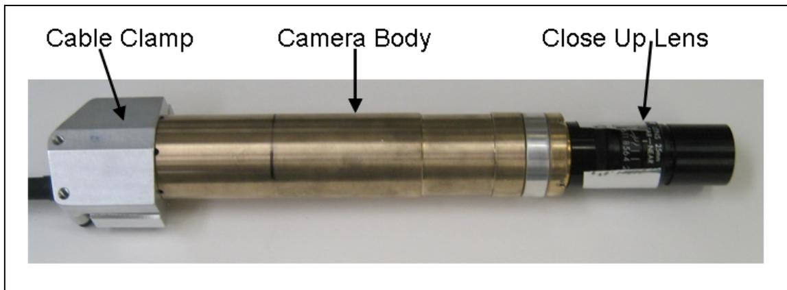
**Figure 1 Camera body with offset-angled cable clamp and close-up lens.**
