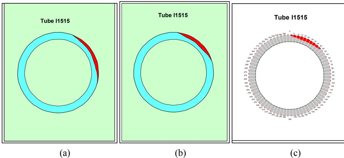
**Figure 5 Graphic representations of crack profile a) Original X-probe, b) HiRes X-probe, c) Destructive examination.**
