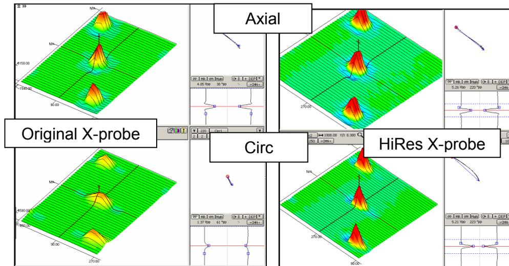
**Figure 3 Axial and circ. channel responses of the original X-probe and the HiRes probe to 1-mm diameter through wall holes.**
