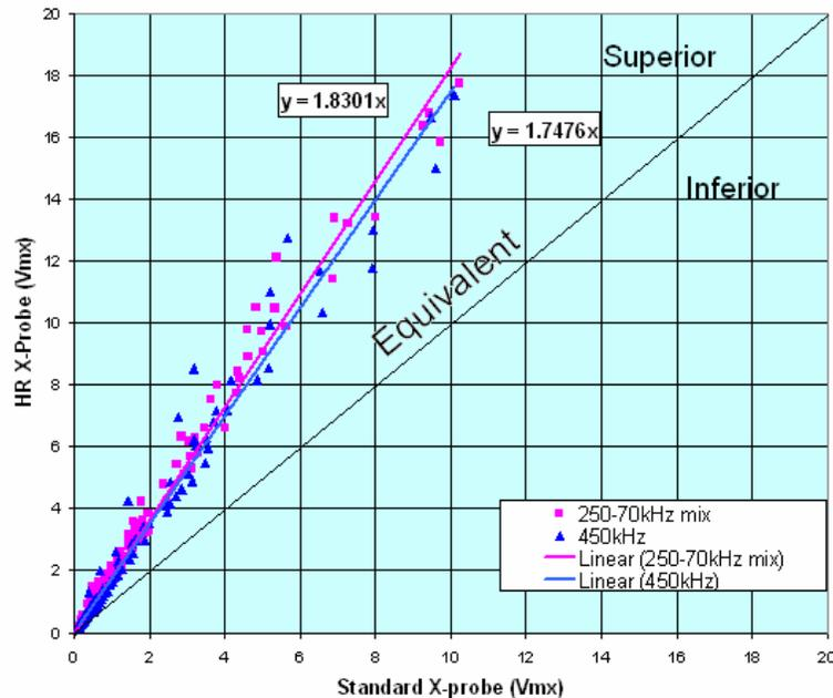
**Figure 7 Plot of the responses for all tested flaws obtained with the HiRes X-probe versus the responses from the original X-probe.**
