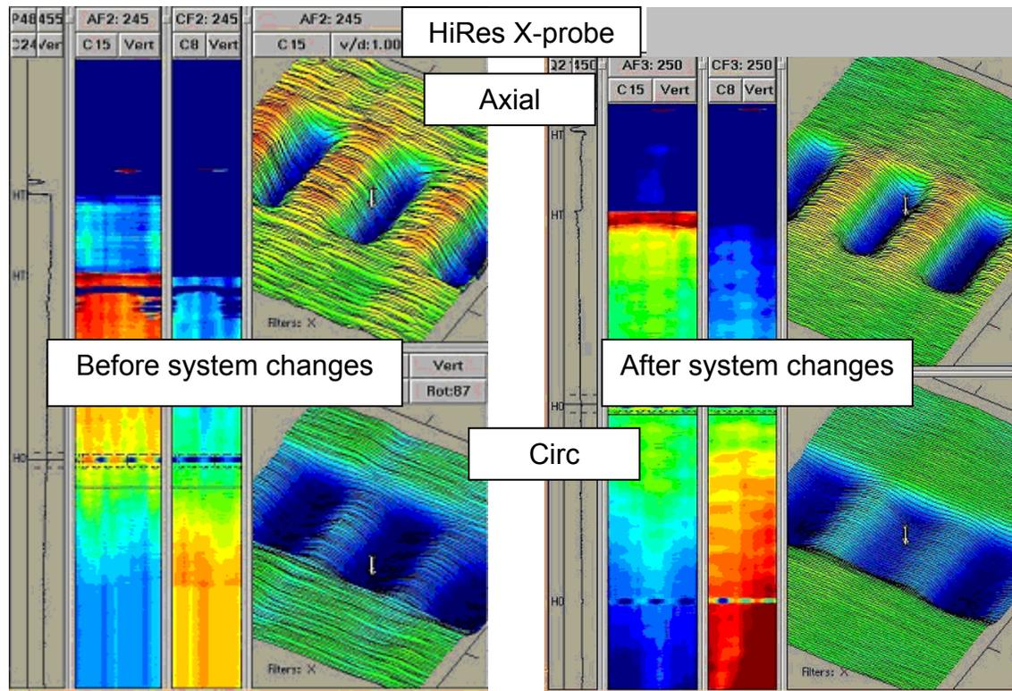
**Figure 6 High-resolution X-probe field data showing reduced noise levels before and after system changes.**
