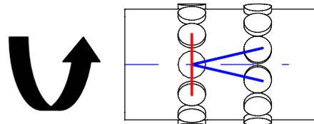
**Figure 2 HiRes X-probe with 2 rows of 12 coils.**
