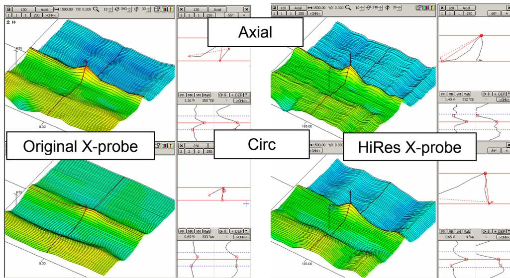
**Figure 4 Comparison of the original X-probe and the HiRes X-probe response to a short volumetric indication at the TTS.**
