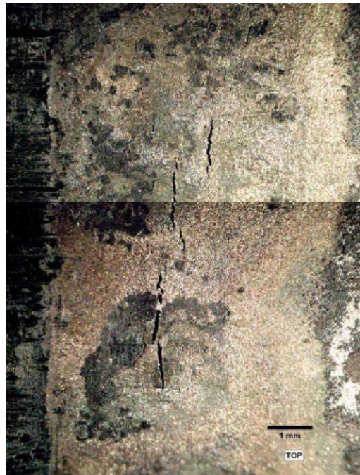
Figure 3 - Multiple Crack-like Features in BO1 R37C59
