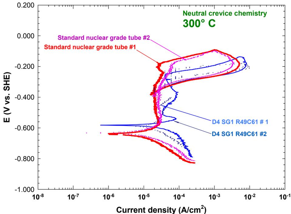
**Figure 4 Comparisons between the Potentiodynamic Polarization Curves of the Reference Alloy 800 Tubing and the Darlington Tubing D4 SG1 R49C61 Obtained at 300°C in Neutral Crevice Chemistry**
