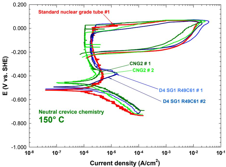
**Figure 12 Comparisons between the Potentiodynamic Polarization Curves of the Reference Alloy 800 Tubing, the Darlingtong Tubing D4 SG1 R49C61 and the Archived G2 NGS Tubing obtained at 150°C in Neutral Crevice Chemistry**
