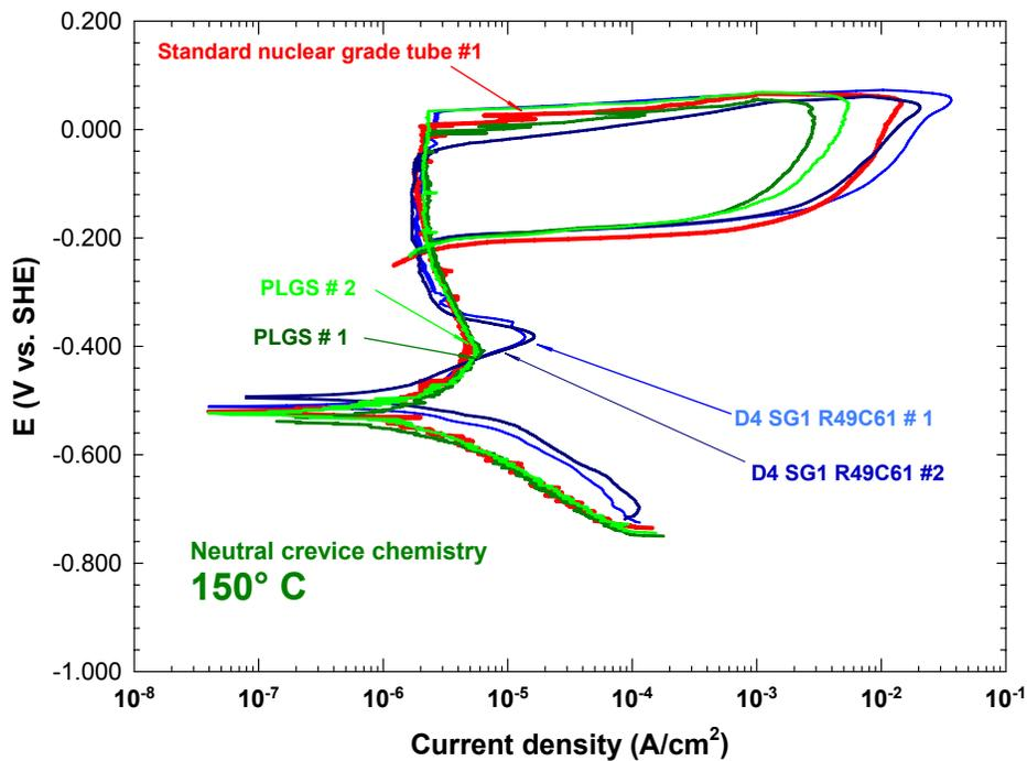
**Figure 13 Comparisons between the Potentiodynamic Polarization Curves of the Reference Alloy 800 Tubing, the Darlington Tubing D4 SG1 R49C61 and the Archived PLGS Tubing obtained at 150°C in Neutral Crevice Chemistry**
