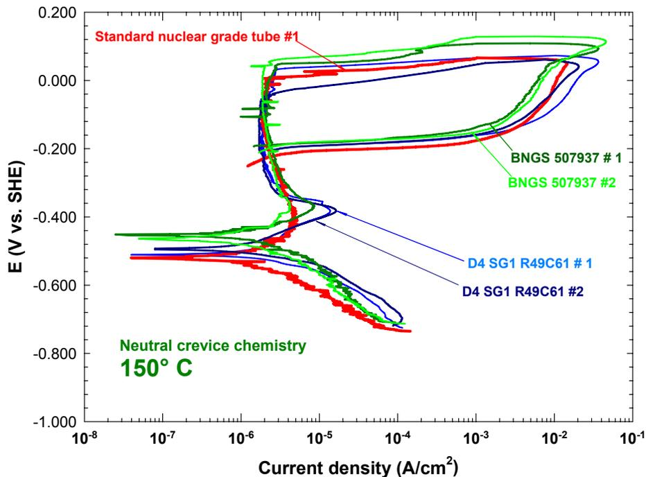
**Figure 14 Superimposed Potentiodynamic Polarization Curves of the Reference Alloy 800 Tubing, the Darlington Tubing D4 SG1 R49C61 and the Archived BNGS Tubing (HT# 507937) obtained at 150°C in Neutral Crevice Chemistry**
