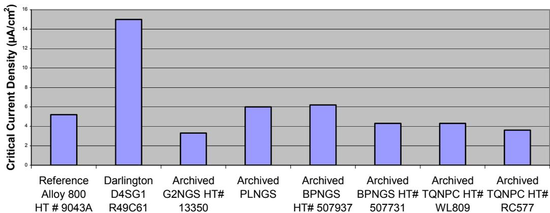
**Figure 18 The Amplitude of the Active Peak of the Polarization Curves of different Alloy 800 SG Tubing obtained at 150°C in Neutral Crevice Solution**
