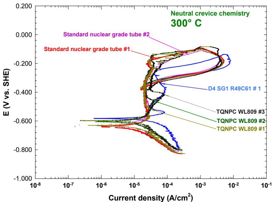
**Figure 9 Comparisons between the Potentiodynamic Polarization Curves of the Reference Alloy 800 Tubing, the Darlington Tubing D4 SG1 R49C61 and the Archived TQNPC Tubing (HT# WL 809) obtained At 300°C in Neutral Crevice Chemistry**
