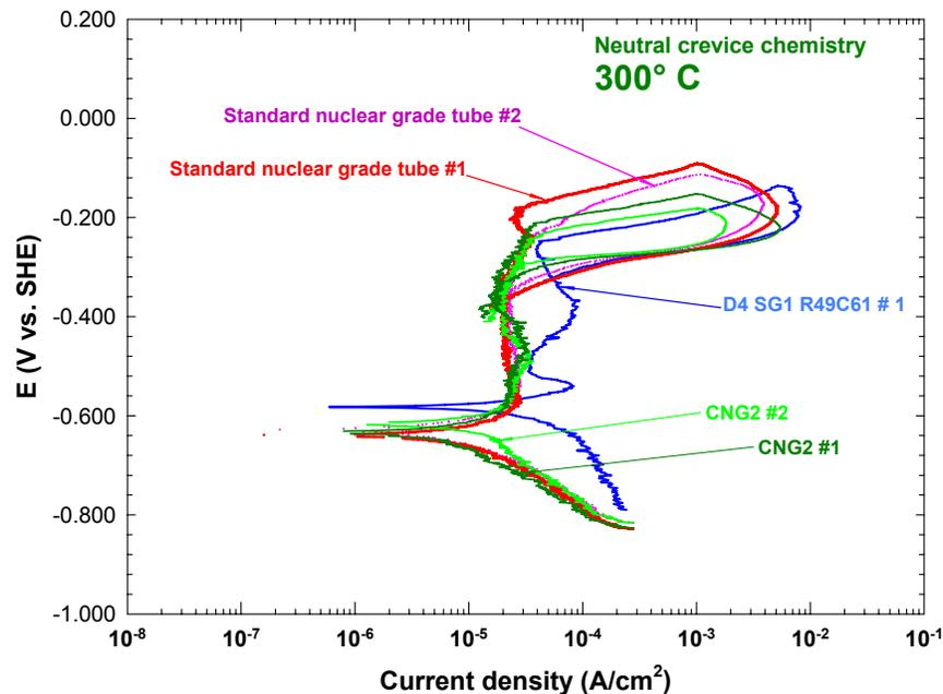
**Figure 5 Comparisons between the Potentiodynamic Polarization Curves of the Reference Alloy 800 Tubing, the Darlington Tubing D4 SG1 R49C61 and the Archived G2 NGS Tubing Obtained at 300°C in Neutral Crevice Chemistry**
