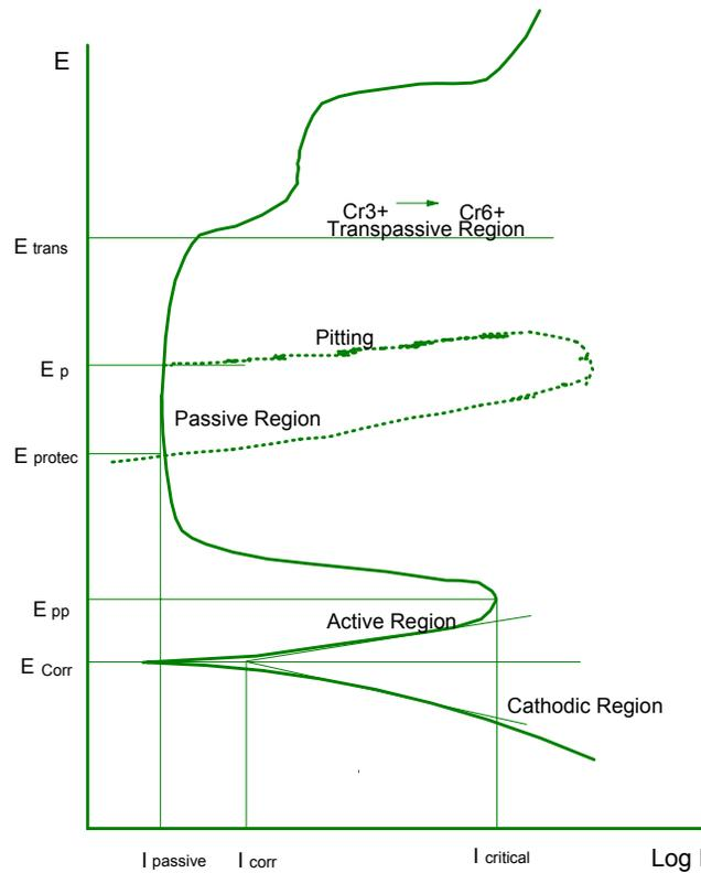
**Figure 1 Schematic Plots of Typical Polarization Curves for Chromium Containing Alloys**
