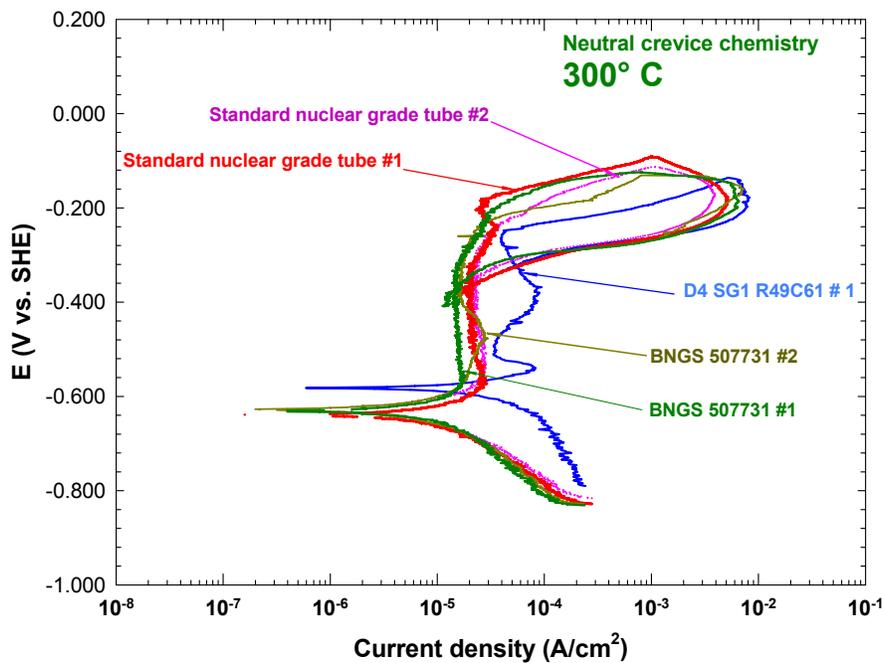
**Figure 8 Comparisons between the Potentiodynamic Polarization Curves of the Reference Alloy 800 Tubing, the Darlington Tubing D4 SG1 R49C61 and the Archived BNGS Tubing (HT# 507731) obtained at 300°C in Neutral Crevice Chemistry**
