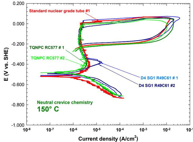
**Figure 17 Comparisons between the Potentiodynamic Polarization Curves of the Reference Alloy 800 Tubing, the Darlington Tubing D4 SG1 R49C61 and the Archived TQNPC Tubing (HT# RC577) obtained at 150°C in Neutral Crevice Chemistry**
