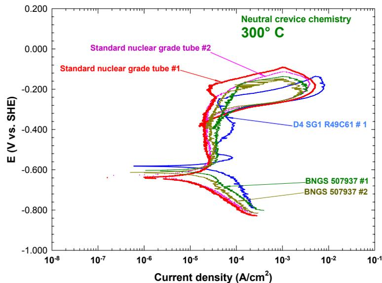
**Figure 7 Comparisons between the Potentiodynamic Polarization Curves of the Reference Alloy 800 Tubing, the Darlington Tubing D4 SG1 R49C61 and the Archived BNGS Tubing (HT# 507937) obtained at 300°C in Neutral Crevice Chemistry**
