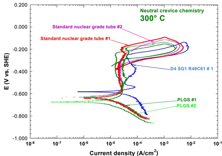
**Figure 6 Superimposed Potentiodynamic Polarization Curves of the Reference Alloy 800 Tubing, the Darlington Tubing D4 SG1 R49C61 and the Archived Alloy 800 Tubing from PLGS obtained at 300°C in Neutral Crevice Chemistry**
