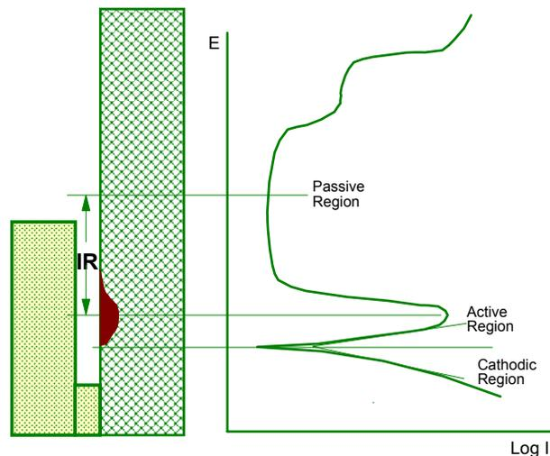
**Figure 19 Schematic Illustration of the IR Drop Mechanism of Crevice Corrosion**
