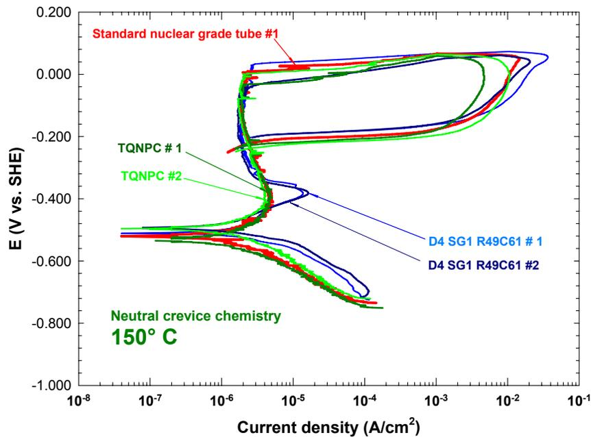
**Figure 15 Superimposed Potentiodynamic Polarization Curves of the Reference Alloy 800 Tubing, the Darlington Tubing D4 SG1 R49C61 and the Archived BNGS Tubing (HT# 507731) obtained at 150°C in Neutral Crevice Chemistry**
