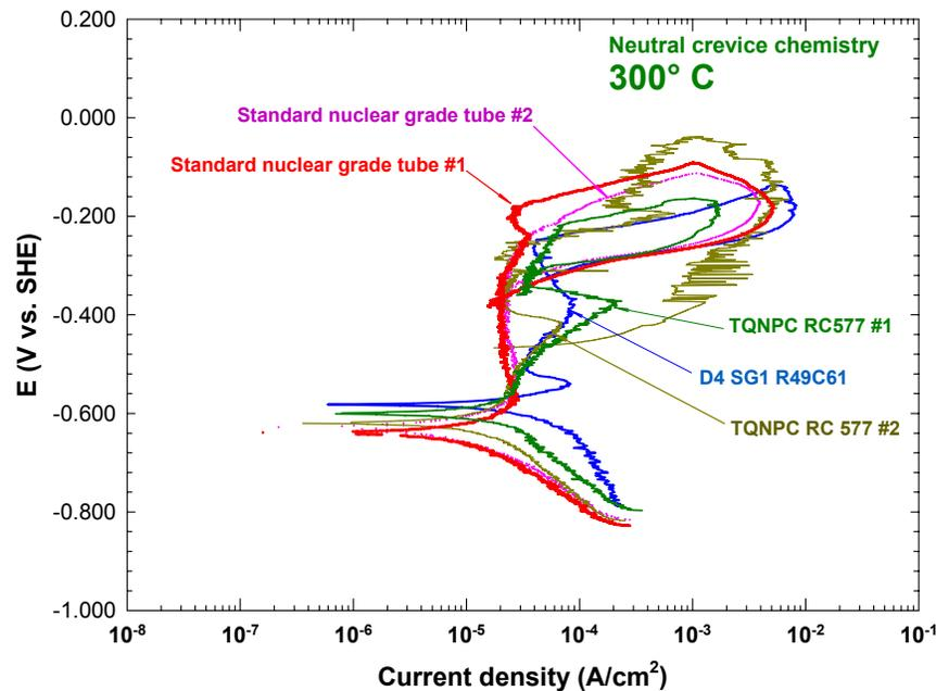
**Figure 10 Comparisons between the Potentiodynamic Polarization Curves of the Reference Alloy 800 Tubing, the Darlington Tubing D4 SG1 R49C61 and the Archived TQNPC Tubing (HT# RC577) obtained at 300°C in Neutral Crevice Chemistry**
