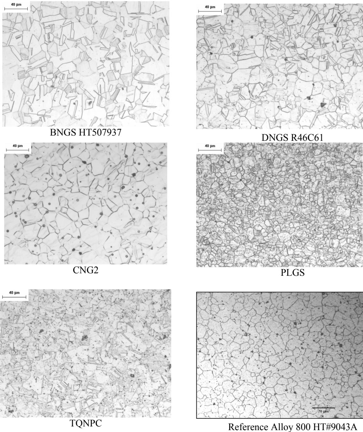
**Figure 3 Microstructure of the Materials taken from the Cross-Section of the Alloy 800 Tubes**
