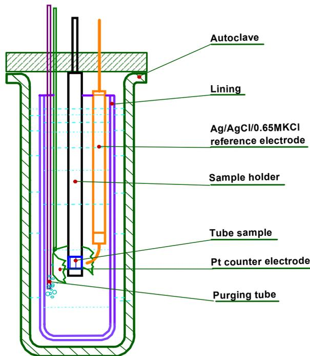
**Figure 2 A 3-Electrode System for Electrochemical Measurements in a Static Autoclave**
