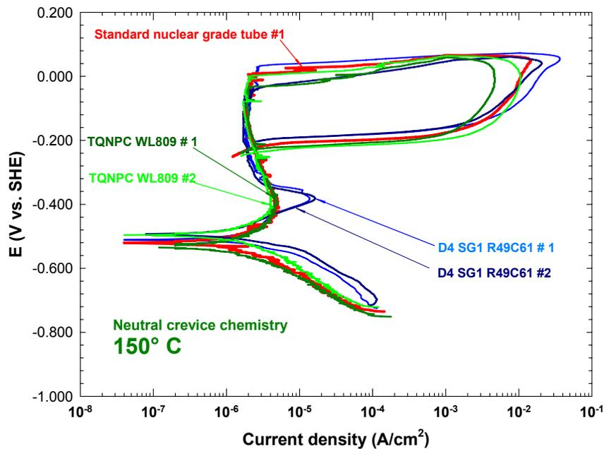
**Figure 16 Comparisons between the Potentiodynamic Polarization Curves of the Reference Alloy 800 Tubing, the Darlington Tubing D4 SG1 R49C61 and the Archived TQNPC Tubing (HT# WL809) obtained at 150°C in Neutral Crevice Chemistry**
