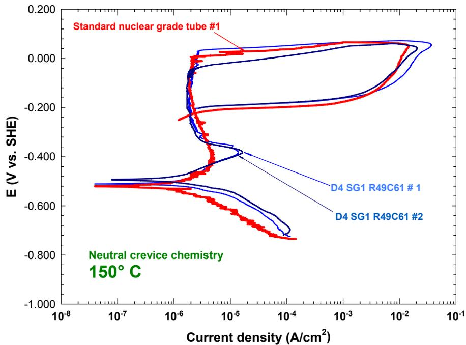
**Figure 11 Superimposed Potentiodynamic Polarization Curves of the Reference Alloy 800 Tubing, the Darlingtong Tubing D4 SG1 R49C61 obtained at 150°C in Neutral Crevice Chemistry**
