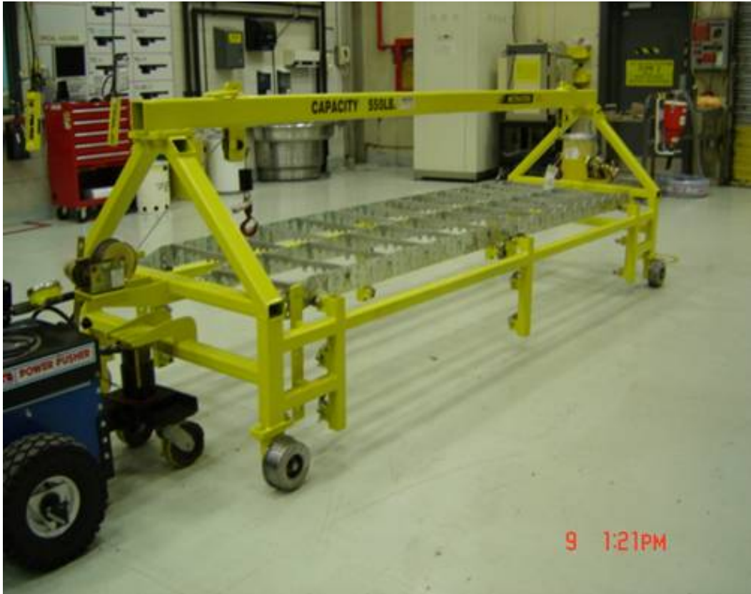
Staff Designed Powertrack Chain Replacement Tool
