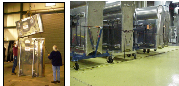
Figure 7. Application of Water Shield Wall for Dose Reduction
