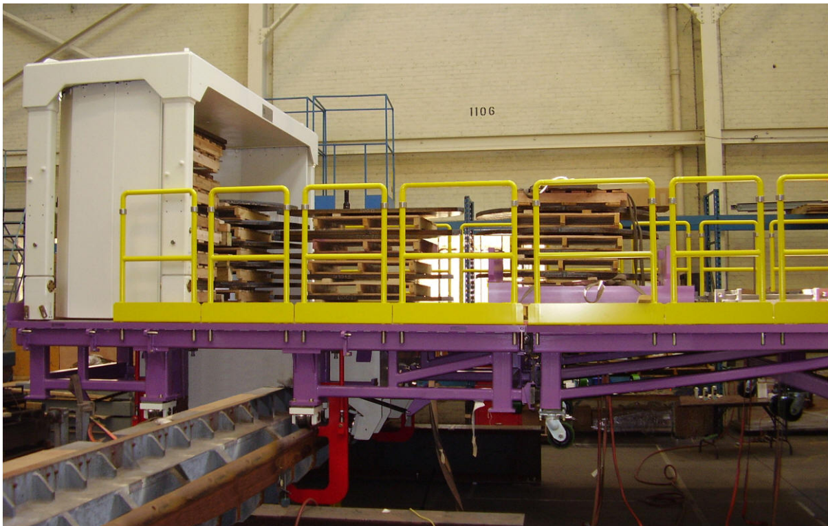
Figure 7 Configuration B, Illustration On The RAB Bridge Beam And Photographed On The Mock-Up Bridge Beam During Proof Load Testing At GEH
