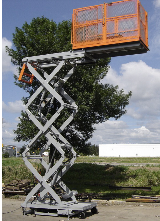
Figure 20 Worker Access Time Further Improved By A Cantilevering Scissor-Lift
