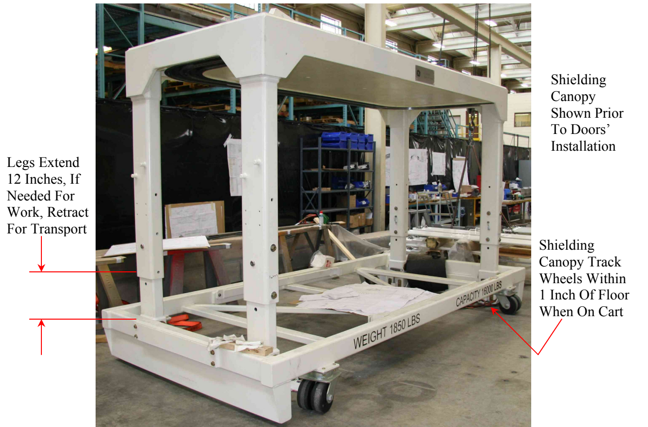
Figure 15 Shielding Canopy, Shown Legs Extended, On Low-Height Transportation Cart
