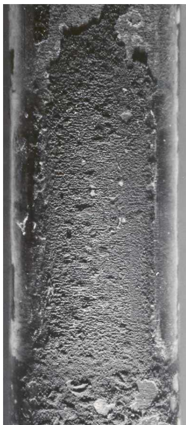
Light erosion corrosion feature at 1 st Support
