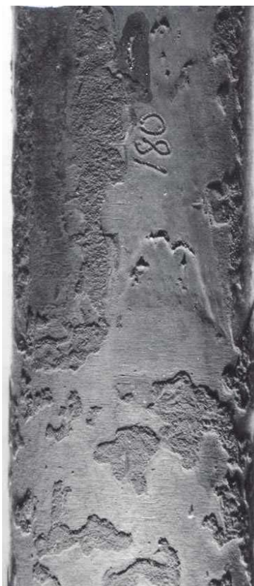
Moderate erosion corrosion feature at 3 rd Support
