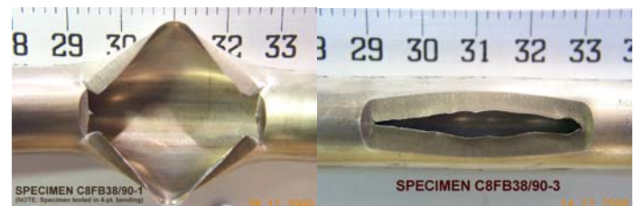
Figure 11: Effect of Break-Opening 4-point (left) versus 3-point (right)
