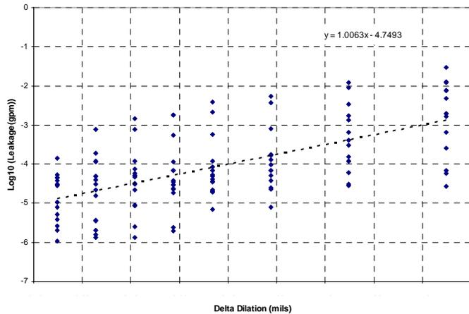
**FIGURE 5 DELTA DILATION VERSUS LEAKAGE**
