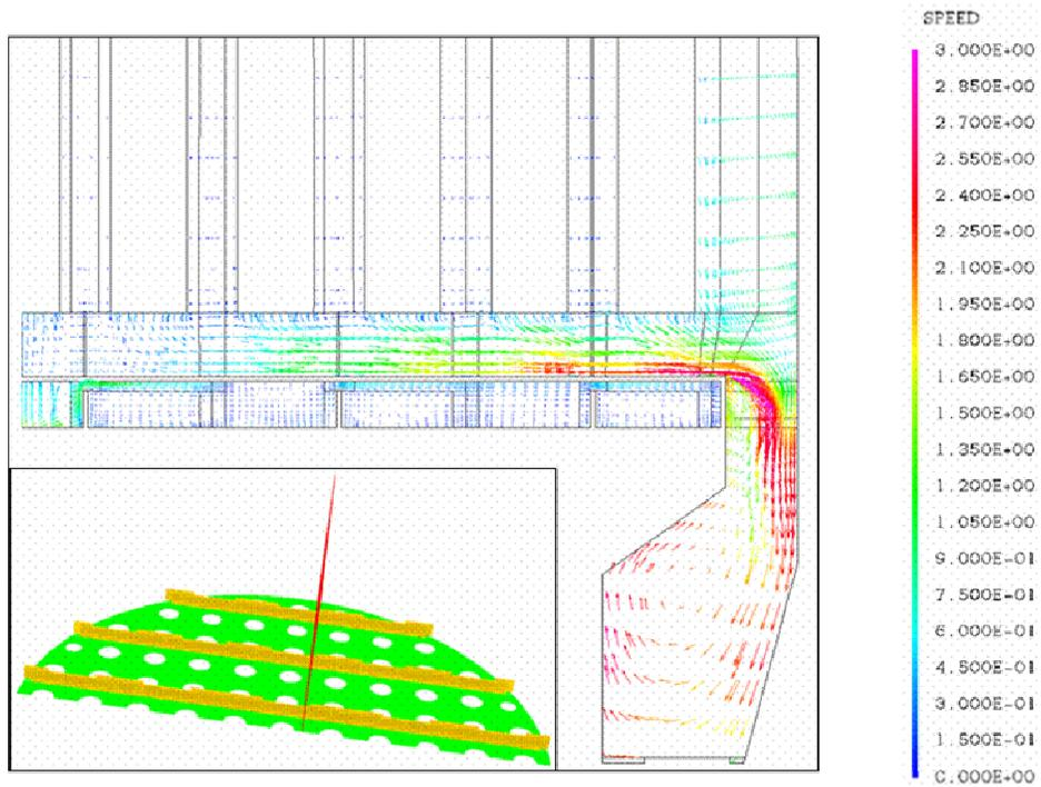
Figure 16 – Sludge Collector Velocity Profile
