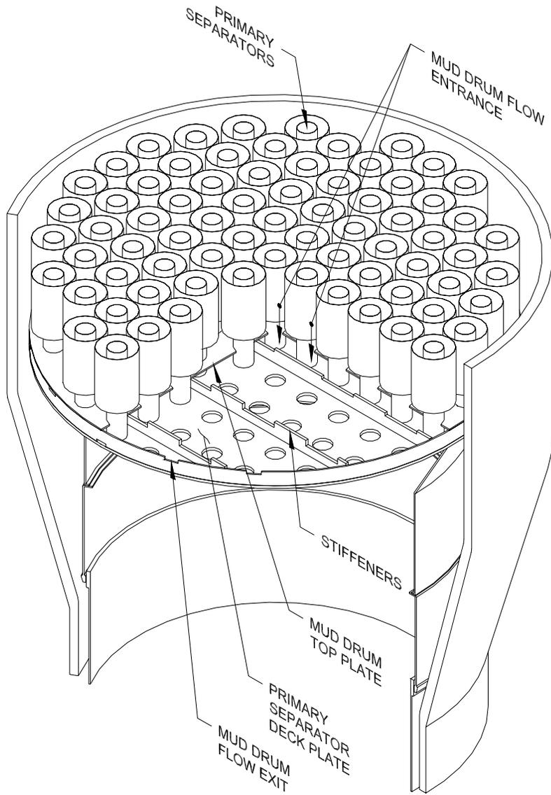
**Figure 12 – Sludge Collector Arrangement**
