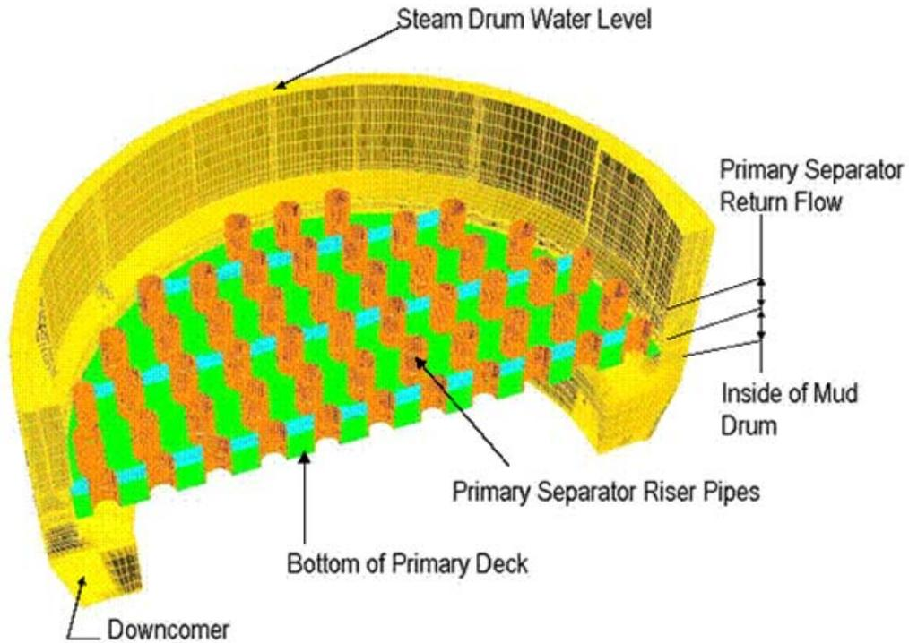
**Figure 13 – CFD Model Solution Domain**
