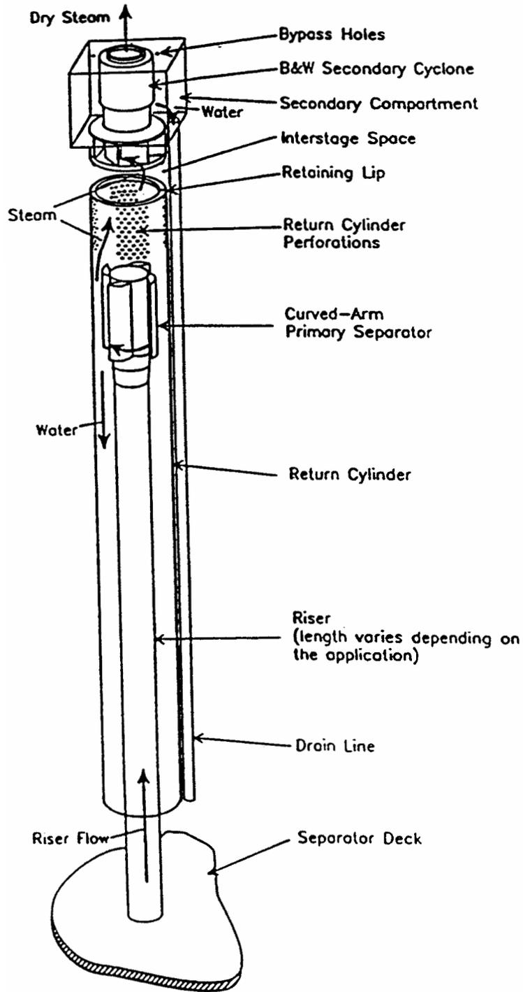
Figure 9 – Primary and Secondary Steam Separators
