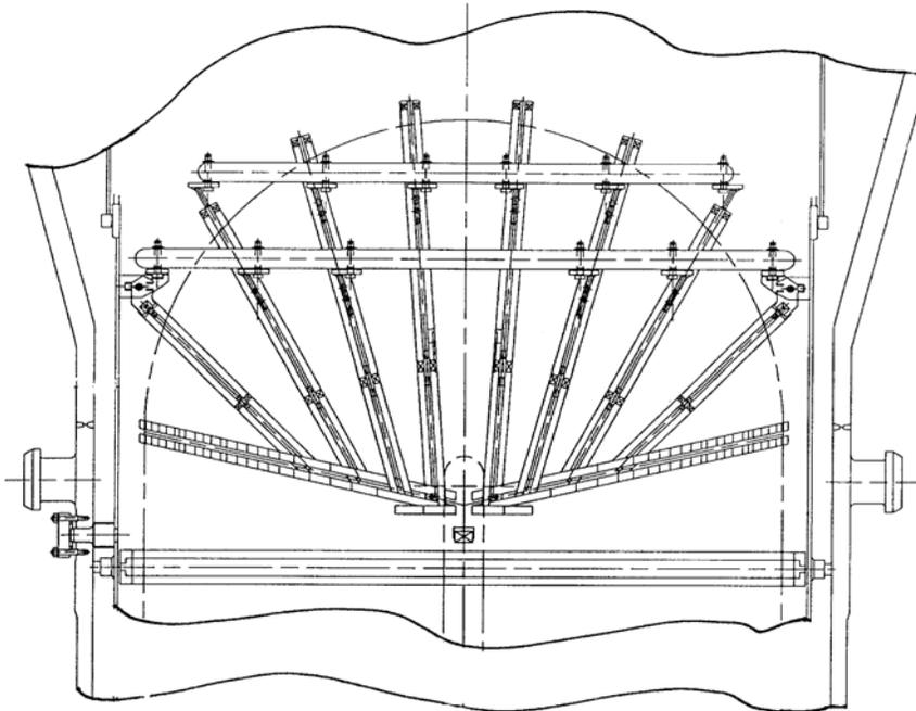
**Figure 7 – Flatbar U-Bend Restraint Configuration**
