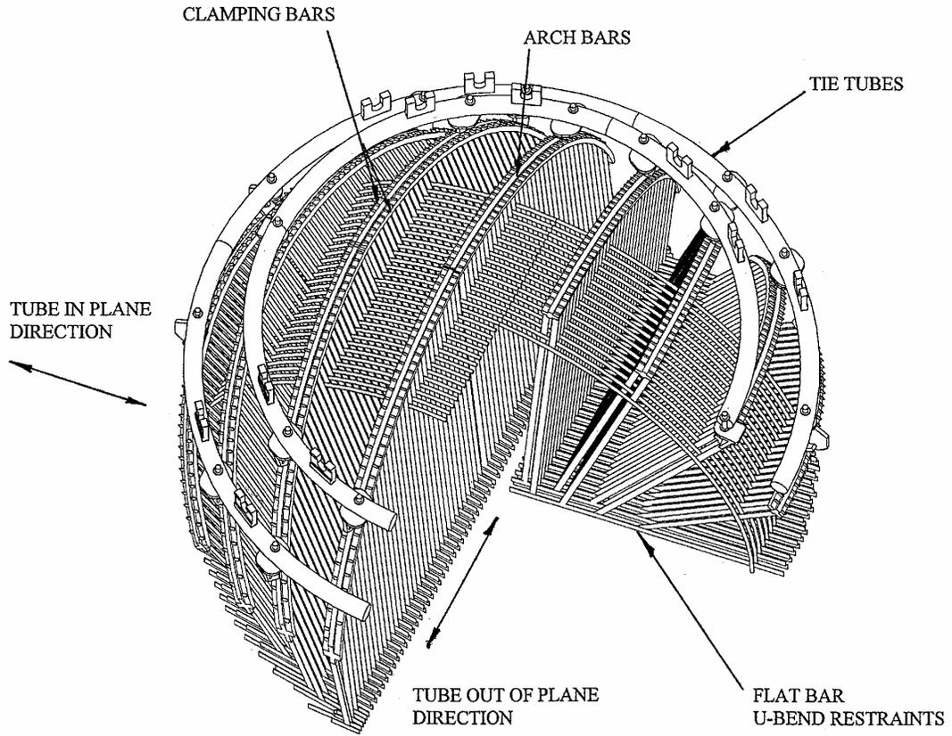
**Figure 8 – Flatbar U-Bend Restraint Arrangement**
