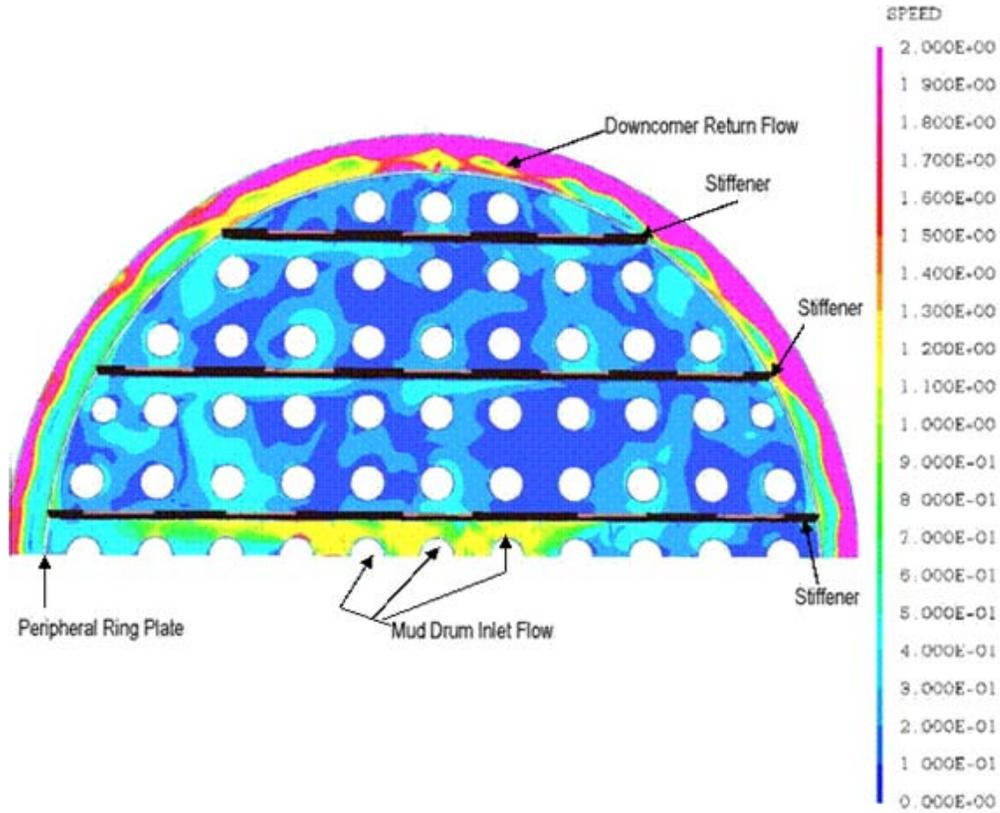
Figure 15 – Velocity Distribution within the Sludge Collector
