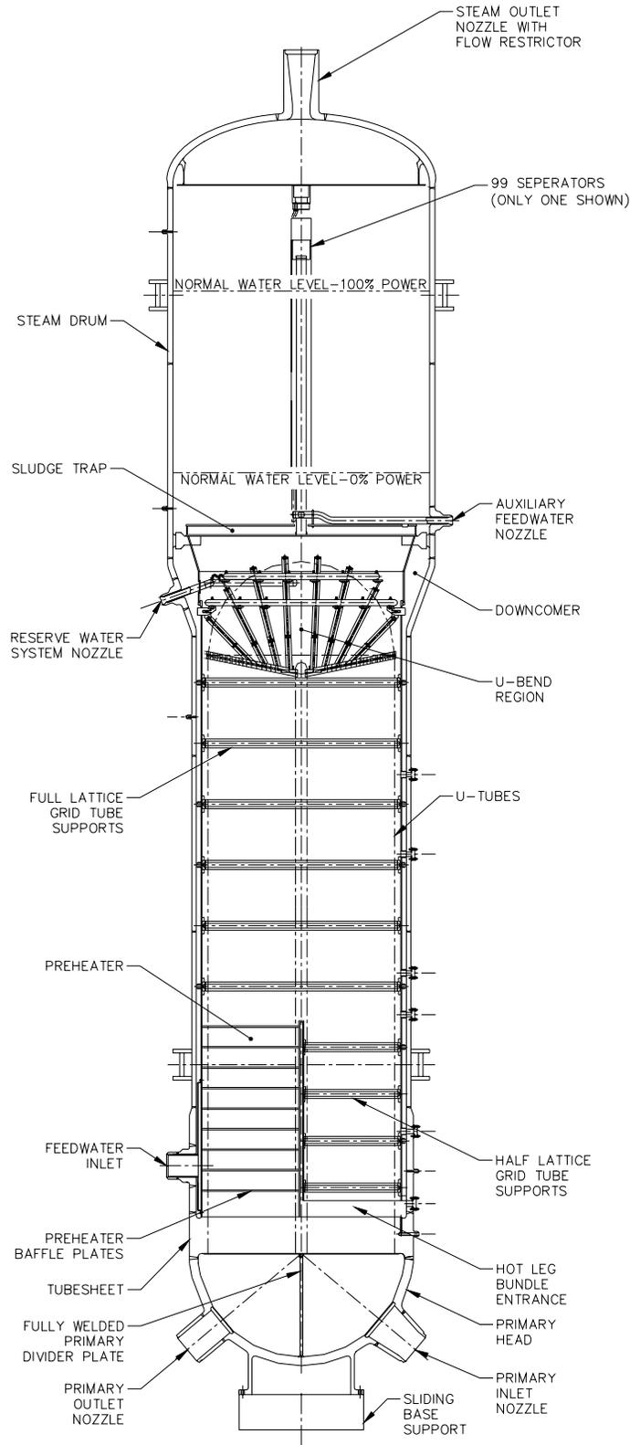
**Figure 1 – Overall Arrangement of the ACR-1000 Steam Generator**
