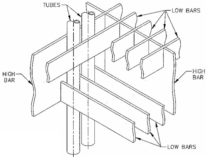
**Figure 6 –Lattice Bar Tube Support Arrangement**
