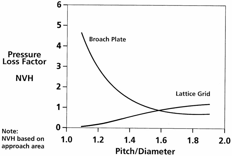
Figure 4 – Tube Support NVH versus Pitch / Diameter Ratio
