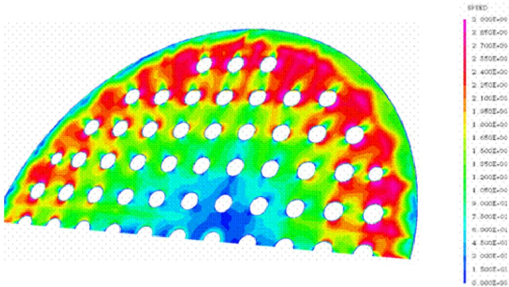
**Figure 14 – Velocity Profile Above Primary Separator Deck
