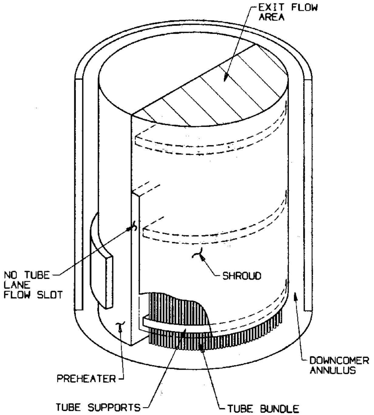
Figure 2 – Isometric View of Preheater
