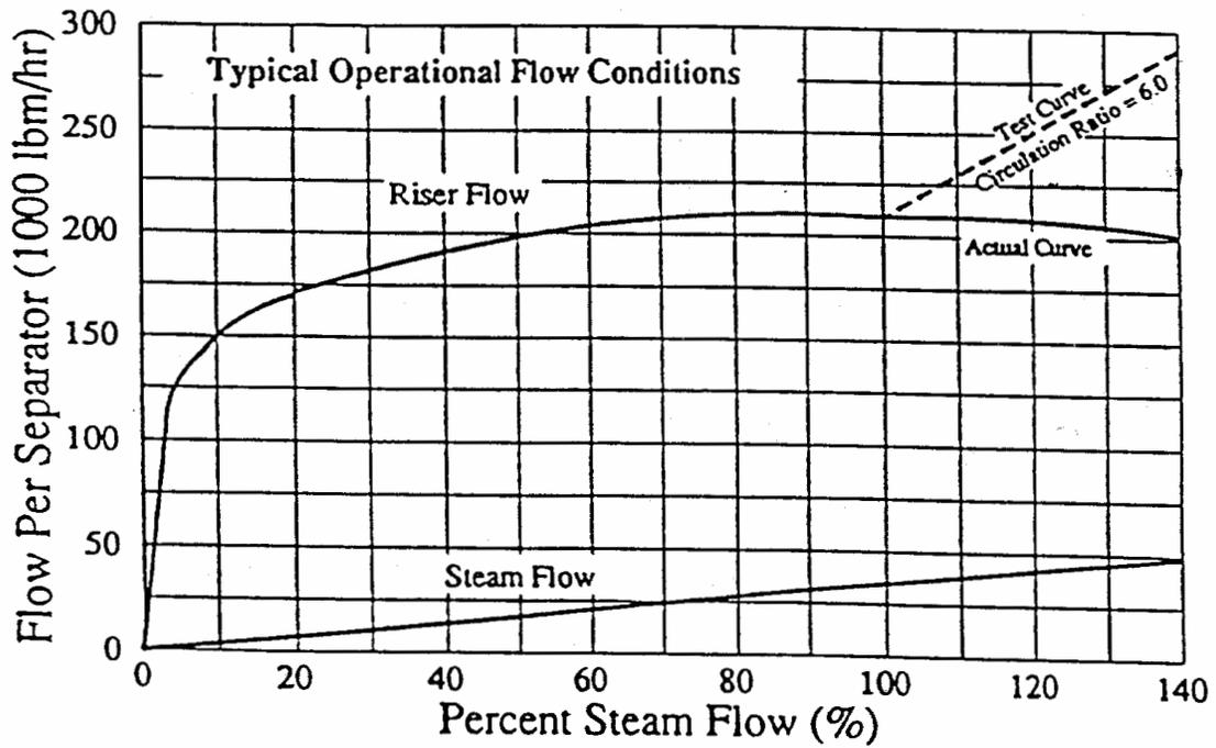
Figure 10 – Typical Operational Circulation Ratio and Flow Conditions
