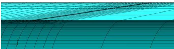
(b) crack-tip mesh parallel to the axial direction (biased outward, closer spacing on the OD side)
