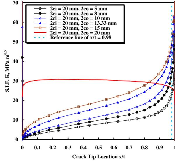
**Fig. 10** Variation of stress intensity factors along the crack front line of trapezoidal crack and rectangular crack ( $P_i = 6.90$  MPa)
