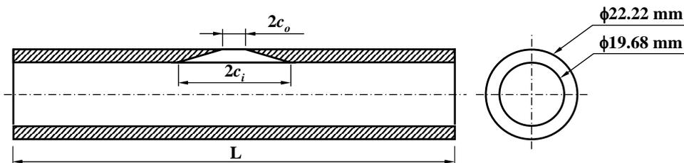
**Fig. 3** Geometry and size of tube specimen
