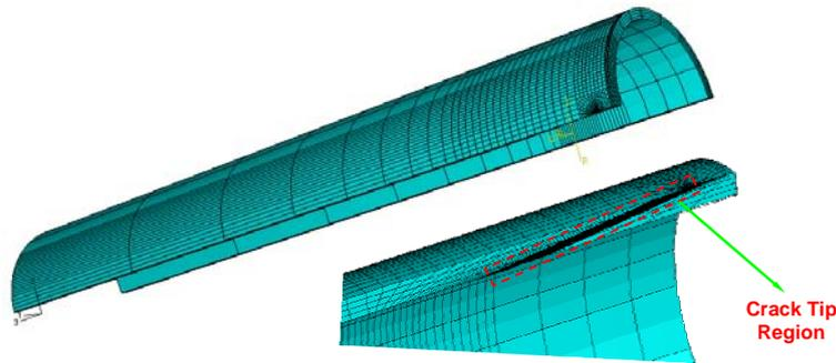
Fig. 6 Typical finite element mesh of SG tube containing axial through-wall trapezoidal crack
