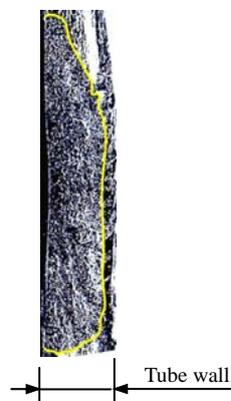
**Fig. 2** A typical fracture surface of the tube pulled out from expansion region[8]
