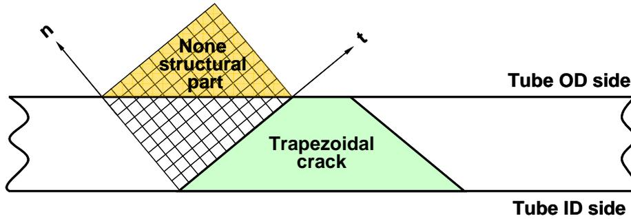
Fig. 5 Generation of crack-tip finite element mesh for trapezoidal crack analysis
