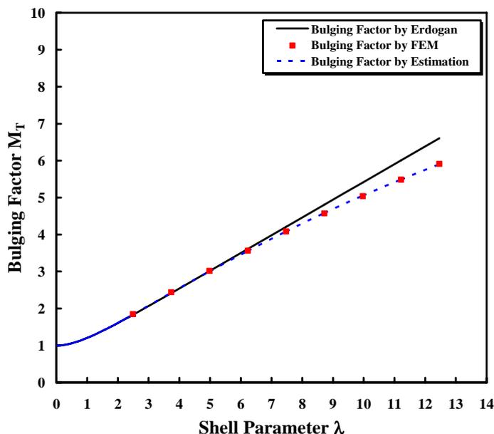
Fig. 7 Comparison of bulging factors between Erdogan's results and finite element results
