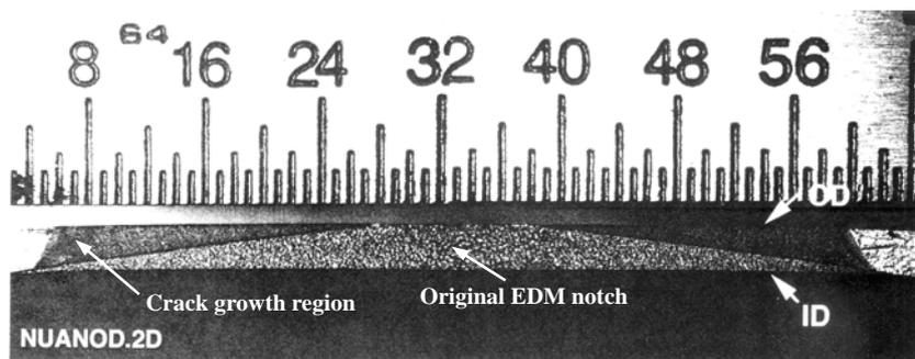
**Fig. 4** Fracture surface of the tube specimen with the original flaw length of  $2c_i = 25.4$  mm and  $2c_o = 4.78$  mm.
