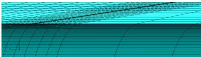
(a) crack-tip mesh parallel to the axial direction (non-biased, uniform spacing through thickness)
