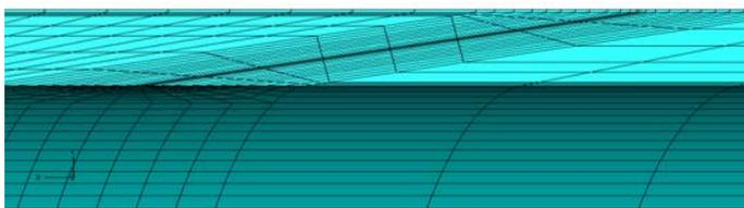
(c) crack-tip mesh normal to the crack front line over the inner part of the tube thickness
