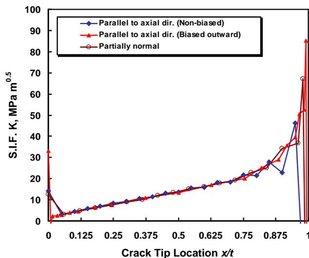
**Fig. 9** Variation of stress intensity factors along the crack front line of a trapezoidal crack with  $2c_i = 25.4$  mm and  $2c_o = 12.7$  mm ( $P_i = 7.1$  MPa)
