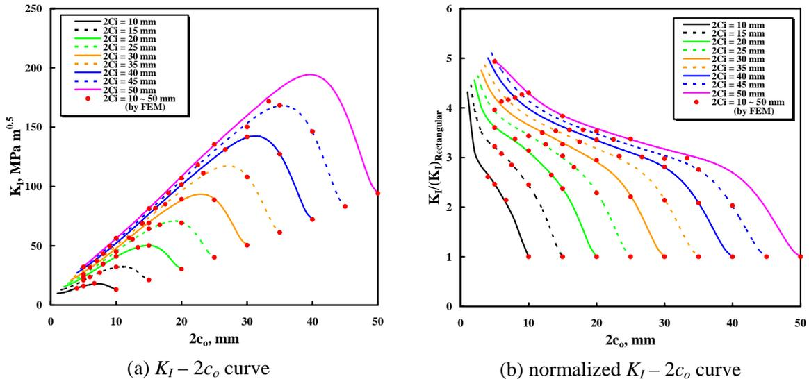
Fig. 11 Variation of stress intensity factor as the crack size and shape change
