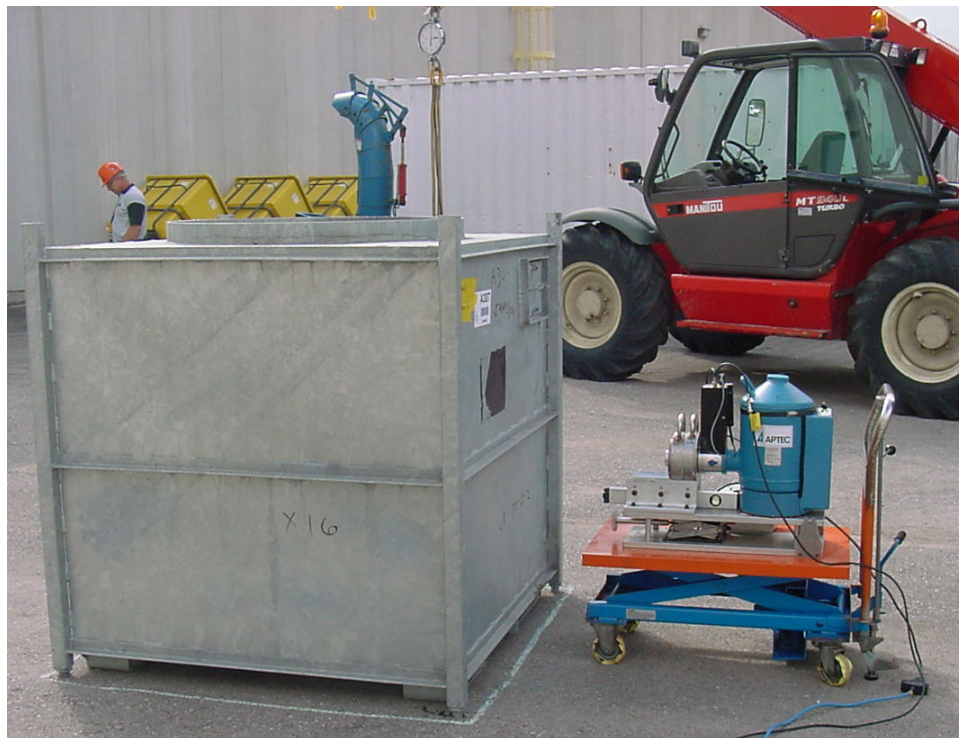
Figure 1 In-Situ Scanning of an Ash Box Using the Portable Germanium Detector
