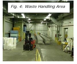
As long as the bags meet the criteria, they are loaded into stainless steel reusable storage containers (RSC's) which are subsequently loaded into an ISO container. As long as the criteria for the standing shipment permit are not exceeded, the shipment is then classified by the staff loading the ISO.
